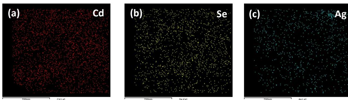
Figure S3. (a, b, c) EDS mapping of Cd, Se, and Ag respectively in Ag: CdSe NPLs.
