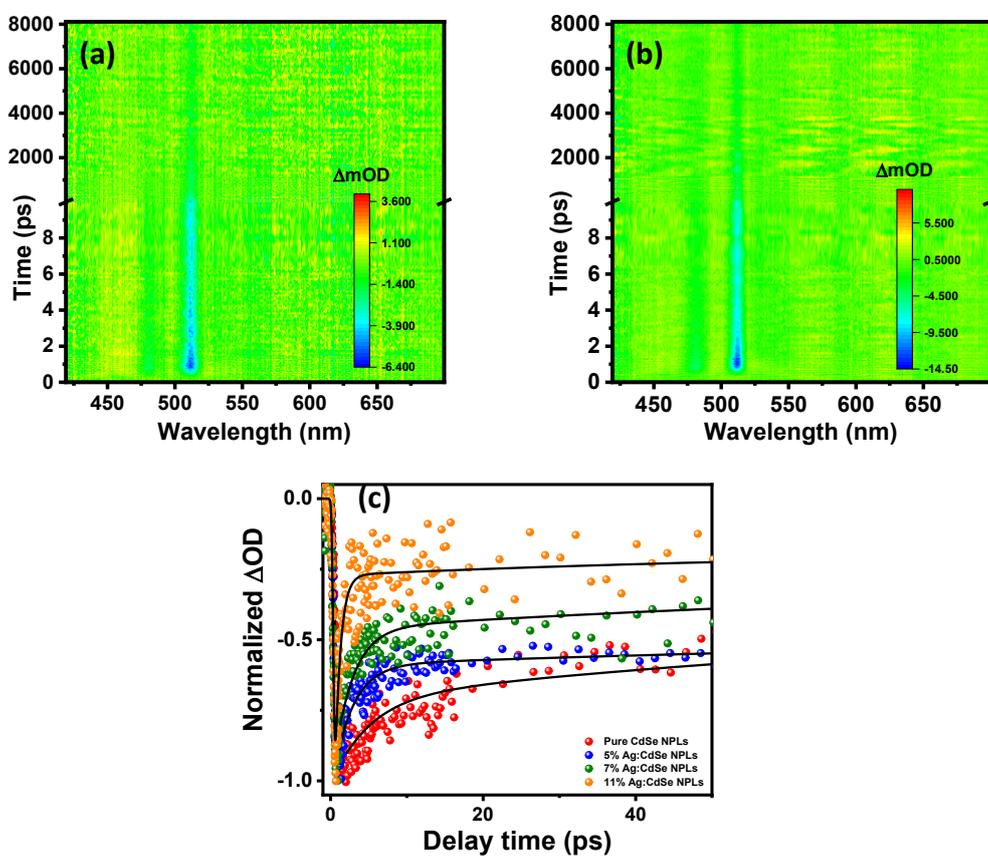
Figure S6. (a, b) 2D false color map of 4 ML 5% and 7% Ag doped CdSe NPLs, respectively. (c) Normalized bleach recovery kinetics of undoped and doped CdSe NPLs
