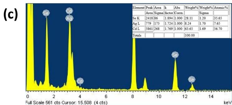
Figure S2. (a, b, and c) EDS spectra of 4 ML 5%, 7%, and 11% Ag: CdSe NPLs.
