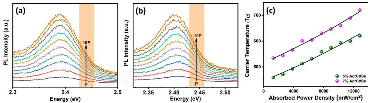
**Figure S7.** (a, b) Power-dependent PL of 5% and 7%Ag: CdSe NPLs respectively. (c) Carrier temperature increases with increasing power density (olive- 5% Ag: CdSe and purple- 7% Ag: CdSe NPLs)
