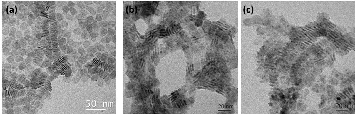
**Figure. S1.** (a, b, and c)TEM images of 4 ML undoped, 7%, and 11% Ag doped CdSe NPLs, respectively.
