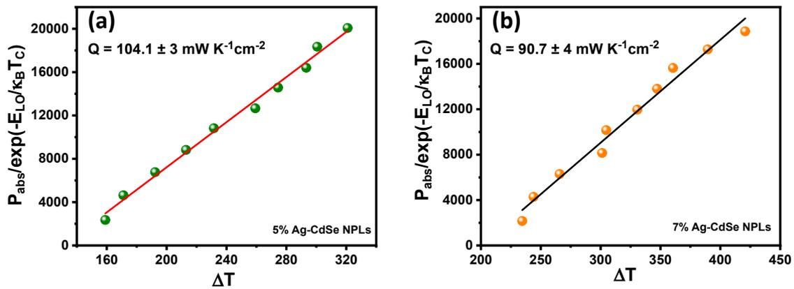
**Figure S8.** (a, b)  $P_{abs}/\exp\left(\frac{E_{LO}}{k_B T_C}\right)$  plot as a function of  $\Delta T$ , where slopes give the thermalization coefficient values ( $Q$ ) for 5% and 7% Ag-CdSe NPLs respectively.
