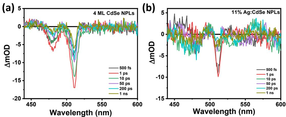
Figure S5. TA spectra of (a) undoped and (b) 11% Ag-doped CdSe NPLs.
