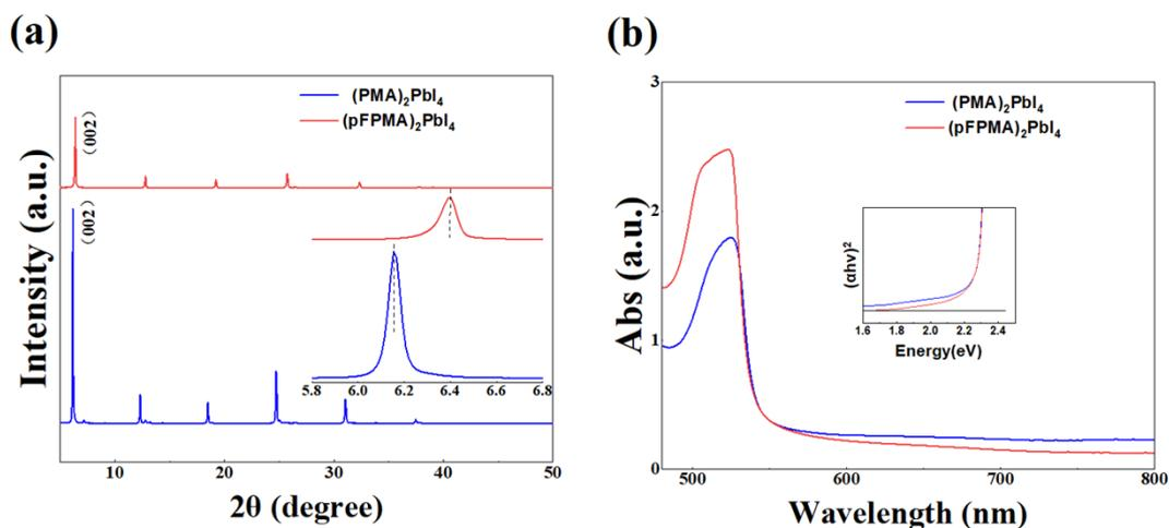
**Figure S1.** (a) XRD patterns of  $(\text{PMA})_2\text{PbI}_4$  and  $(\text{pFPMA})_2\text{PbI}_4$  films. The inset is the enlarged XRD patterns with  $2\theta$  between  $5.8^\circ$  and  $6.8^\circ$ . (b) UV-vis absorption spectra of the  $(\text{PMA})_2\text{PbI}_4$  and  $(\text{pFPMA})_2\text{PbI}_4$  films. The inset is the band gap of films.
