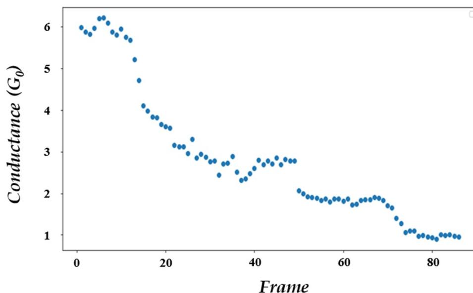
Figure S3 Typical conductance profile during the pulling of the silver compact nanowire.
