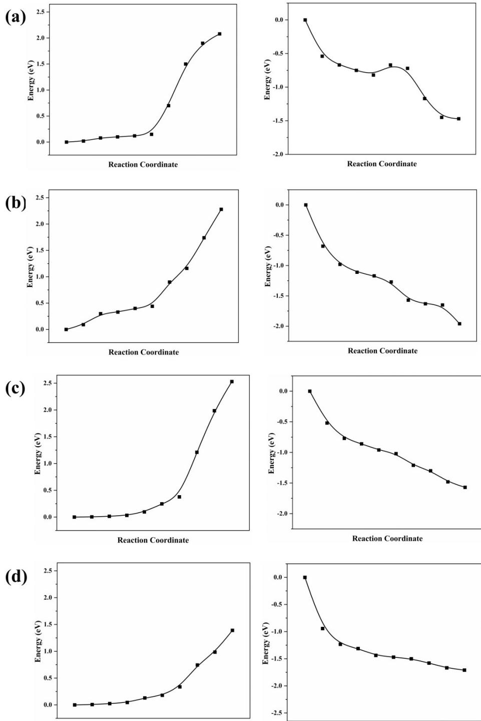
Fig. S8. Reaction pathways using Initial/transition states (IS/TS) as the start/end (left), and transition/final states TS/FS as the start/end (right), respectively. (a)  $\text{Fe}_6\text{N}_0$ , (b)  $\text{Fe}_6\text{N}_2$ , (c)  $\text{Fe}_6\text{N}_0@\text{graphene}$  and (d)  $\text{Fe}_6\text{N}_2@\text{graphene}$ .
