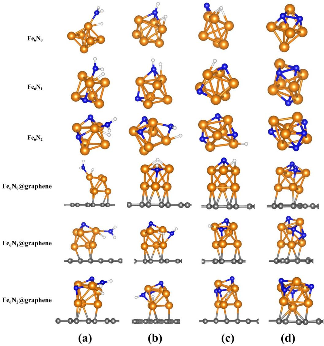
Fig. S7. Transition states (TS) for (a)  $\text{NH}_3^* \rightarrow \text{NH}_2^* + \text{H}^*$ , (b)  $\text{NH}_3^* \rightarrow \text{NH}^* + \text{H}^*$ , (c)  $\text{NH}^* \rightarrow \text{N}^* + \text{H}^*$  and (d)  $\text{N}^* + \text{N}^* \rightarrow \text{N}_2^*$ . Color codes follow Fig. S2.
