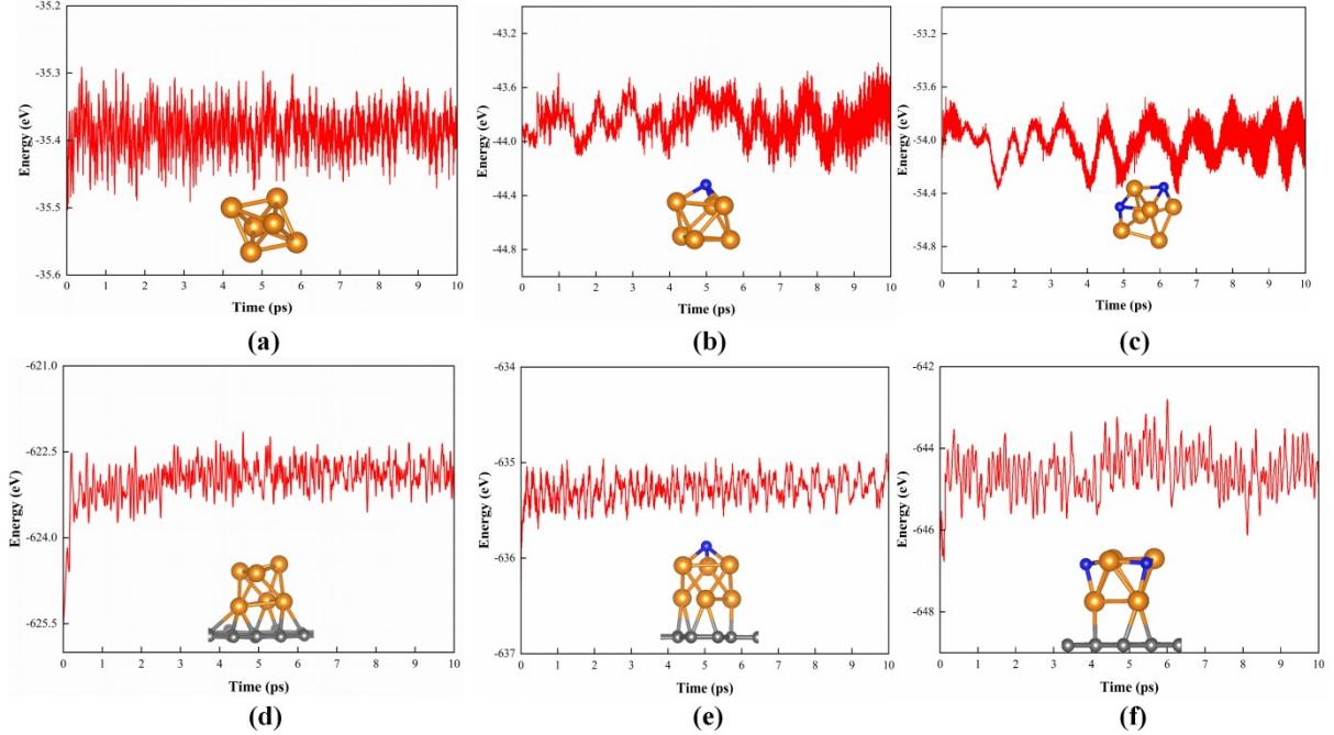
Fig. S1. AIMD simulations of (a) Fe<sub>6</sub>N<sub>0</sub>, (b) Fe<sub>6</sub>N<sub>1</sub>, (c) Fe<sub>6</sub>N<sub>2</sub>, (d) Fe<sub>6</sub>N<sub>0</sub>@graphene, (e) Fe<sub>6</sub>N<sub>1</sub>@graphene and (f) Fe<sub>6</sub>N<sub>2</sub>@graphene at 823 K. The C, N, and Fe atoms are colored in gray, blue, and orange, respectively.
