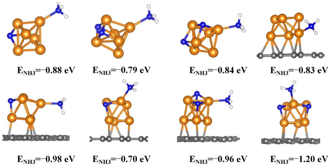
Fig. S3. Configurations and adsorption energies of  $NH_3$  at additional adsorption sites. Color codes follow Fig. S1, with H atoms depicted in white.
