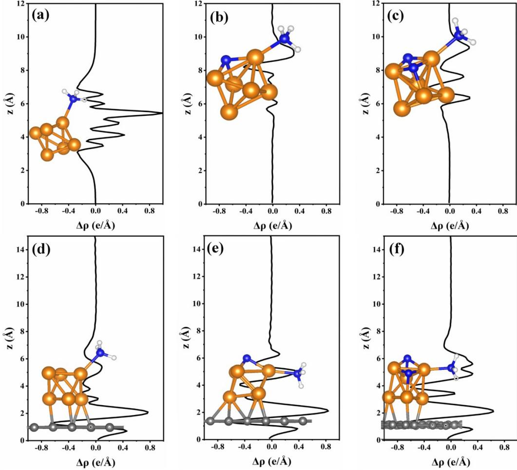
Fig. S5. Plane-averaged charge density difference plot along the z-axis for (a)  $\text{Fe}_6\text{N}_0$ , (b)  $\text{Fe}_6\text{N}_1$ , (c)  $\text{Fe}_6\text{N}_2$ , (d)  $\text{Fe}_6\text{N}_0@\text{graphene}$ , (e)  $\text{Fe}_6\text{N}_1@\text{graphene}$  and (f)  $\text{Fe}_6\text{N}_2@\text{graphene}$ . Color codes follow Fig. S1.
