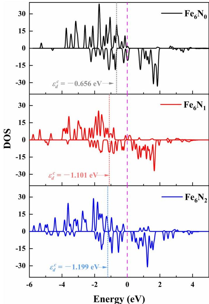
Fig. S4. d-projected density of states (PDOS) of Fe in (a)  $\text{Fe}_6\text{N}_0$ , (b)  $\text{Fe}_6\text{N}_1$  and (c)  $\text{Fe}_6\text{N}_2$  configurations.  $\varepsilon_d^c$  denotes the d-band center. The purple dashed line denotes the Fermi level set at 0 eV.
