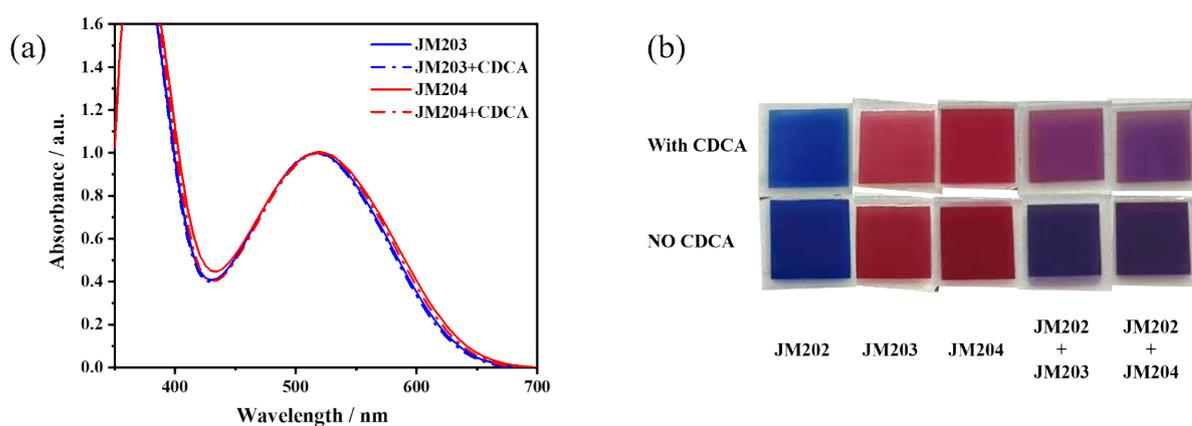
**Figure S1.** (a) UV-vis absorption spectra of sensitizers JM203/JM203+CDCA and JM204/JM204+CDCA attached on 4 μm TiO<sub>2</sub> film immersed in CH<sub>3</sub>CN solutions with 0.1 M LiClO<sub>4</sub>. (b) Photograph of dye adsorption on 6 μm TiO<sub>2</sub>.
