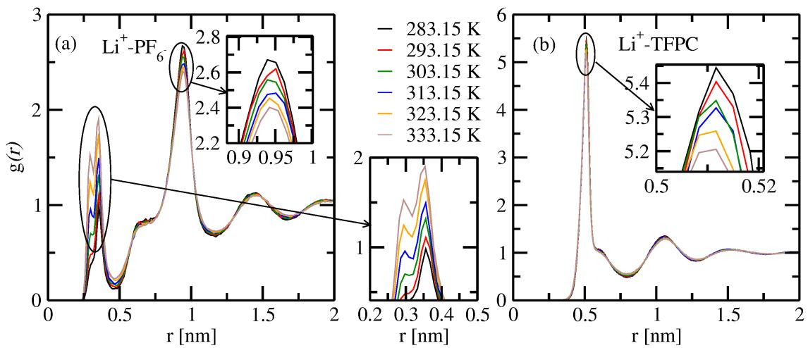
**Figure S1.** COM RDF of (a)  $\text{Li}^+\text{-}\text{PF}_6^-$ , and (b)  $\text{Li}^+\text{-TFPC}$ . Inset shows the zoomed view of the peaks.
