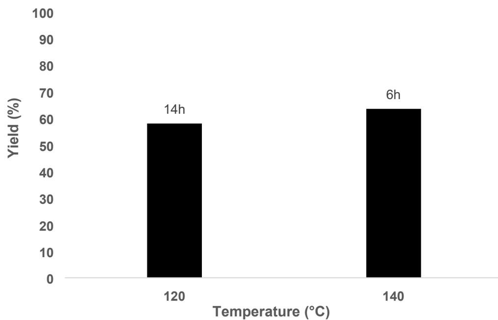
**Figure S19** Yield in LA at 120 and 140°C (5 wt% fructose in water)
