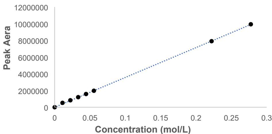
**Figure S1** Calibration curve of fructose
