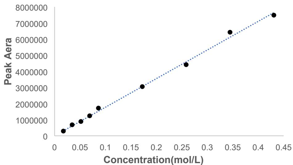
**Figure S2** Calibration curve of levulinic acid
