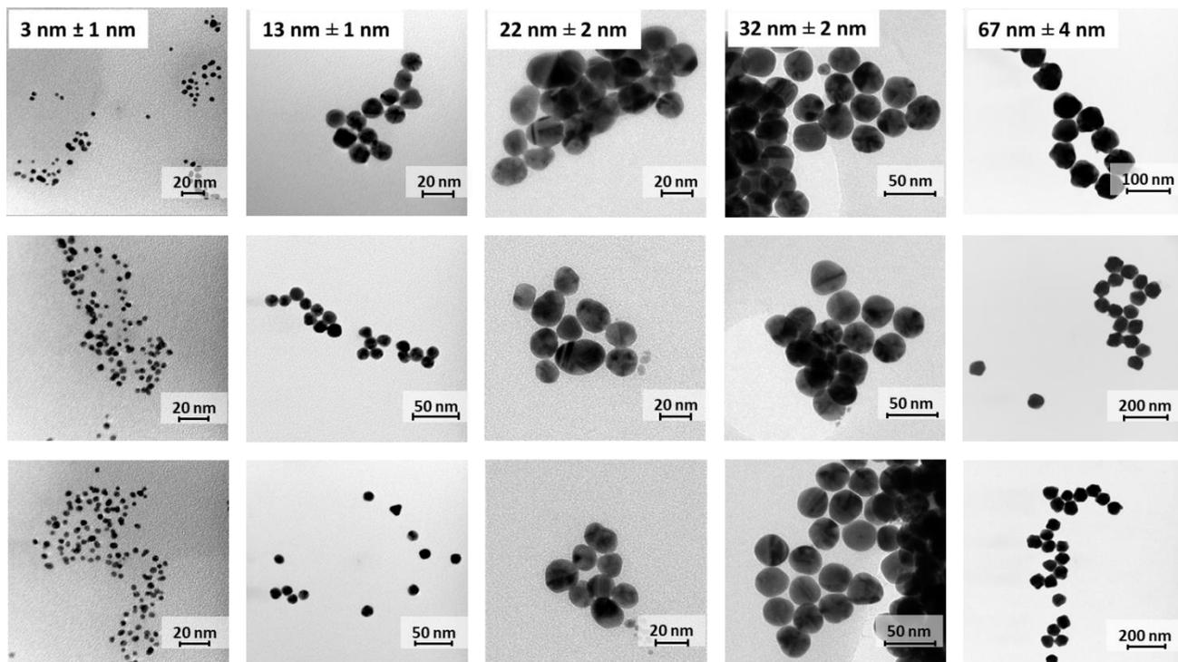
**Figure S1.** TEM images of gold nanoparticles with 3, 13, 22, 32 and 67 nm diameter.
