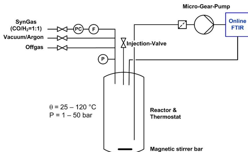
**Scheme S1.** Scheme of the HP FTIR-reactor system used for the *in situ* spectroscopic investigations within this study.
