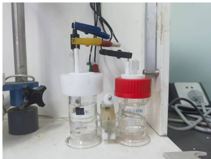
Figure S2. The image of a H-type electrolytic cells used for HER stability test.
