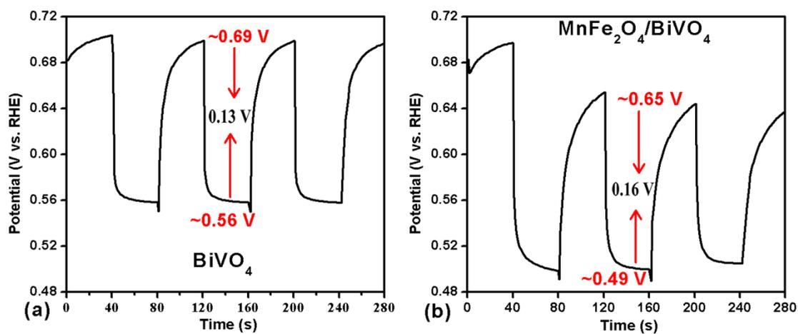
**Fig. S8** The OCP of BiVO<sub>4</sub> and MnFe<sub>2</sub>O<sub>4</sub>/BiVO<sub>4</sub> film photoanodes in 0.1 M NaPi under 1.5G illumination and in dark, respectively.
