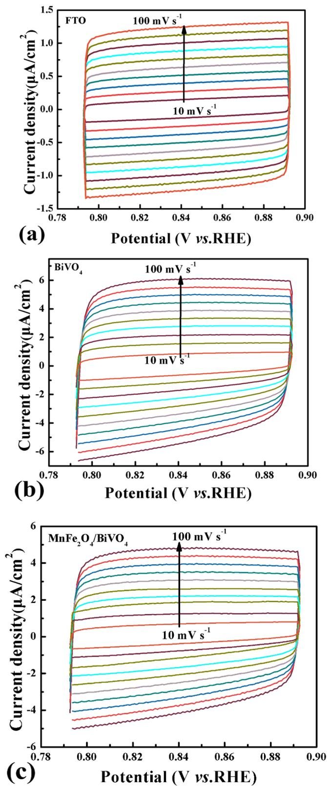
**Fig. S6** The  $\Delta I \sim \nu$  plots used for the calculation of double-layer capacitance ( $C_{dl}$ ) for (a) FTO, (b)  $\text{BiVO}_4$  and (c)  $\text{MnFe}_2\text{O}_4/\text{BiVO}_4$  electrode at 0.85 V vs. RHE.
