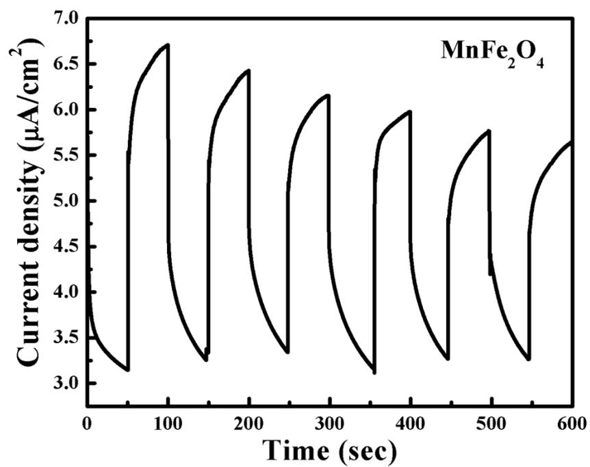
**Fig. S3** The photocurrent response of MnFe<sub>2</sub>O<sub>4</sub> film in 0.1 M NaPi at 1.23 V vs. RHE under AM 1.5G irradiation.
