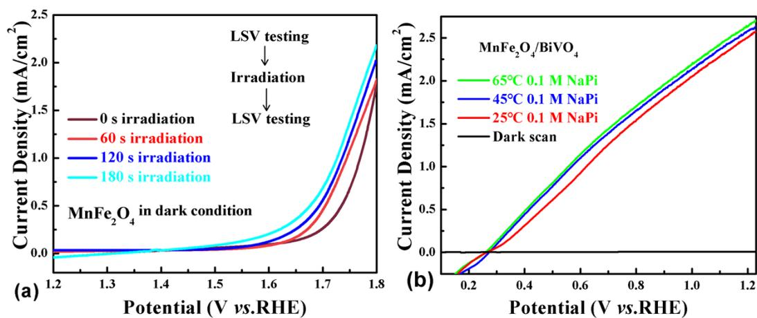
**Fig. S7** (a) LSV curves of  $\text{MnFe}_2\text{O}_4$  film electrode in 0.1 M NaPi in dark condition after different AM 1.5G irradiation times. (b) LSV curves of  $\text{MnFe}_2\text{O}_4/\text{BiVO}_4$  film in 0.1 M NaPi under/without AM 1.5G irradiation, the temperature of 0.1 M NaPi was controlled at different temperatures.
