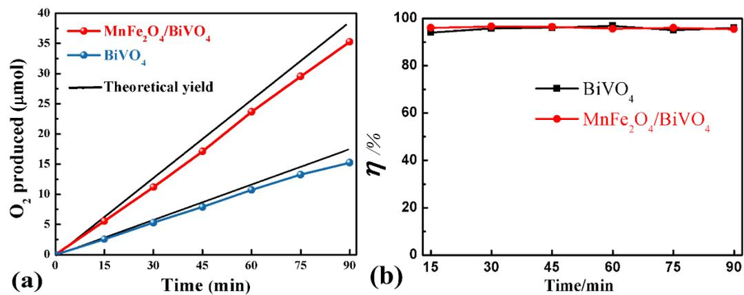
**Fig. S4** (a) The curves of O<sub>2</sub> generation vs. reaction time, and (b) faradic efficiency of oxygen evolution reaction on BiVO<sub>4</sub> and MnFe<sub>2</sub>O<sub>4</sub>/BiVO<sub>4</sub> film photoelectrode in 0.1 M NaPi under AM 1.5G irradiation at 1.23 V vs. RHE.
