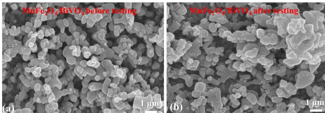
**Fig. S5** SEM image of MnFe<sub>2</sub>O<sub>4</sub>/BiVO<sub>4</sub> film photoanode (a) before and (b) after 2 h of testing in 0.1 M NaPi at 1.23 vs. RHE under AM 1.5G irradiation.
