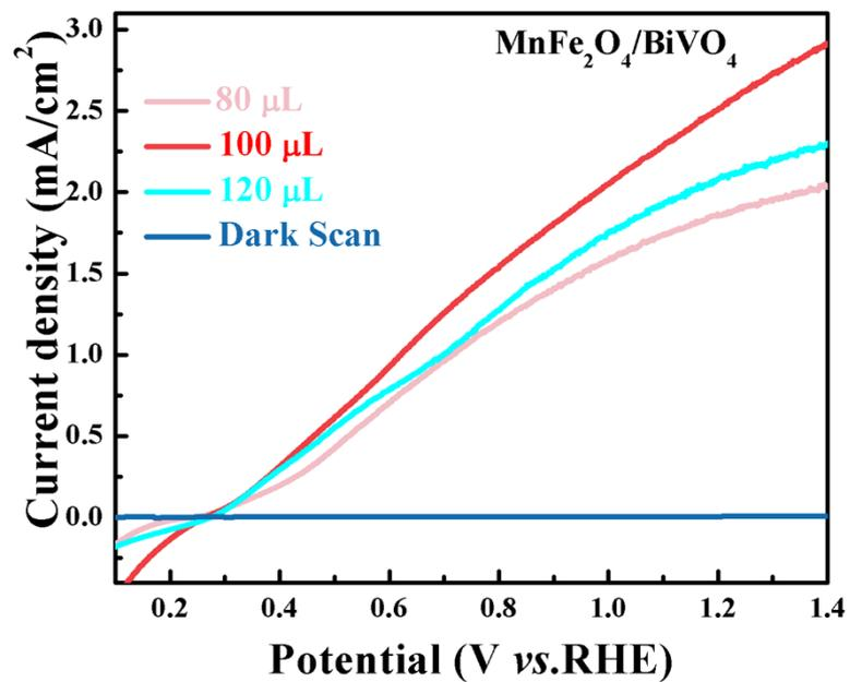
**Fig. S2** LSV curves of the MnFe<sub>2</sub>O<sub>4</sub>/BiVO<sub>4</sub> films in 0.1 M NaPi under AM 1.5G irradiation. The MnFe<sub>2</sub>O<sub>4</sub>/BiVO<sub>4</sub> films were prepared using different MnFe<sub>2</sub>O<sub>4</sub>-containing suspensions on BiVO<sub>4</sub> film.
