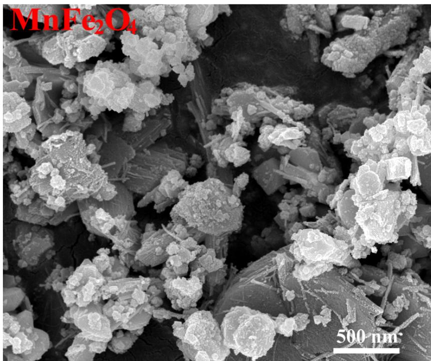
**Fig. S1** SEM image of MnFe<sub>2</sub>O<sub>4</sub> sample.
