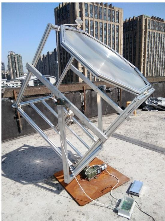
Figure S2 The picture of the outdoor reactor system with nature solar light source
