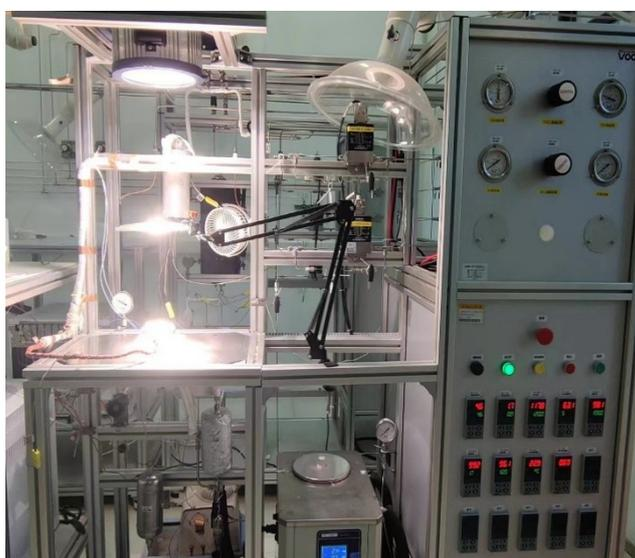
Figure S1 The picture of the indoor reactor system with simulated light source
