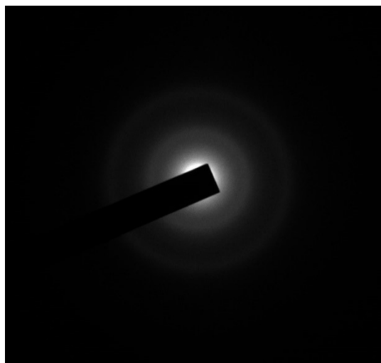
Figure S5. SAED pattern of recovered catalyst
