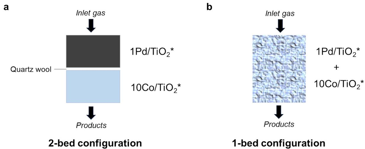
**Figure S14.** Different configurations used for the monometallic catalysts: **a** 2-beds configuration; and **b** 1-bed configuration.
