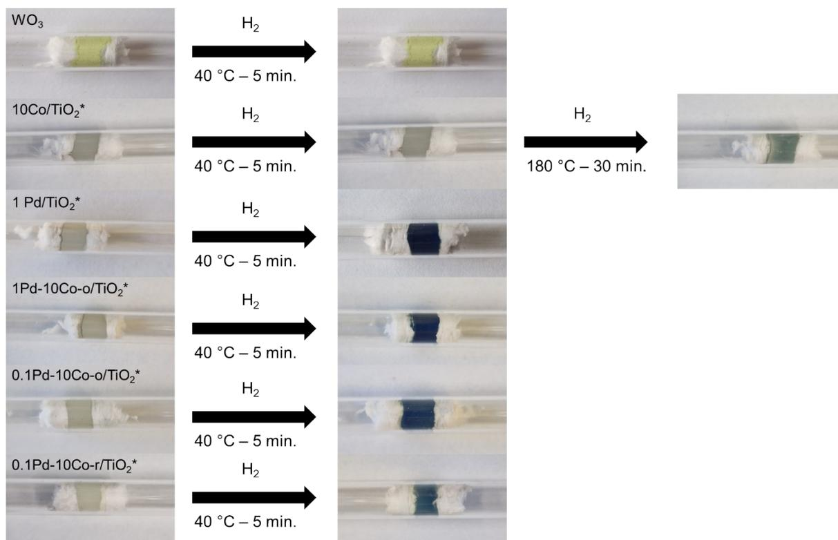
**Figure S7.** Photographs of samples made with 1 g of  $\text{WO}_3$  mixed or not with 5 mg of the catalysts investigated in this study before (left) and after (right) treatment with  $\text{H}_2$  ( $10\text{ mL min}^{-1}$ ) at  $40\text{ }^\circ\text{C}$  for 5 min.
