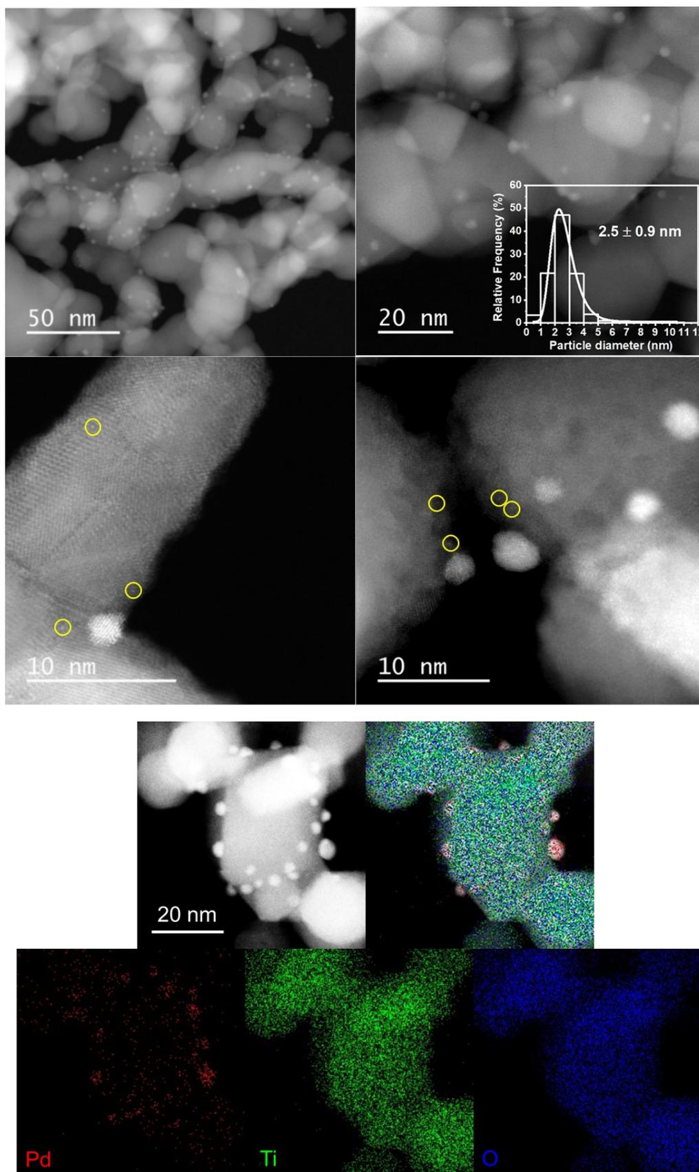
**Figure S2.** HAADF-STEM micrographs with Pd particle size distribution and EDX analysis of the reduced 1Pd/TiO<sub>2</sub>\* catalyst. Pd single atoms are surrounded by a yellow circle for better visualization.
