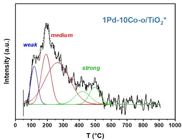
**Figure S12.** CO<sub>2</sub>-TPD profiles and deconvolutions of mono and bimetallic catalysts.
