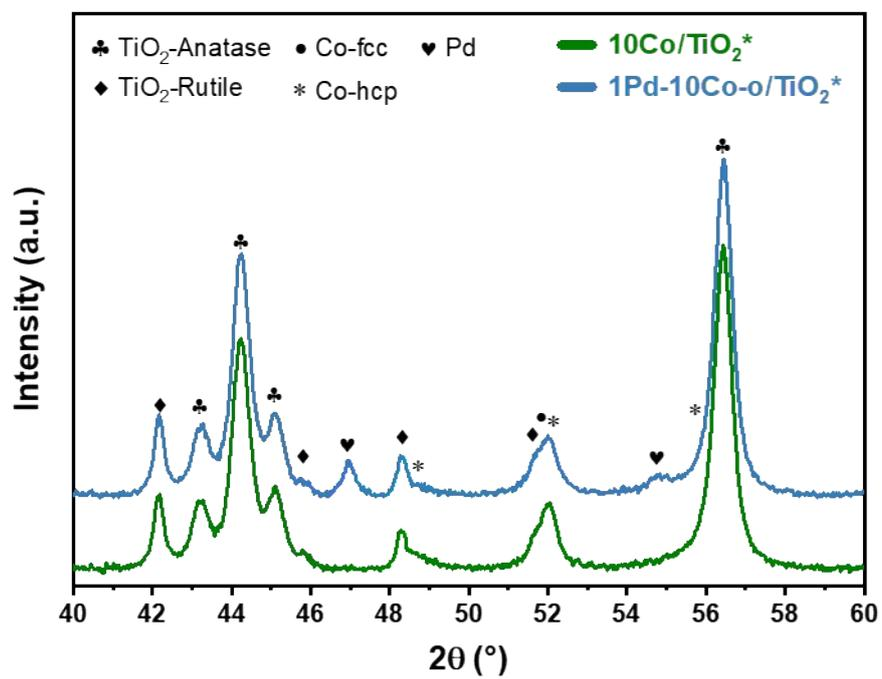
**Figure S10.** XRD diffractograms (40°-60°) of the 10Co/TiO<sub>2</sub>\* and 1Pd-10Co-o/TiO<sub>2</sub>\* catalysts.
