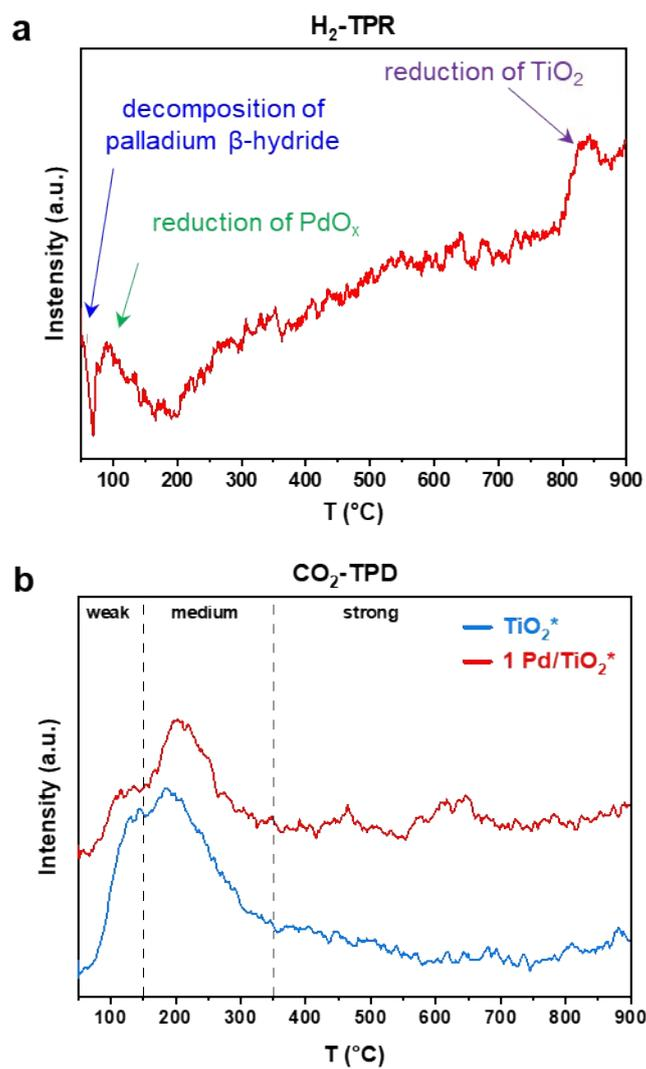
**Figure S4.** **a**  $H_2$ -TPR profile of the  $1Pd/TiO_2^*$  catalyst; and **b**  $CO_2$ -TPD profiles of the  $1Pd/TiO_2^*$  catalyst and of the  $TiO_2^*$  support.
