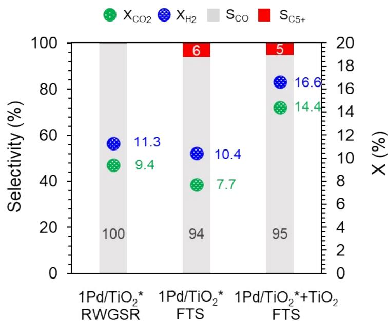
**Figure S6.** Conversions  $X$  ( $\text{CO}_2$ : green;  $\text{H}_2$ : blue) and selectivity ( $\text{CO}$ : grey;  $\text{C}_{5+}$ : red) for the 1%Pd/TiO<sub>2</sub>\* catalyst at 60 hours on stream under various conditions,  $T = 220\text{ }^\circ\text{C}$ ,  $P = 20\text{ bar}$ ,  $\text{WHSV} = 1620\text{ mL}_{\text{g}_{\text{cat}}}^{-1}\text{ h}^{-1}$ . RWGSR and FTS correspond to the feeding ratio of  $\text{H}_2/\text{CO}_2 = 1/1$  and  $2/1$ , respectively.
