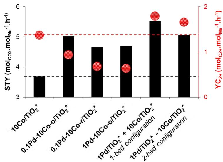
**Figure S15.** STY (mol<sub>CO2</sub> mol<sub>Me</sub><sup>-1</sup> h<sup>-1</sup>) and yields Y (mol<sub>Z</sub> mol<sub>Me</sub><sup>-1</sup> h<sup>-1</sup>, Z = C<sub>2+</sub>) of the mono- and bimetallic catalysts at 25 hours on stream, T = 220 °C, P = 20 bar, WHSV = 1620 mL g<sub>cat</sub><sup>-1</sup> h<sup>-1</sup>.
