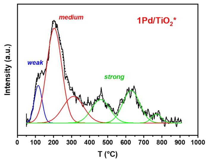
**Figure S5.** CO<sub>2</sub>-TPD profiles and deconvolutions of the support and the 1Pd/TiO<sub>2</sub>\* catalyst.
