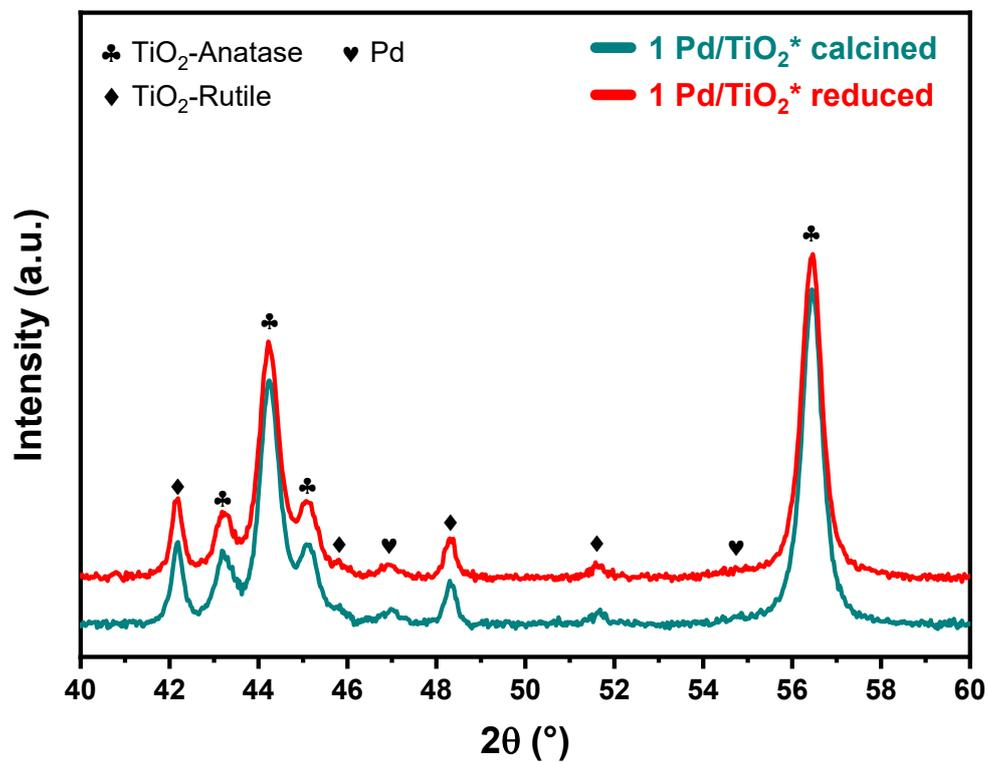
**Figure S1.** XRD diffractograms (40°-60°) of the 1Pd/TiO<sub>2</sub>\* catalyst after calcination and subsequent reduction (4 h, 350 °C, 40% H<sub>2</sub>/Ar).
