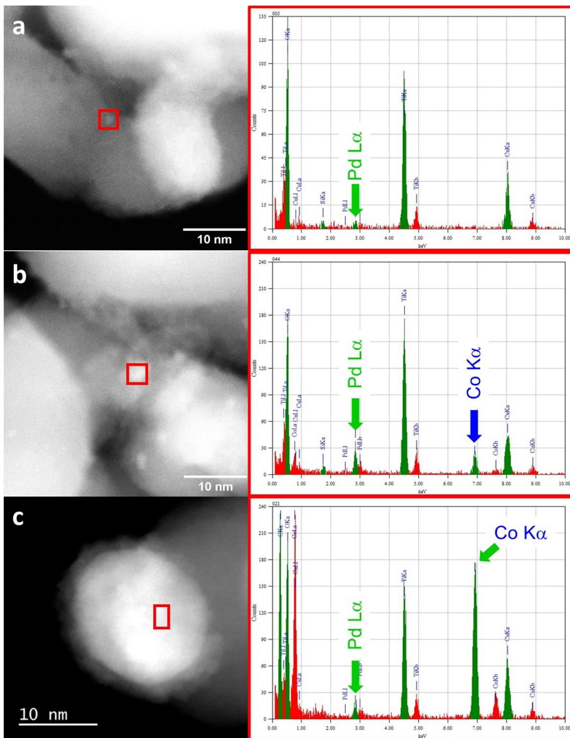
**Figure S8.** HAADF-STEM micrographs and EDX analysis of the reduced: **a** and **b** 0.1Pd-10Co-o/TiO<sub>2</sub>\*; and **c** 0.1Pd-10Co-r/TiO<sub>2</sub>\* catalysts.
