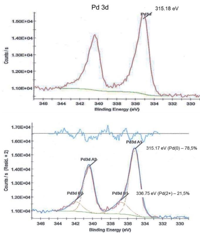
**Figure S3.** High-resolution XPS spectrum of Pd 3d of the sample 1Pd/TiO<sub>2</sub>\*.
