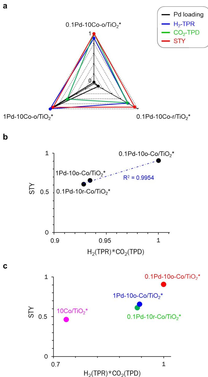
**Figure S13.** **a** Radar chart including the main measured parameters and the measured STY on a 0-1 scale. **b** Correlation between the two most relevant parameters and STY taken the values calculated on a 0-1 scale. **c** Correlation between the two most relevant parameters and STY taken the values calculated on a 0-1 scale for the 10Co/TiO<sub>2</sub>\* catalyst and the bimetallic catalysts.
