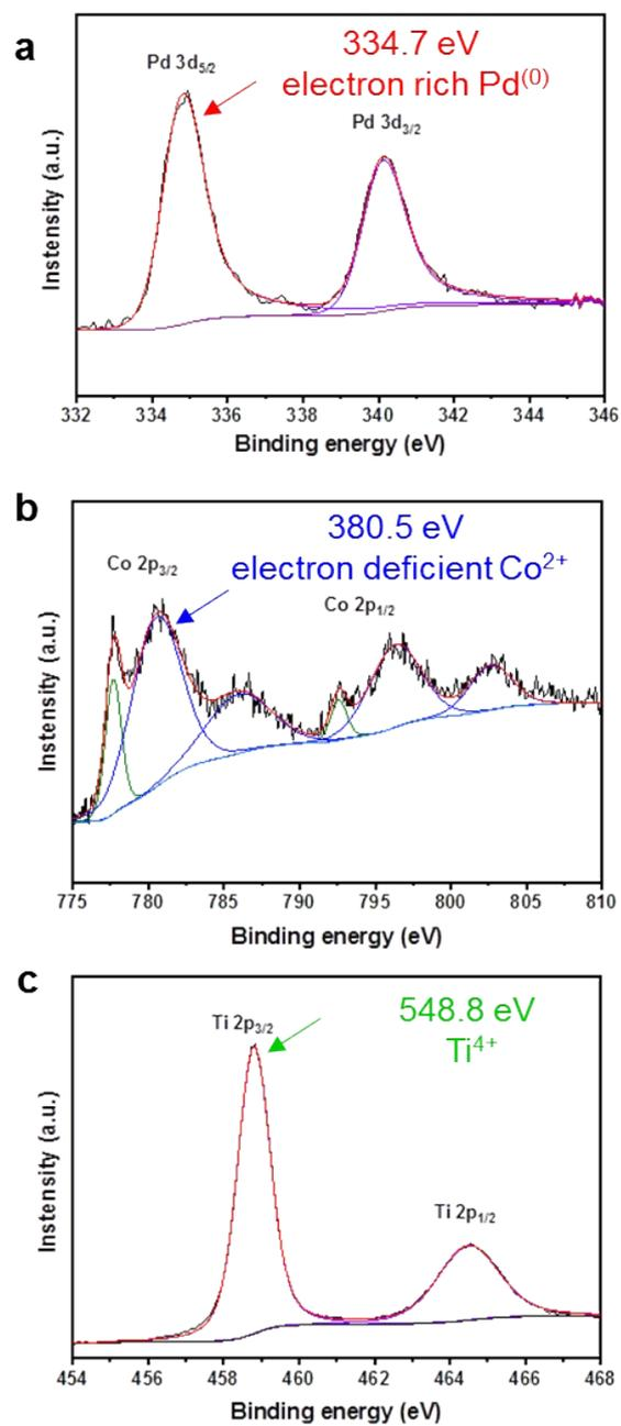
**Figure S11.** High-resolution XPS spectra of: **a** Pd 3d; **b** Co 2p; and **c** Ti 2p regions of the 1Pd-10Co-o/TiO<sub>2</sub>\* catalyst.
