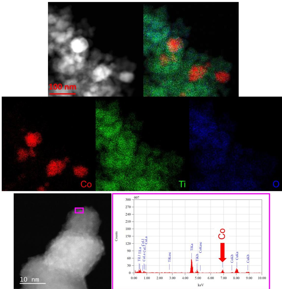
**Figure S9.** HAADF-STEM micrographs and EDX analysis of the reduced 10Co/TiO<sub>2</sub>\* catalyst.
