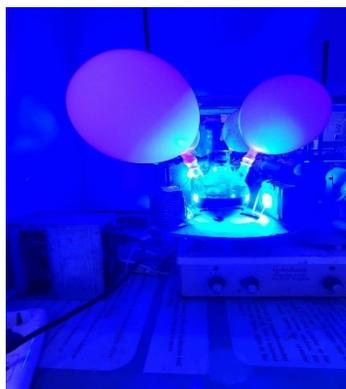
**Figure S2.** Batch photoreactor for large scale reaction
