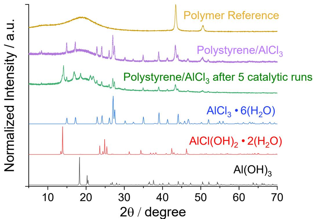
**Figure S13.** Normalized PXRD patterns of the polymer reference without AlCl<sub>3</sub> (yellow), the polymer-bound AlCl<sub>3</sub> composite before (violet) and after 5 catalytic runs (green). The diffractograms of AlCl<sub>3</sub> · 6(H<sub>2</sub>O) (ICSD-22071, blue), AlCl(OH)<sub>2</sub> · 2(H<sub>2</sub>O) (ICSD-425880, red) and Al(OH)<sub>3</sub> (ICSD-6162, black) are shown for comparison.
