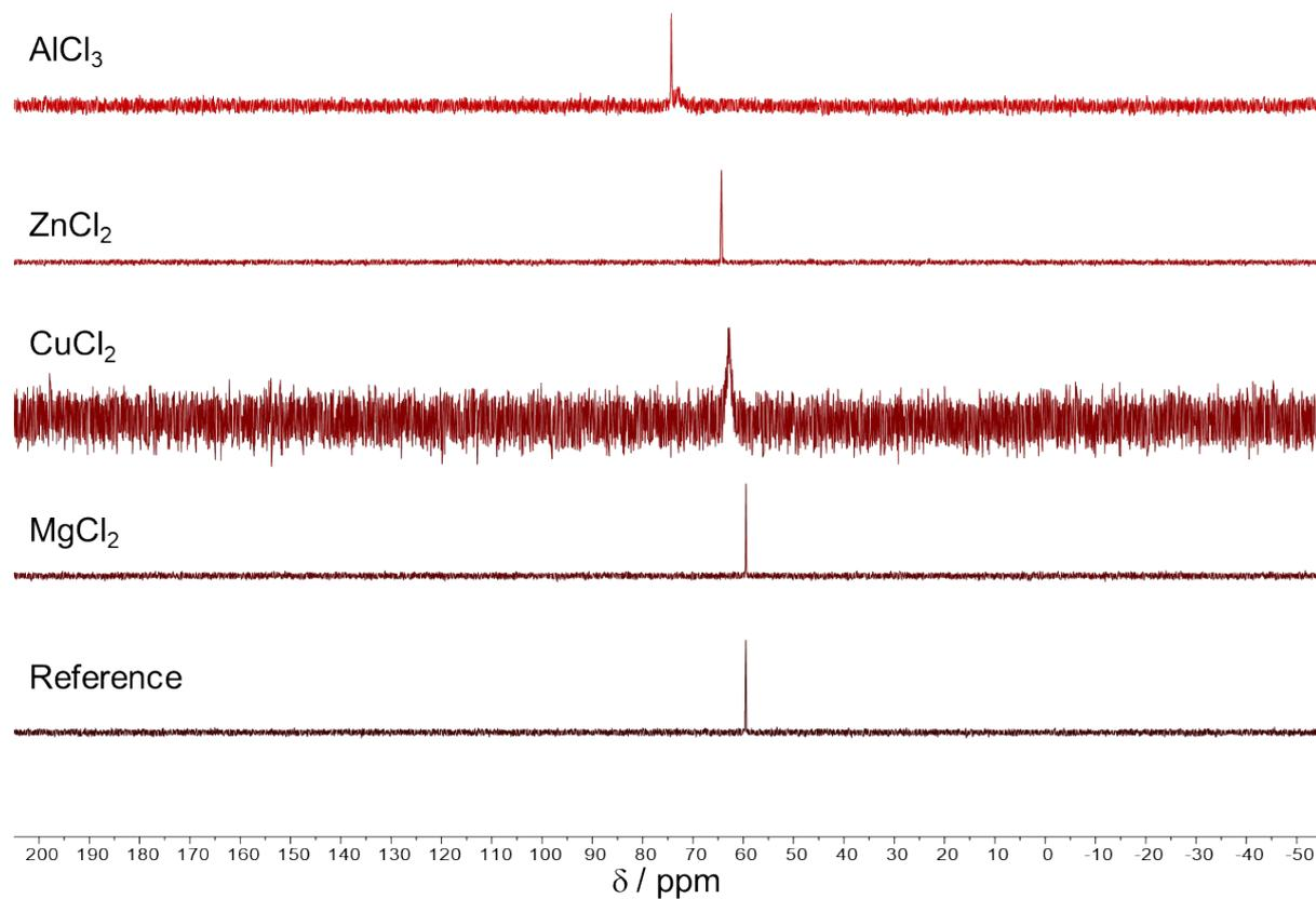
**Figure S1.**  $^{31}\text{P}$  NMR spectra of TEPO in the presence of different LAs; spectra were recorded in  $\text{MeOH-d}_4$ .
