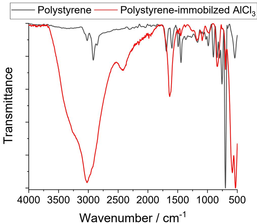
**Figure S9.** ATR-IR spectra of polystyrene (black) and  $\text{AlCl}_3$  immobilized in polystyrene (red)
