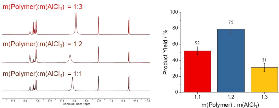
**Figure S14** <sup>1</sup>H-NMR-spectra of **3a** using polymer-bound AlCl<sub>3</sub> prepared with different polymer-to-AlCl<sub>3</sub> mass ratios as catalyst in under bulk conditions at 160°C; spectrum was recorded in DMSO-d<sub>6</sub> (left) and comparison of the obtained product yields (right) rationalizing the 1:2 polymer:AlCl<sub>3</sub> ratio used in all further experiments
