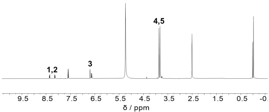
**Figure S8** <sup>1</sup>H-NMR-spectrum of **3f** using polymer-bound AlCl<sub>3</sub> as catalyst in under bulk conditions at 160°C; spectrum was recorded in DMSO-d<sub>6</sub>
