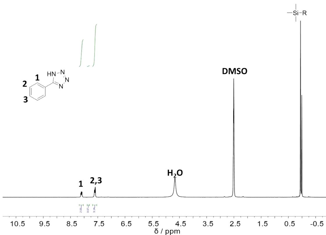
**Figure S2** <sup>1</sup>H-NMR-spectrum of 5-phenyltetrazole formation reaction using AlCl<sub>3</sub> as catalyst in under bulk conditions at 160°C; spectrum was recorded in DMSO-d<sub>6</sub>.
