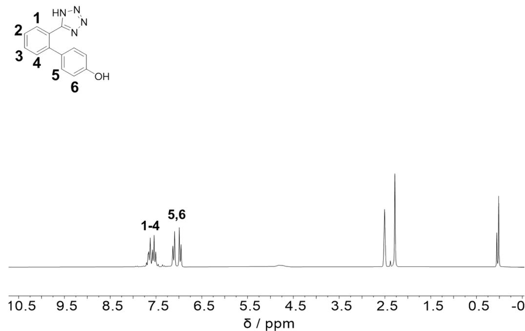
**Figure S5** <sup>1</sup>H-NMR-spectrum of **3c** using polymer-bound AlCl<sub>3</sub> as catalyst in under bulk conditions at 160°C; spectrum was recorded in DMSO-d<sub>6</sub>.
