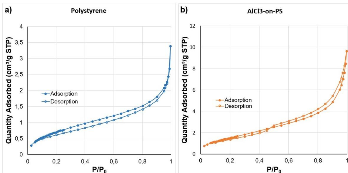
Figure S10. N<sub>2</sub> adsorption isotherms. a) Polystyrene sample. b) AlCl<sub>3</sub>-on-PS
