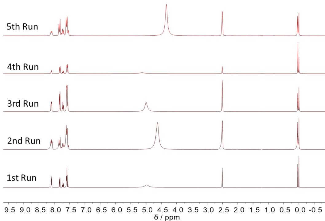
**Figure S3** <sup>1</sup>H-NMR-spectra of the formation of 5-phenyltetrazole tetrazole using Polymer-bound AlCl<sub>3</sub> as catalyst under bulk conditions at 160°C; for all runs, the catalyst was recycled and used again; spectra were recorded in DMSO-d<sub>6</sub>.
