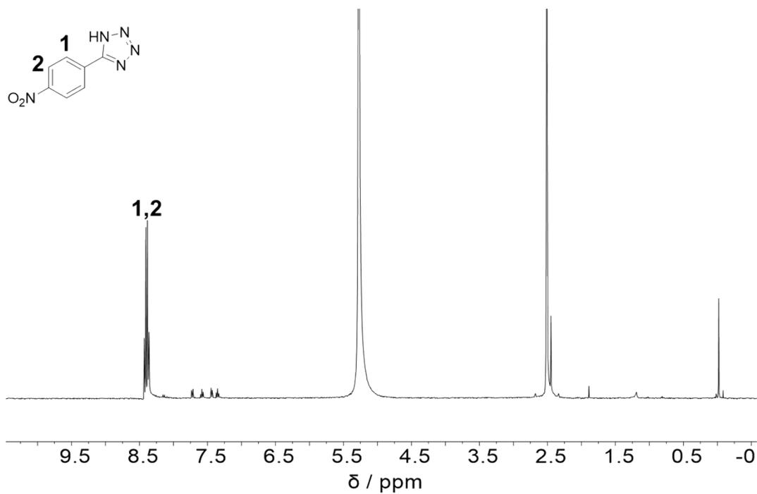
**Figure S6** <sup>1</sup>H-NMR-spectrum of **3d** using polymer-bound AlCl<sub>3</sub> as catalyst in under bulk conditions at 160°C; spectrum was recorded in DMSO-d<sub>6</sub>.
