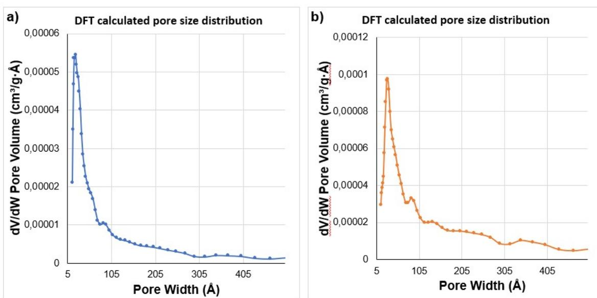
Figure S12. Pore size distribution analysis obtained from Density Functional Theory (DFT)
