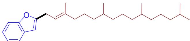
According to General Procedure B, phytol (0.59 mL; 1.7 mmol) was reacted with 2,3-benzofuran (1.9 mL; 17.2 mmol) in the presence of Perlkat 46-10 (125 mg) and 1,2-dichloroethane (2 mL) at 60 °C. After removal of excess furan under vacuum on a Schlenk line at 70 °C, the crude reaction mixture was purified by flash column chromatography (circa 270 mL silica gel; hexanes) to give the product as a colorless oil (449 mg; 66%).
