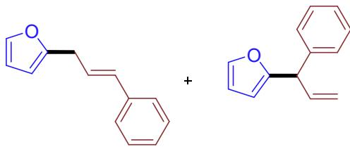
According to General Procedure A, cinnamyl alcohol (228 mg; 1.7 mmol) was reacted with furan (1.2 mL; 16.5 mmol) in the presence of CBV720CY (250 mg). The crude reaction mixture was purified by flash column chromatography (circa 50 mL silica gel; hexanes) to give the product as a colorless oil (236 mg; 75%).
