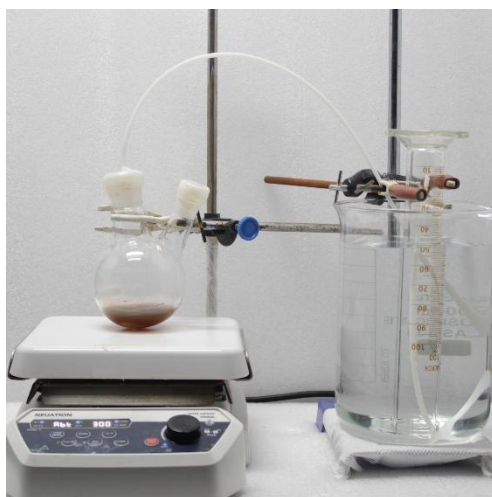
Figure S1. Experimental set-up used for FA reaction over different supported Pd catalysts.
