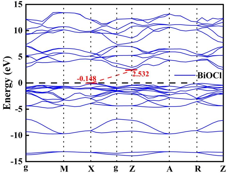
Figure S1. Band structure of BiOCl
