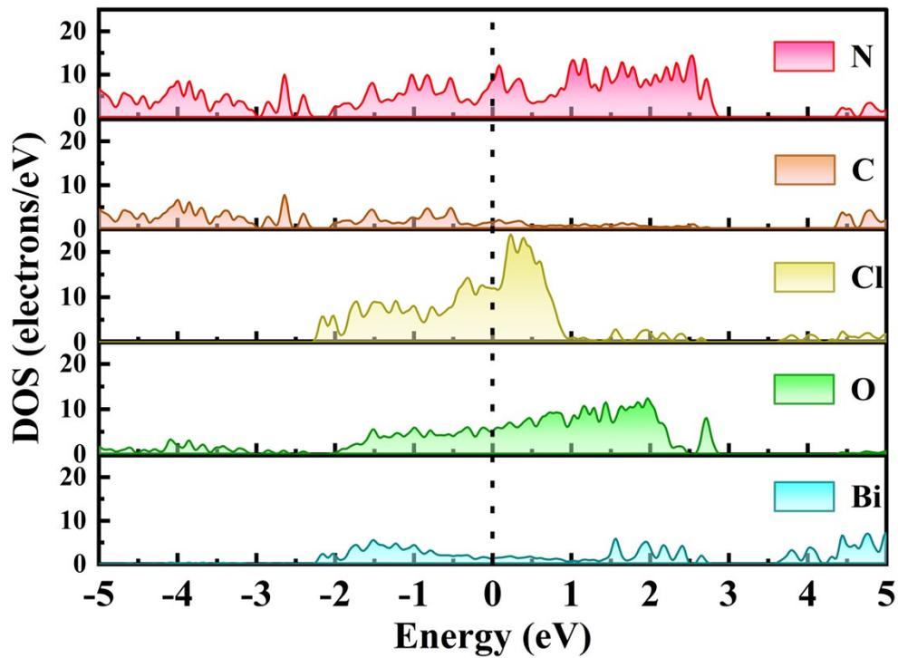
Figure S3. Partial density of states (PDOS) of each atom in BiOCl/g-C<sub>3</sub>N<sub>4</sub> heterojunction
