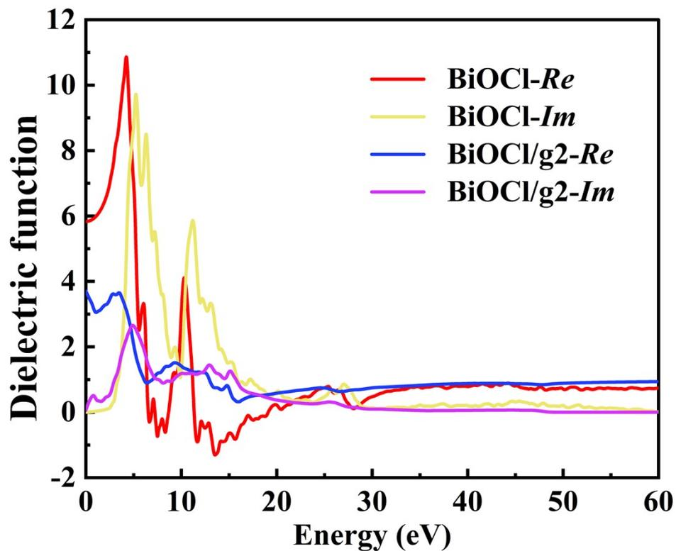
Figure S4. Real part (*Re*) and imaginary part (*Im*) of dielectric function for BiOCl and BiOCl/g-C<sub>3</sub>N<sub>4</sub> heterojunction, respectively
