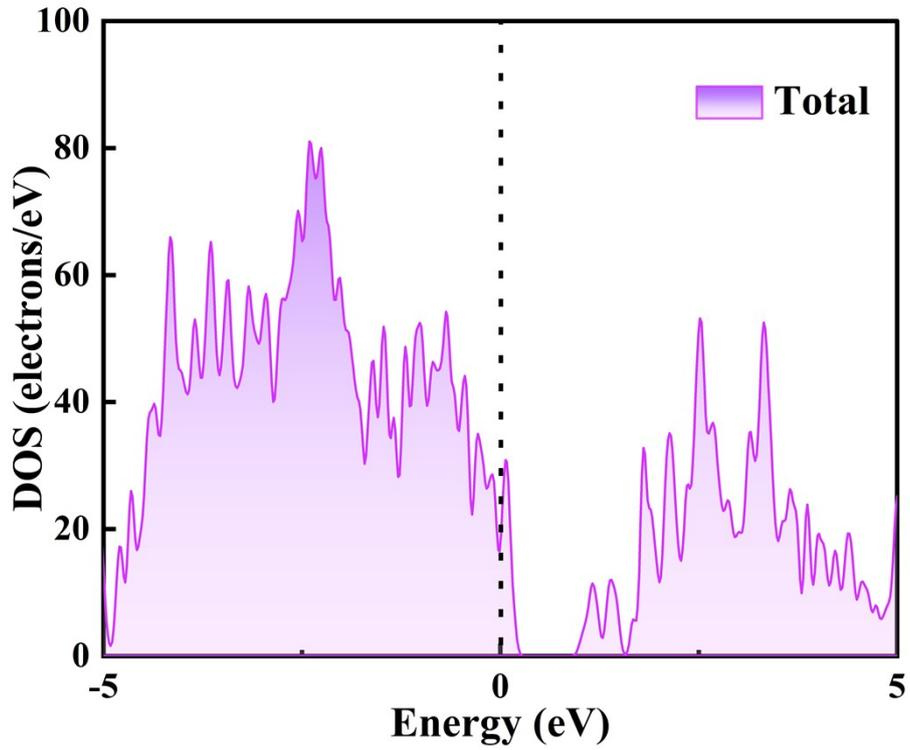
Figure S2. Total density of states (TDOS) of BiOCl/g-C<sub>3</sub>N<sub>4</sub> heterojunction
