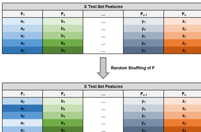
Figure S45 - Graphical explanation for how feature shuffling was performed. Each feature was individually randomly shuffled to create a new X test set that is used to evaluate how important that feature is relative to the target.
