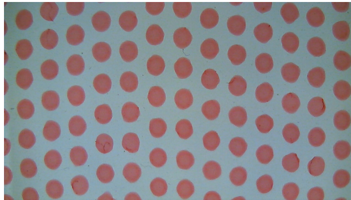
Fig. S-5 Red dyed water droplets generated using the droplet generator and PWM driver with settings of 5 Hz and 11% duty cycle.
