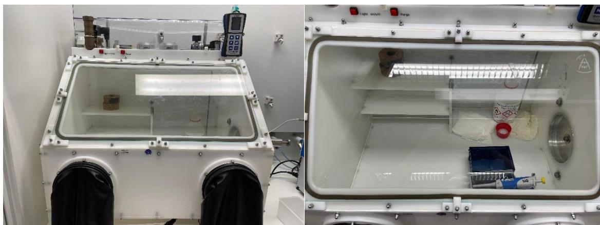
**Figure S1.** Custom glove box equipped with Orbitec OXY SMART Oxygen Analyser.
