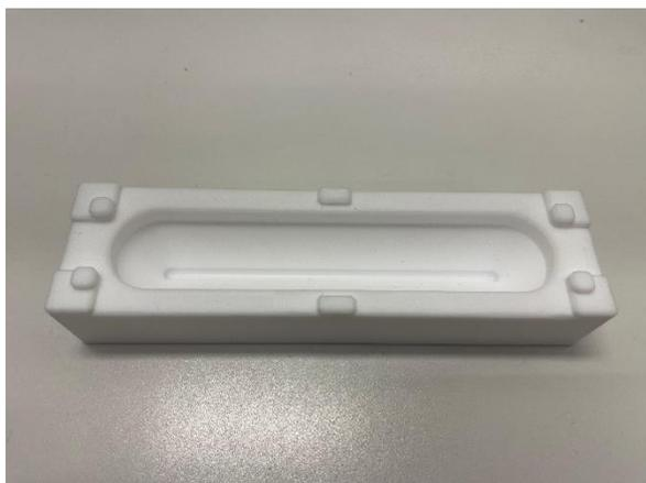
**Figure S2.** Custom-made polytetrafluorethylene (PTFE) reservoir.
