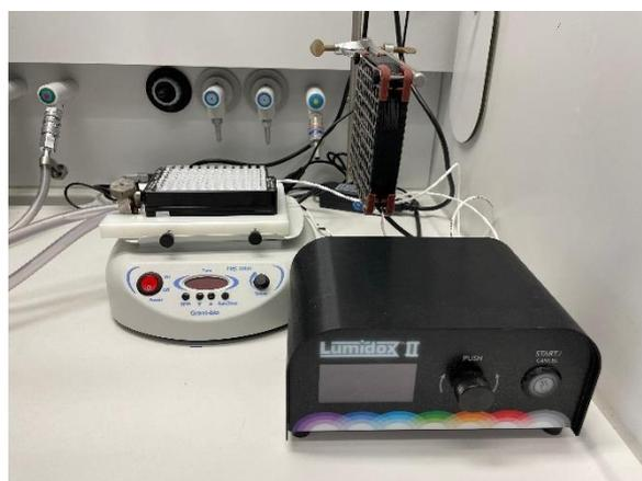
**Figure S4.** Photo setup for 96-well blocks with 445 nm Lumidox® II 96-Well LED Array equipped with a custom water-cooled base, a Noctua NF-A14 industrial PPC-3000 cooling fan and a Grant-Bio PMS-1000i orbital shaker.
