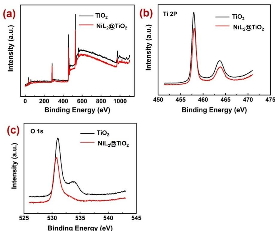
**Fig. S1** XPS results for TiO<sub>2</sub> and NiL<sub>2</sub>@TiO<sub>2</sub> (a) Full; (b) deconvoluted Ti 2p; (c) deconvoluted O1s.
