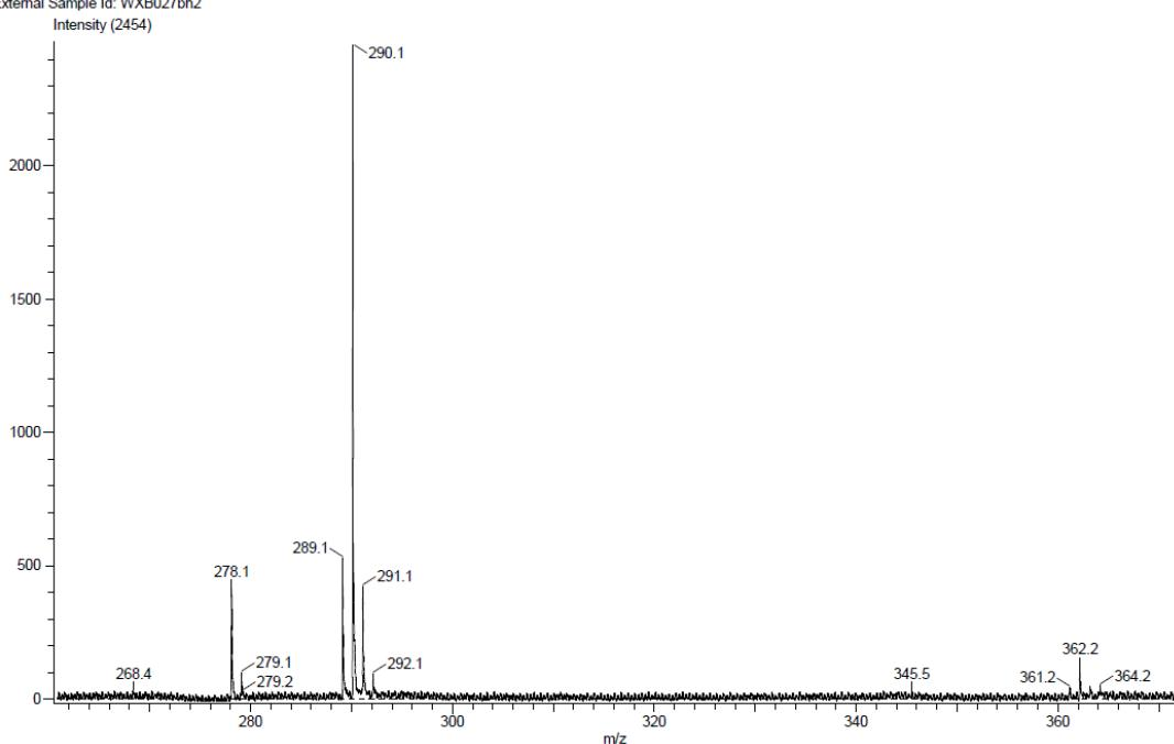
**Figure S8:** Mass spectrum (LIFDI[+], THF) of **1** (2 of 2).
