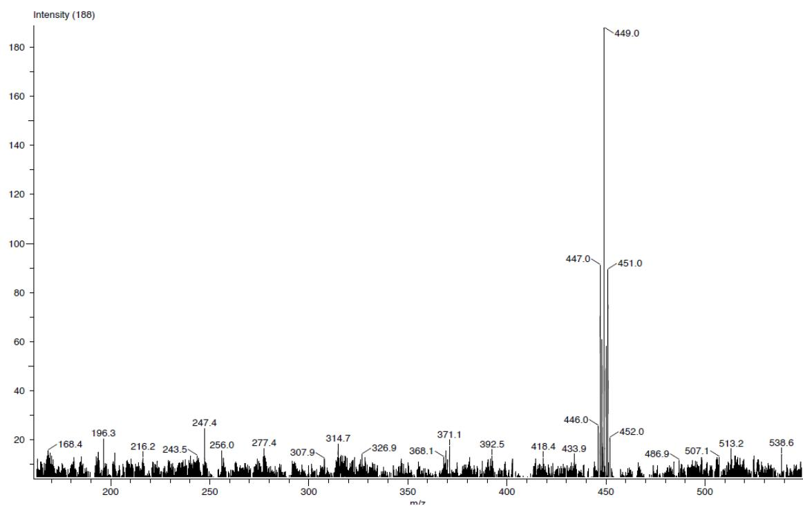
**Figure S23:** Mass spectrum (LIFDI[+], toluene) of **4**.
