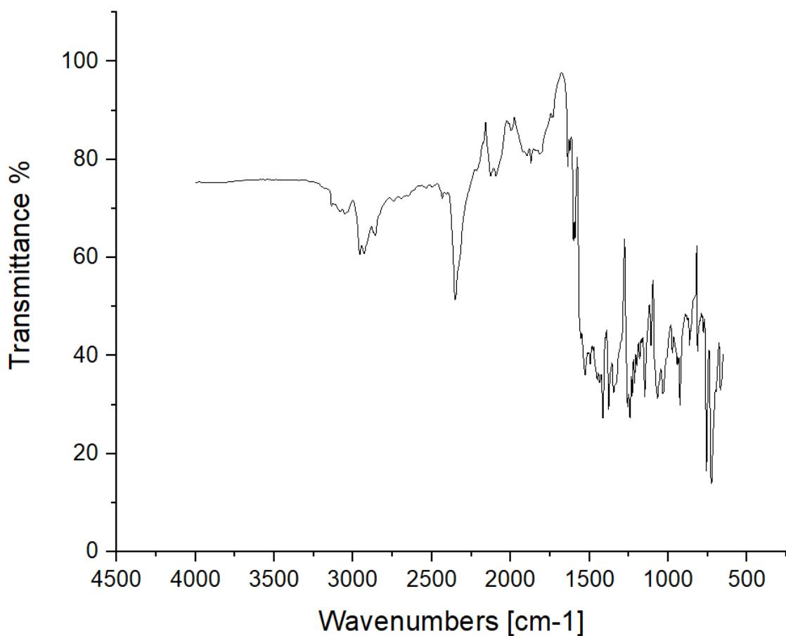
**Figure S24:** ATR-IR spectra (solid, 650–4000 cm<sup>-1</sup>) of compound 1.
