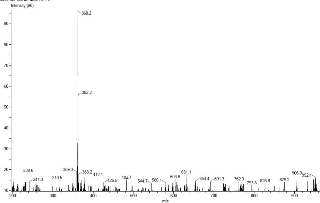
**Figure S19:** Mass spectrum (LIFDI[+], toluene) of **3** (1 of 2).
