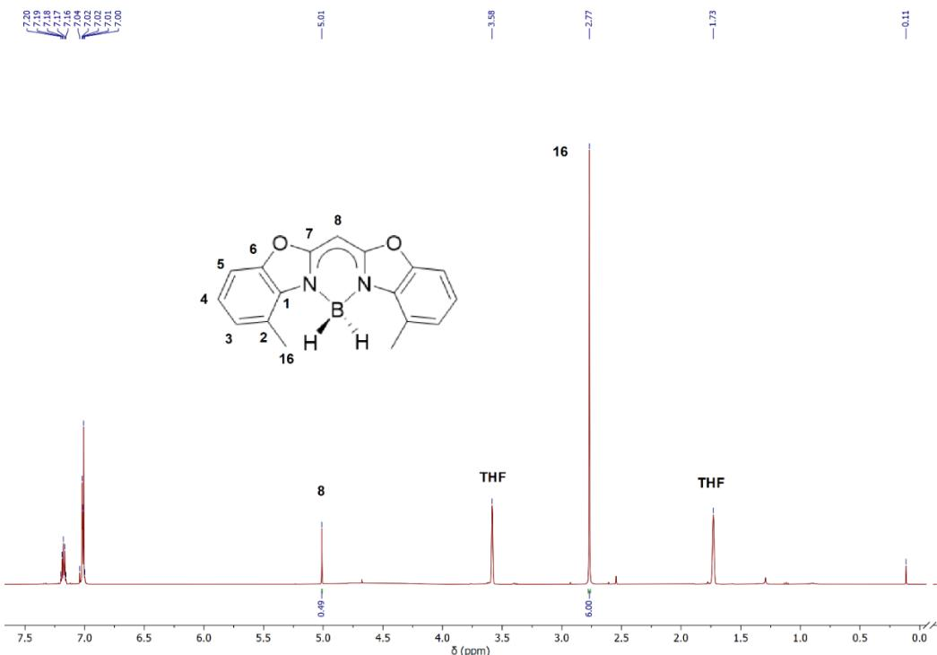
**Figure S1:**  $^1\text{H}$  NMR spectrum of **1** in  $\text{THF}-d_8$ .
