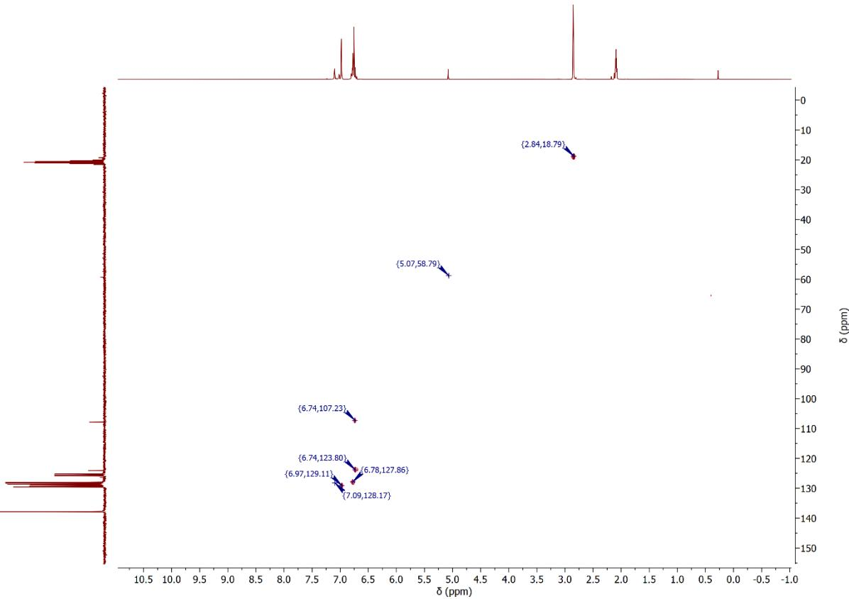
**Figure S15:**  $^1\text{H}$ ,  $^{13}\text{C}$  HSQC NMR spectrum of **2** in  $\text{tol}-d_8$ .
