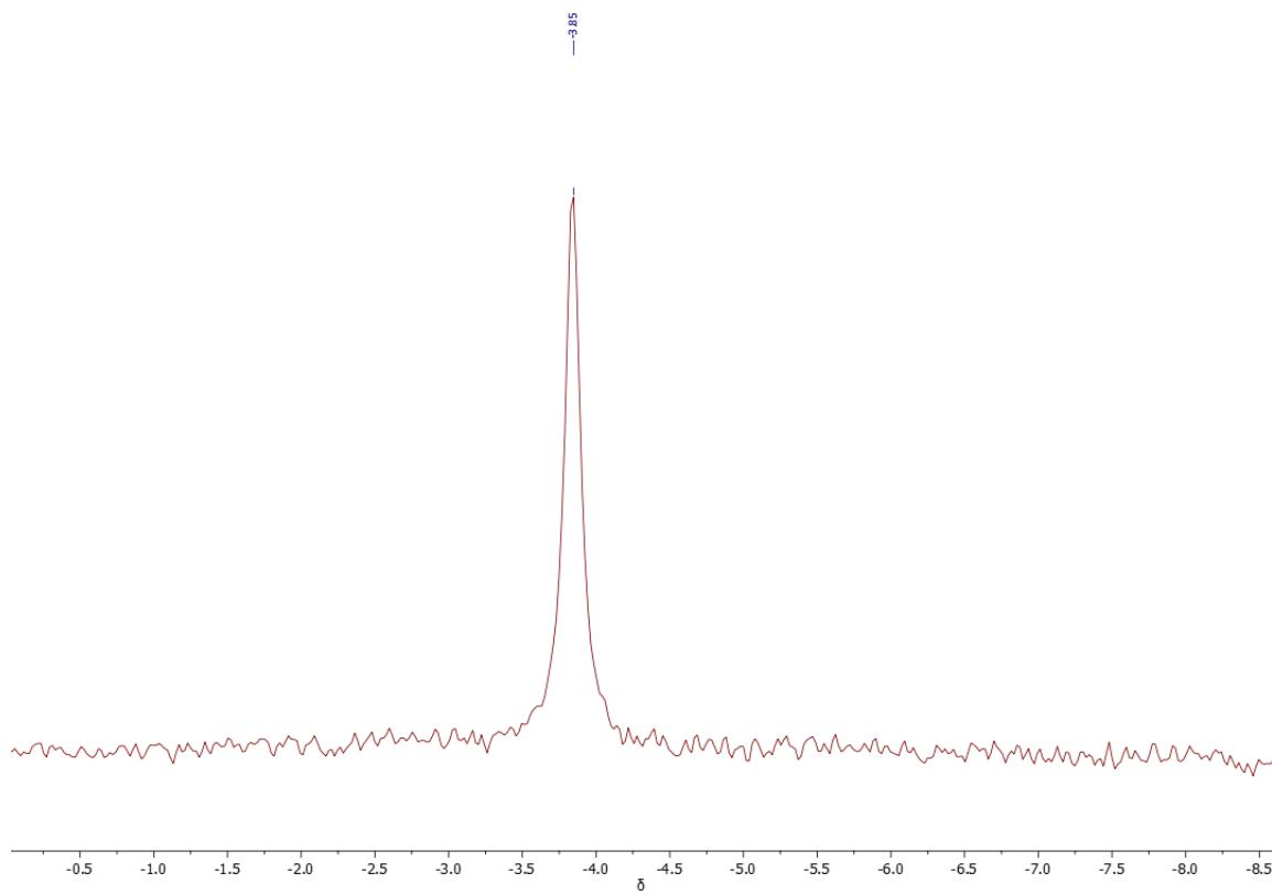
**Figure S22:** <sup>11</sup>B NMR spectrum of **4** in *THF-d*<sub>8</sub>.
