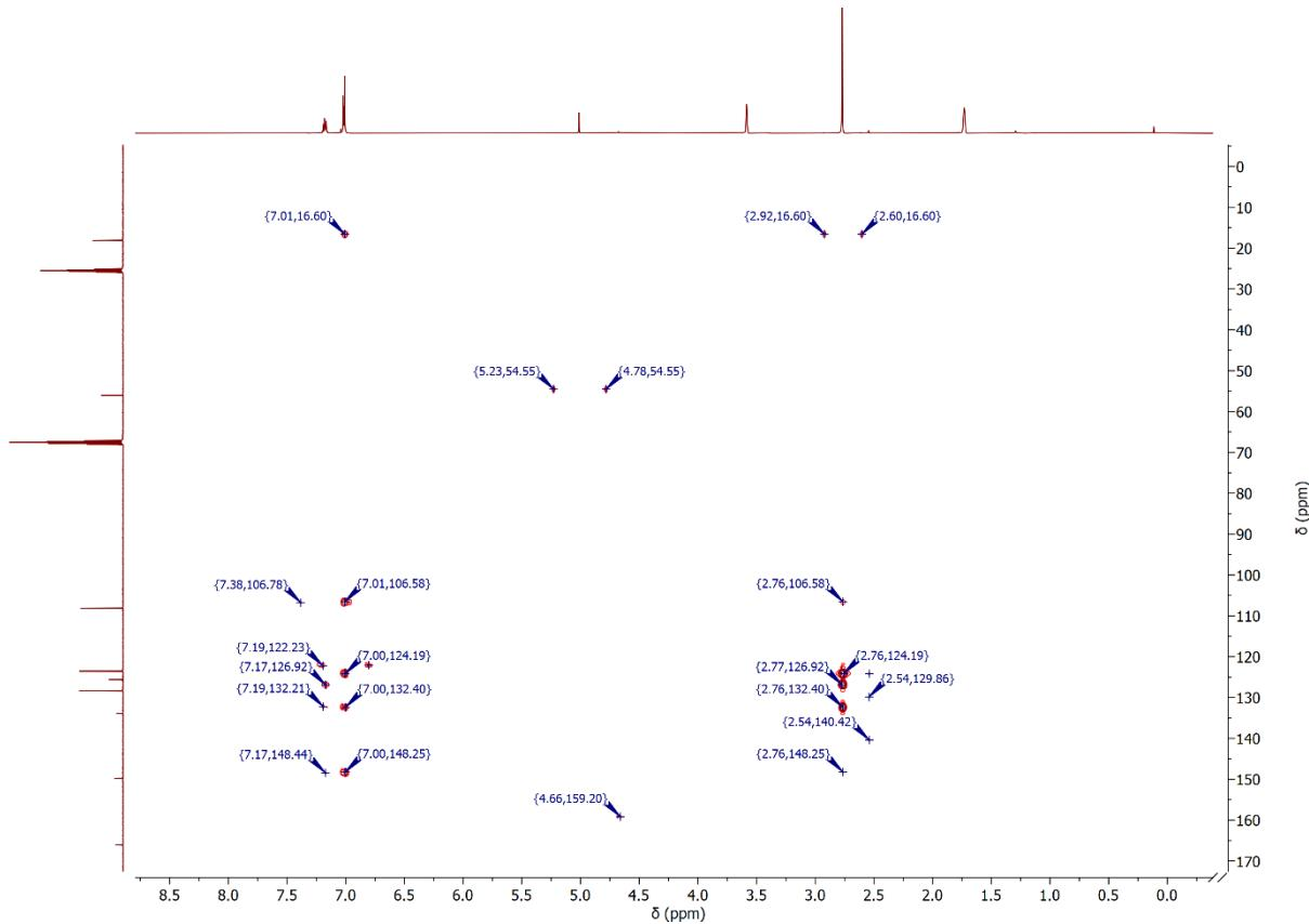
**Figure S4:**  $^1\text{H}$ ,  $^{13}\text{C}$  HMBC NMR spectrum of **1** in  $\text{THF}-d_8$ .
