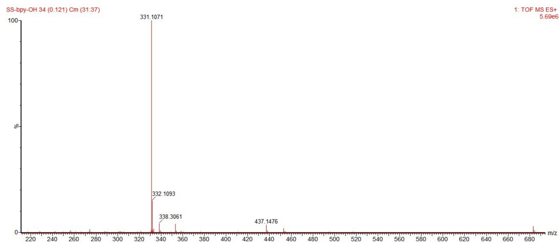
Figure S7. High-resolution mass spectrum of bpy-OH in MeOH
