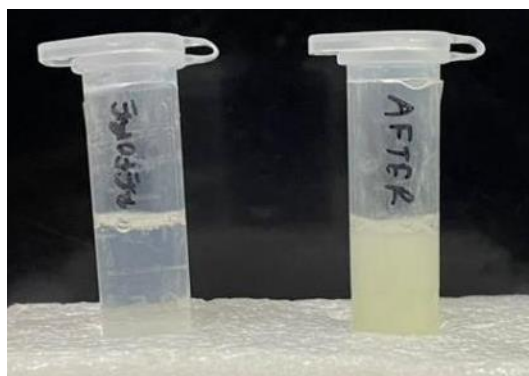
Figure S21: A wet analysis of the electrolyte after 12 h OER CA at 1.6 V CA with Mn-Bi 3 O 4 Br. Left: pre-OER CA electrolyte and right: pale yellow AgBr precipitate (right) obtained by addition of AgNO 3 solution (after acid treatment).
