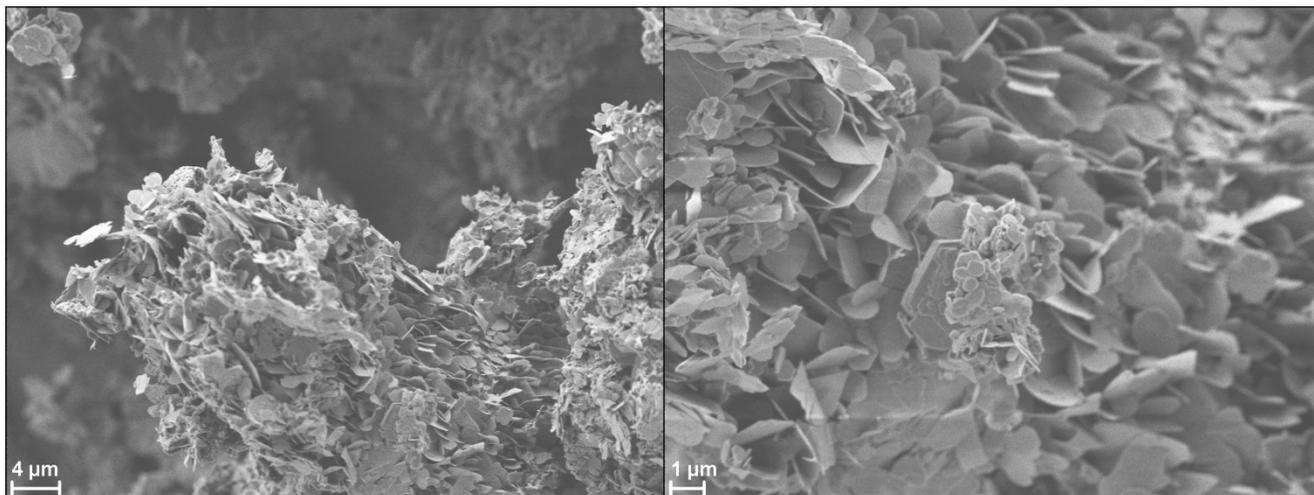
**Fig. S4.2.** SEM images of the product of pyrolysis of  $\text{Li}(\text{BH}_3\text{NH}_2\text{BH}_2\text{NH}_2\text{BH}_3)$  at 1000°C under 1000 bar (HIP) in a steel capsule
