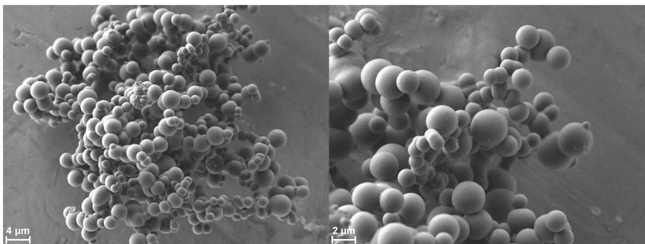
**Fig. S3.2.** SEM images of the product of pyrolysis of ammonia borane at 1000°C under 1000 bar (HIP) in a steel capsule.
