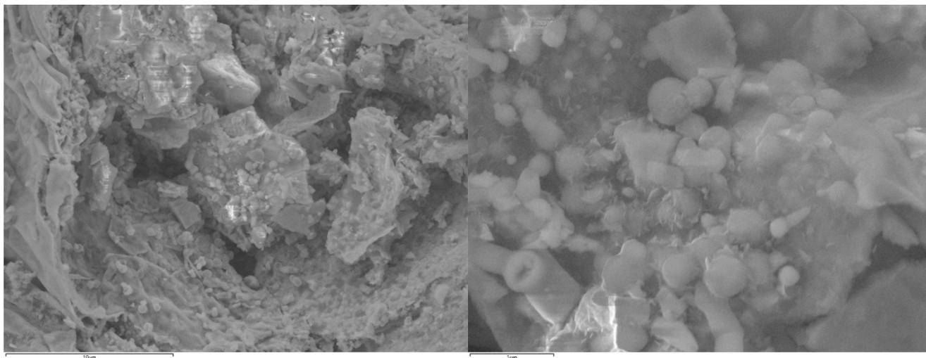
**Fig. S4.1.** SEM images of the product of pyrolysis of  $\text{Li}(\text{BH}_3\text{NH}_2\text{BH}_2\text{NH}_2\text{BH}_3)$  at 850°C in a monel reactor.
