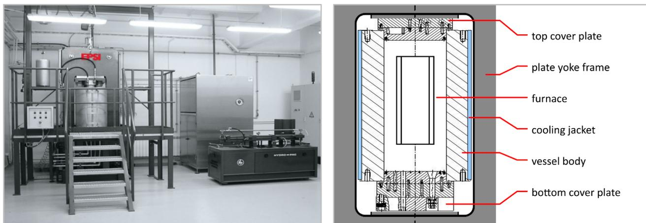
**Fig. S1.** General view of the HIP apparatus at Łukasiewicz-ICIMB (left) and a scheme of the HIP chamber (right).
