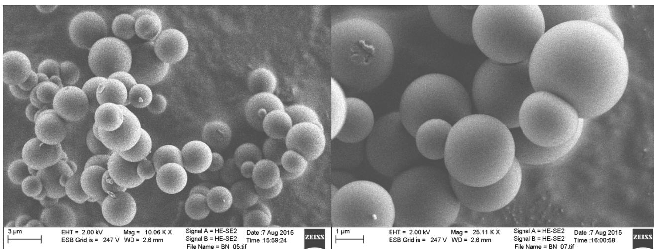
**Fig. S3.1.** SEM images of the product of pyrolysis of ammonia borane at 850°C in a monel reactor.
