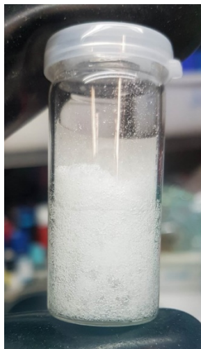
Fig._SI 2 Compound 9 after one week of storage at room temperature under inert conditions. The formation of a foam like, brittle solid was observed.
