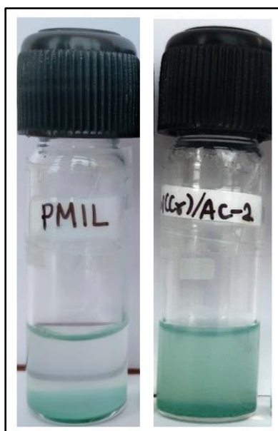
Fig. S11 Dispersion of samples in methanol (a) as-synthesized PMIL after 15 minutes and (b) MIL-101(Cr)/AC-2 after 4 days.
