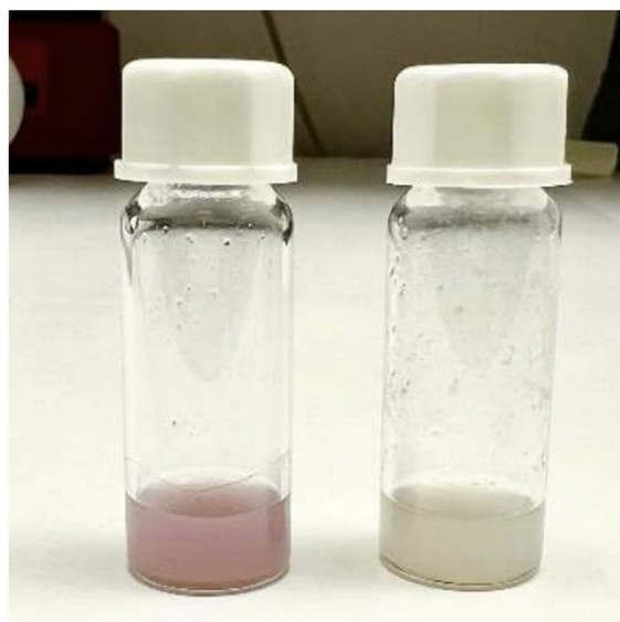
Figure S8. SCO@SiO 2 -1 freshly redispersed in EtOH (pink solution), and after heated to 60°C, and cool down to room temperature (white solution).
