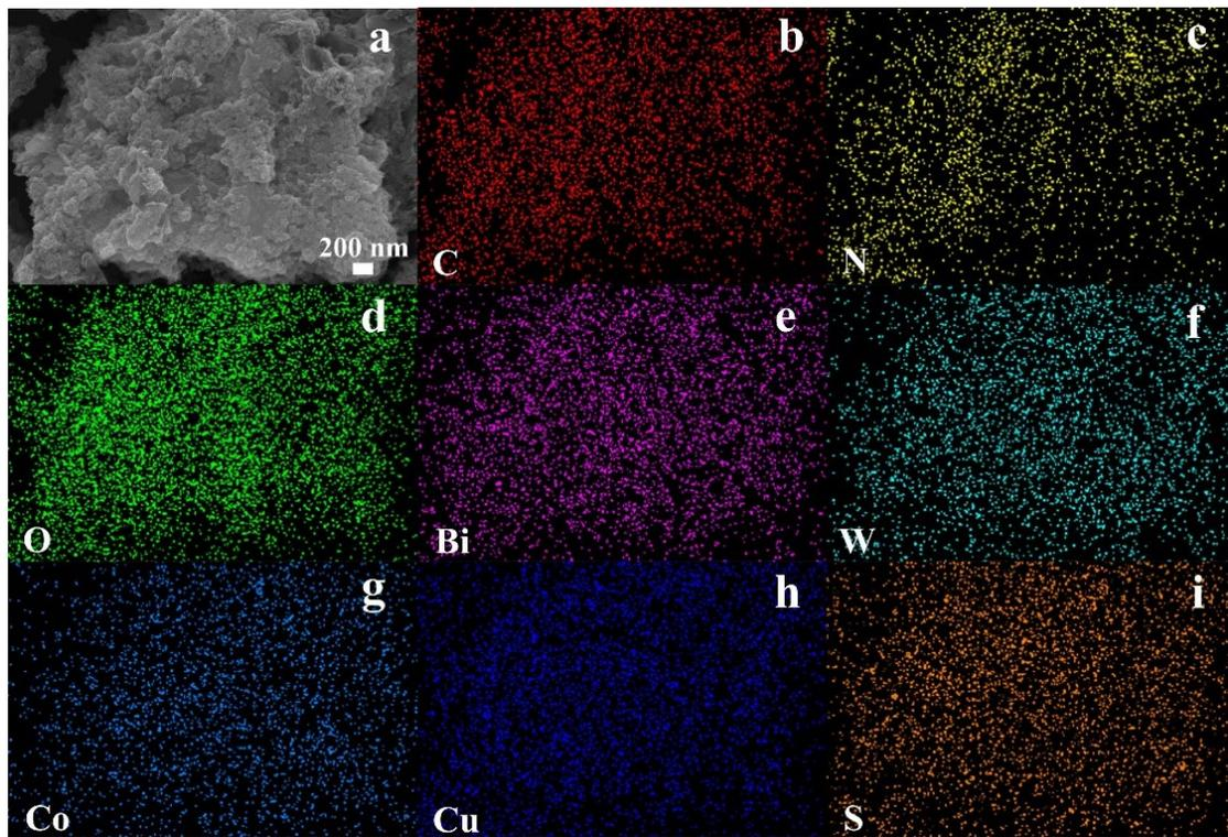
**Fig. S2.** The SEM image of BiWCo/CuS/PGCN (a) and the elemental mapping images of C (b), N
