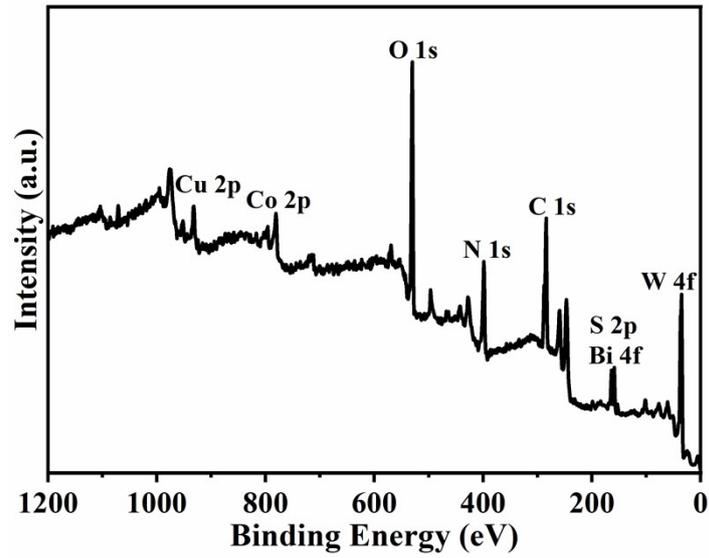
**Fig. S1.** XPS survey spectra of BiWCo/CuS/PGCN.
