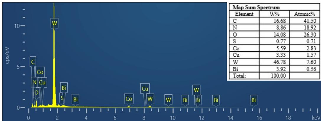
Fig. S3. The EDS spectrum of BiWCo/CuS/PGCN.
