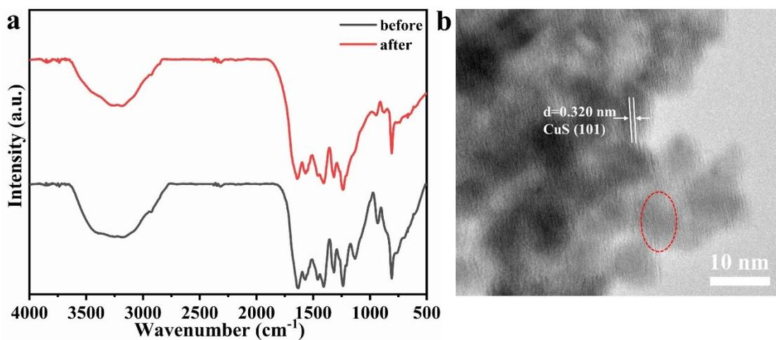
Fig. S4. The FT-IR spectra and the TEM image of BiWCo/CuS/PGCN after 30 h illumination.
