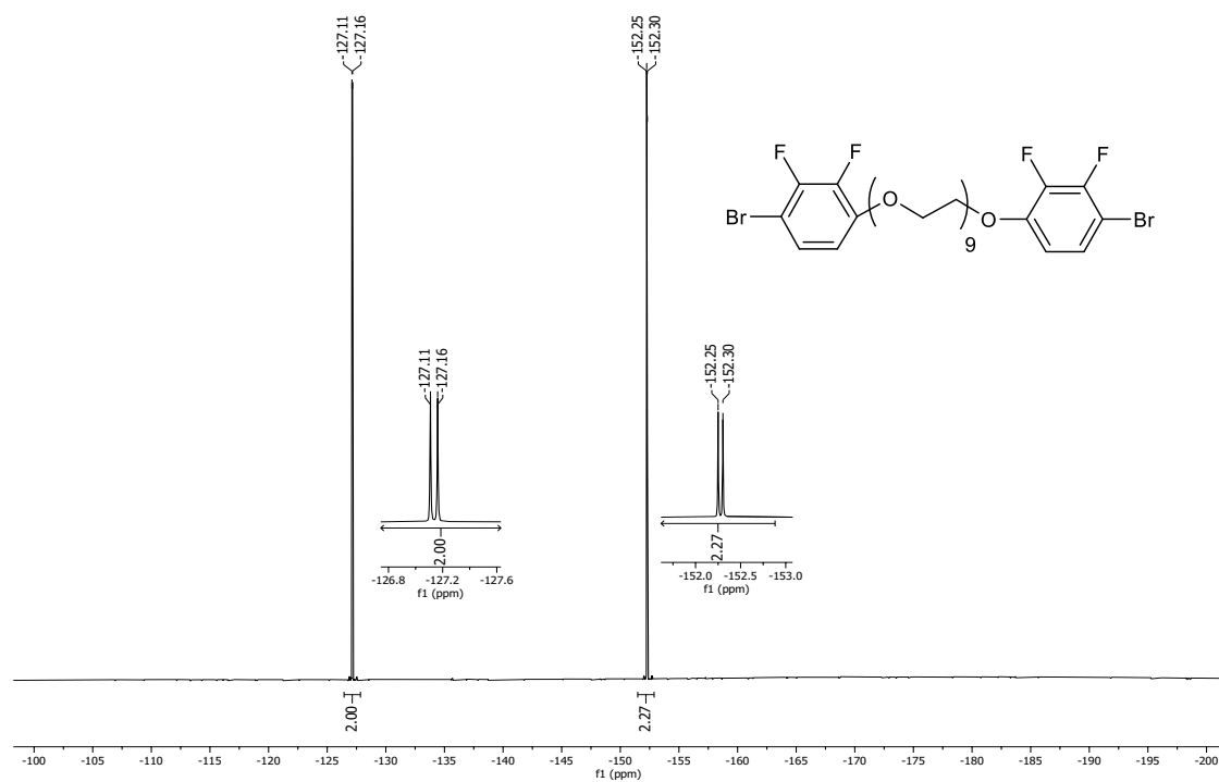
Figure S25. 19 F{ 1 H} NMR spectrum of 5[9] (CDCl 3 , 376 MHz).
