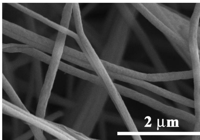
**Fig. S4.** SEM analysis was performed after 10 000 GCD cycles of CNF/Eu<sub>2</sub>O<sub>3</sub>-1.
