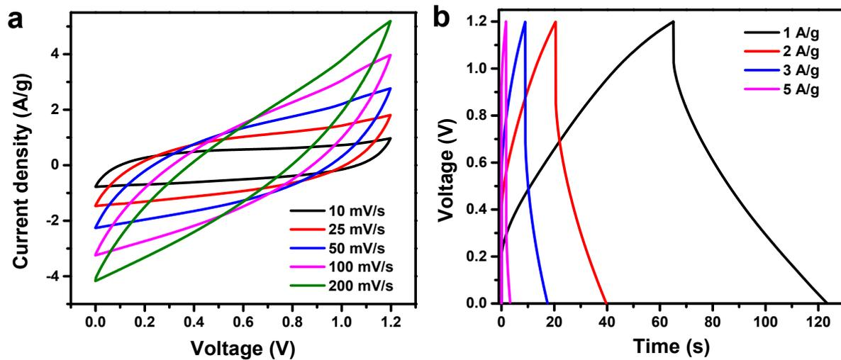
**Fig. S3.** (a) CV curves at different scan rates and (b) GCD curves at different current densities of the CNF/Eu<sub>2</sub>O<sub>3</sub>-2.
