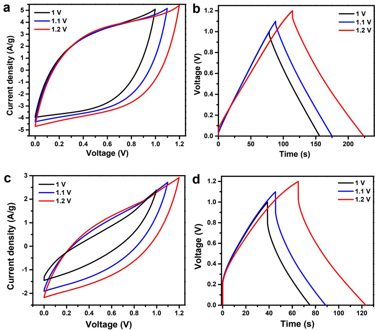
**Fig. S2.** (a, c) CV curves at 50 mV/s and (b, d) GCD curves at 1 A/g of the CNF/Eu<sub>2</sub>O<sub>3</sub>-1 and CNF/Eu<sub>2</sub>O<sub>3</sub>-2 for different voltages, respectively,
