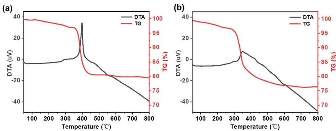
**Figure S4.** TG-DSC curves figure of the compounds **1** and **2**
