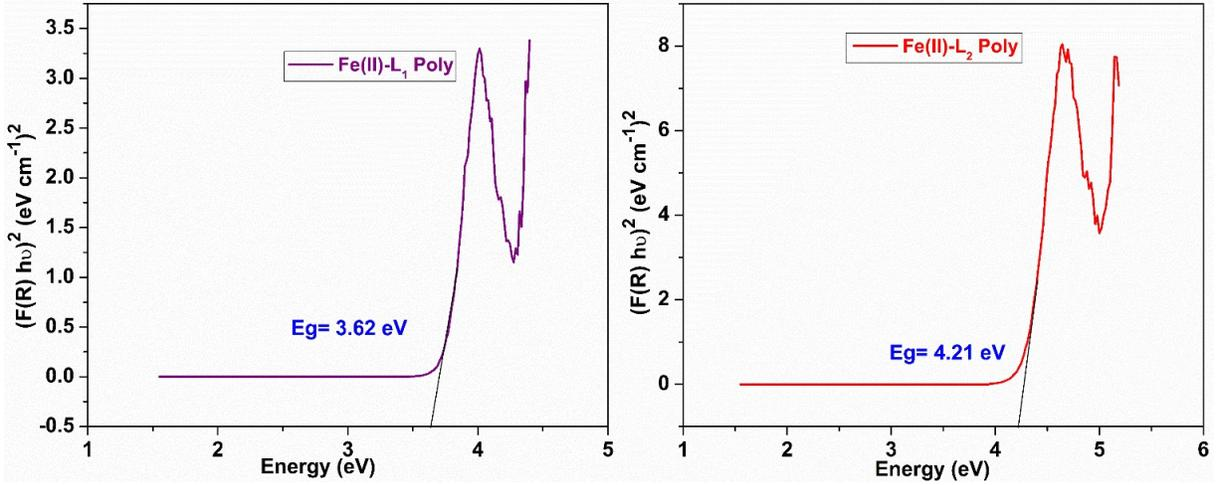
Figure .S-17. DRS of Fe(II)-L<sub>1</sub> poly and Fe(II)-L<sub>2</sub> poly
