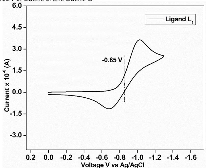
Figure .S-10. Cyclic Voltammogram of Ligand L<sub>1</sub> in dichloromethane containing 0.1 M TBAP at 100mV/s with Glassy Carbon working electrode and Ag/AgCl reference electrode
