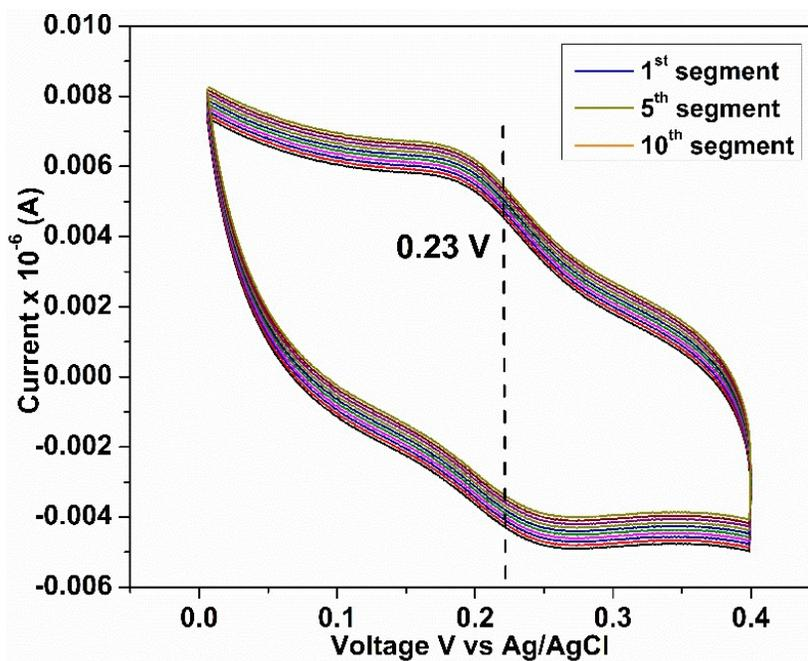
Figure .S-15. 10 segment oxidation Cyclic Voltammogram of Fe(II)-L<sub>2</sub> poly
