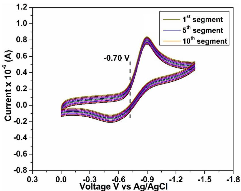
Figure .S-12. 10 segment reduction Cyclic Voltammogram of Fe(II)- $L_1$  poly
