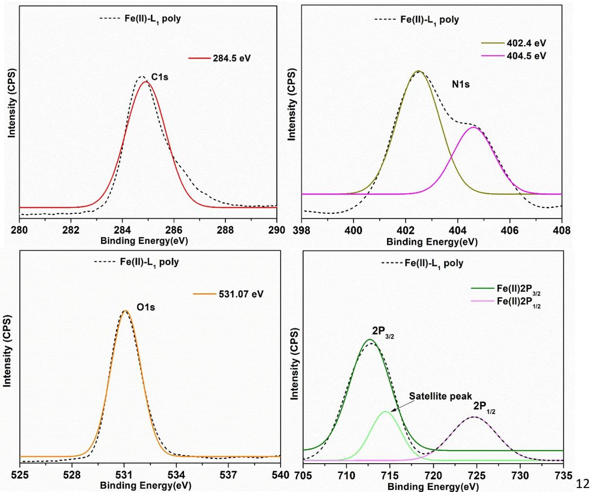
Figure .S-18. XPS of Fe(II)-L<sub>1</sub> poly of a) Carbon b) Nitrogen c) Oxygen and d) Iron element
