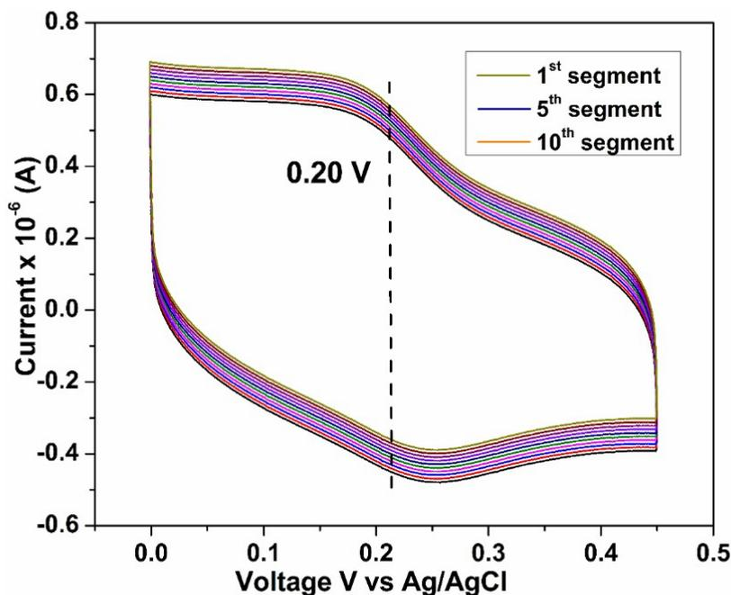
Figure .S-13. 10 segment oxidation Cyclic Voltammogram of Fe(II)- $L_1$  poly
