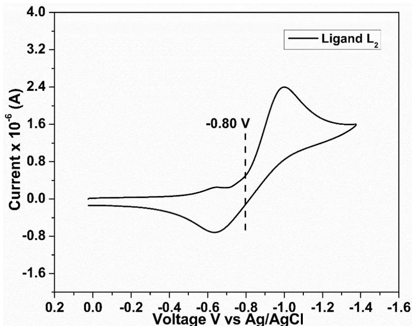
Figure .S-11. Cyclic Voltammogram of ligand  $L_2$  in dichloromethane containing 0.1 M TBAP at 100mV/s with Glassy Carbon working electrode and Ag/AgCl reference electrode
