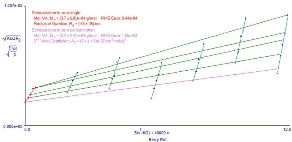
Figure .S-6. Berry Plot of Fe (II)-L<sub>1</sub> poly in batch mode (THF solution)
