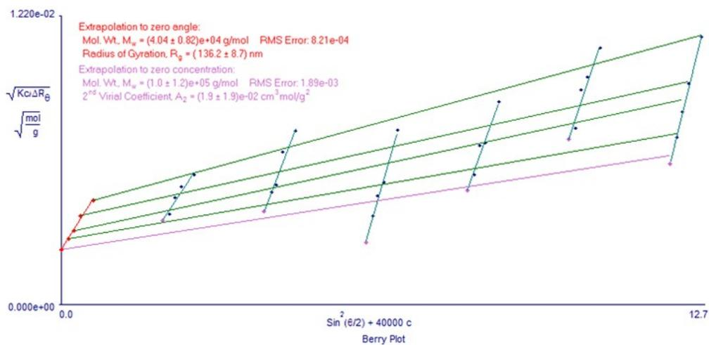
Figure .S-8. Berry Plot of Fe (II)-L<sub>2</sub> poly in batch mode with a solution prepared in THF
