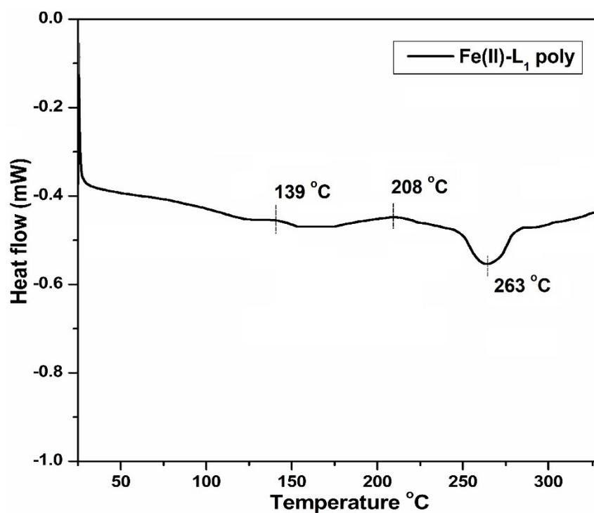
Figure .S-7. DSC Thermogram of Fe(II)-L<sub>1</sub> poly
