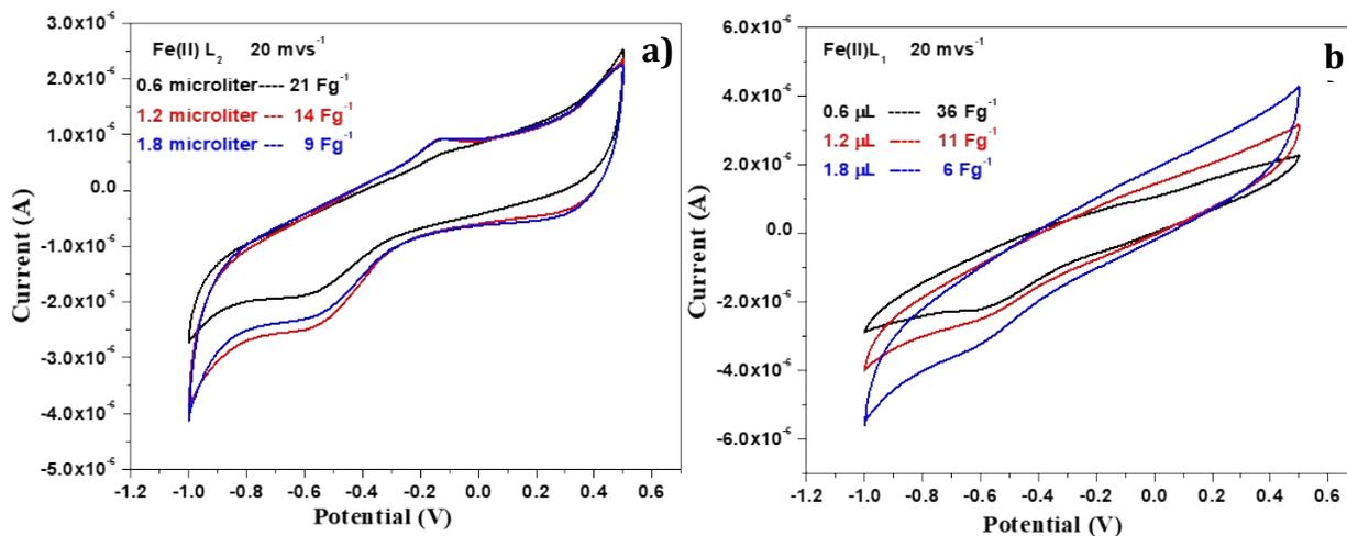
Figure .S-21. Effect of mass loading and scan rate on capacitance value of Fe(II)-L<sub>1</sub> poly and Fe(II)-L<sub>2</sub> poly
