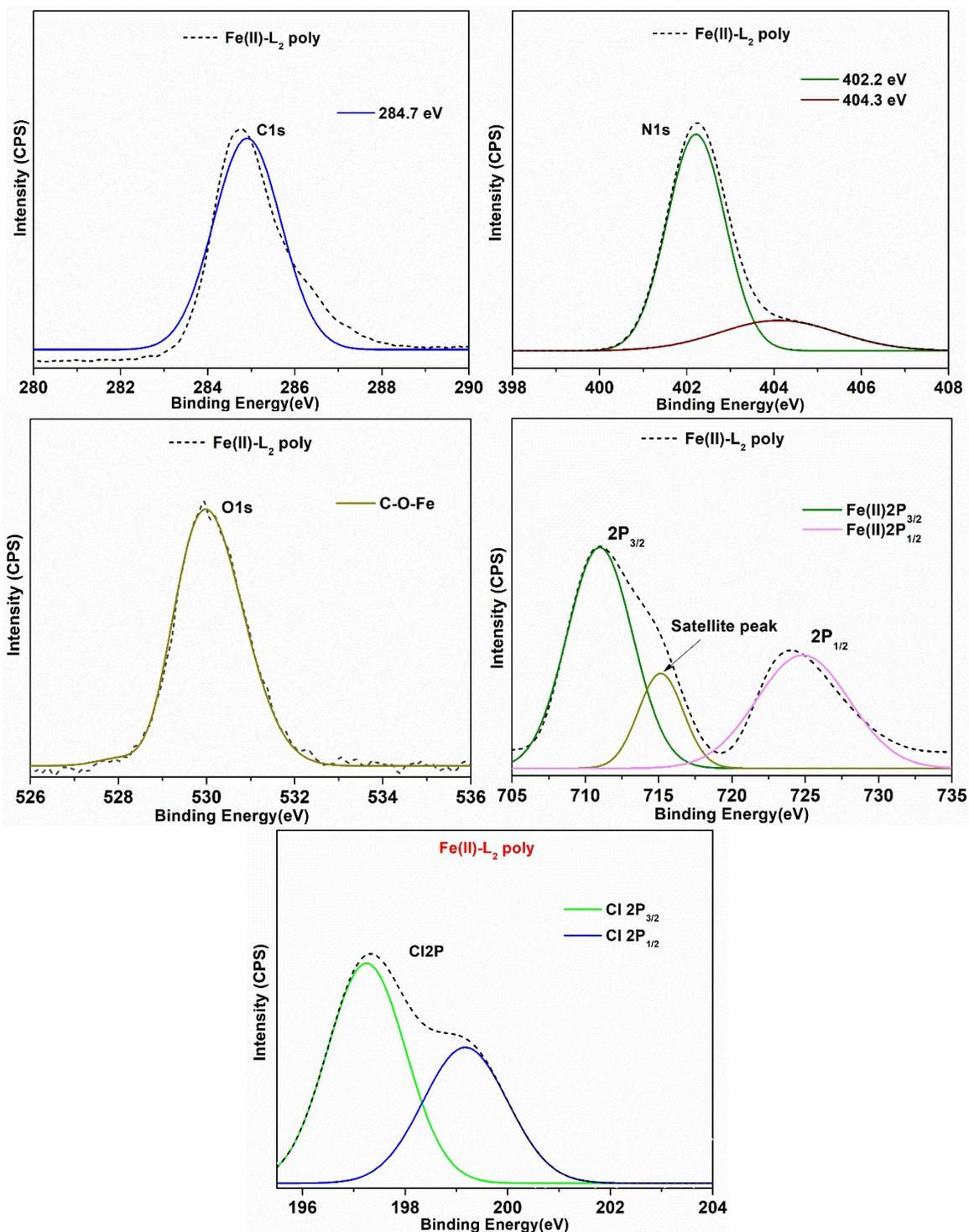
Figure .S-19. XPS of Fe(II)-L<sub>2</sub> poly of a) Carbon b) Nitrogen c) Oxygen d) Iron and e) Chlorine element
