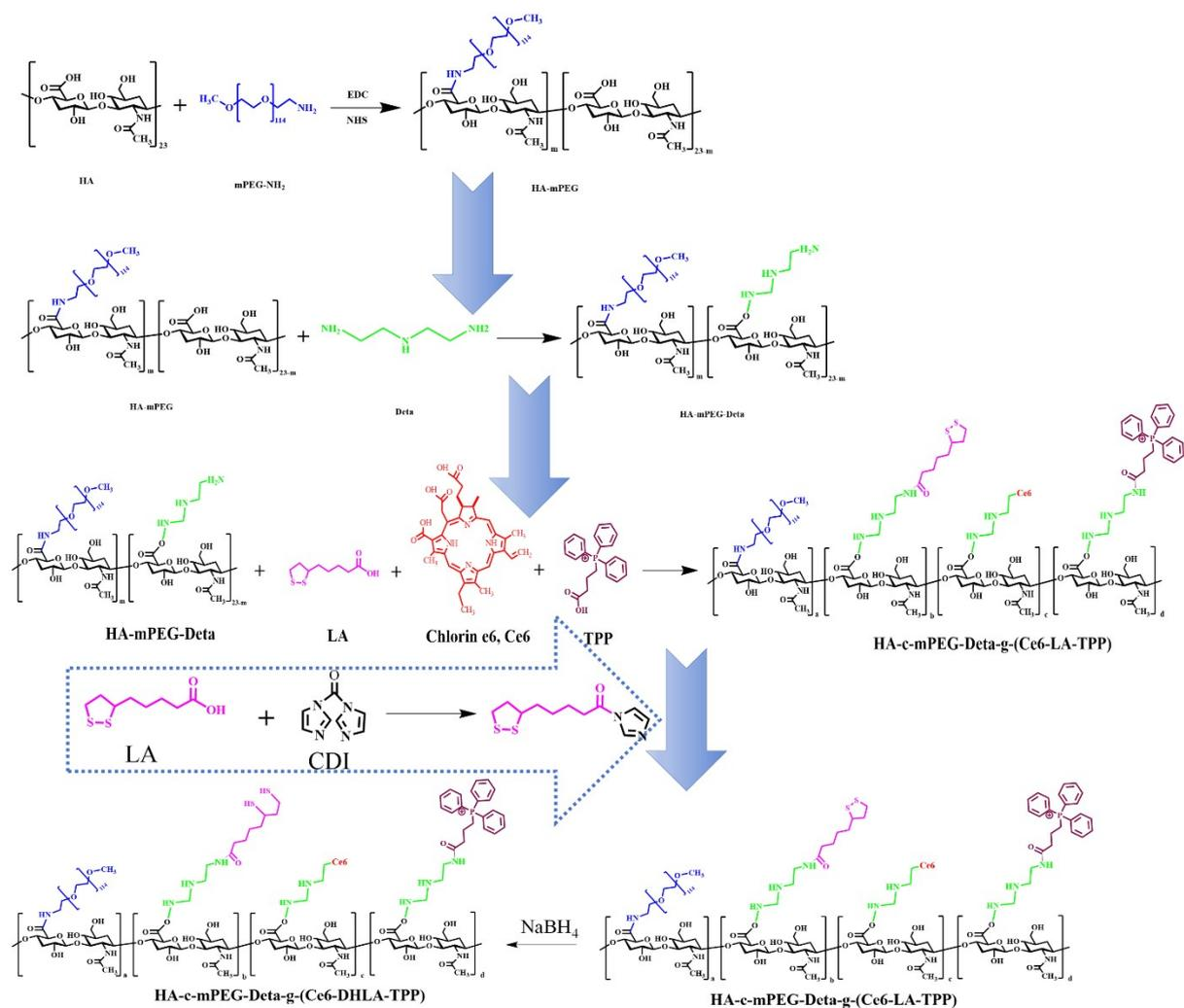
**Scheme S2.** The synthesis route of HA-c-mPEG-Deta-g-(Ce6-DHLA-TPP) polymer ligand.
