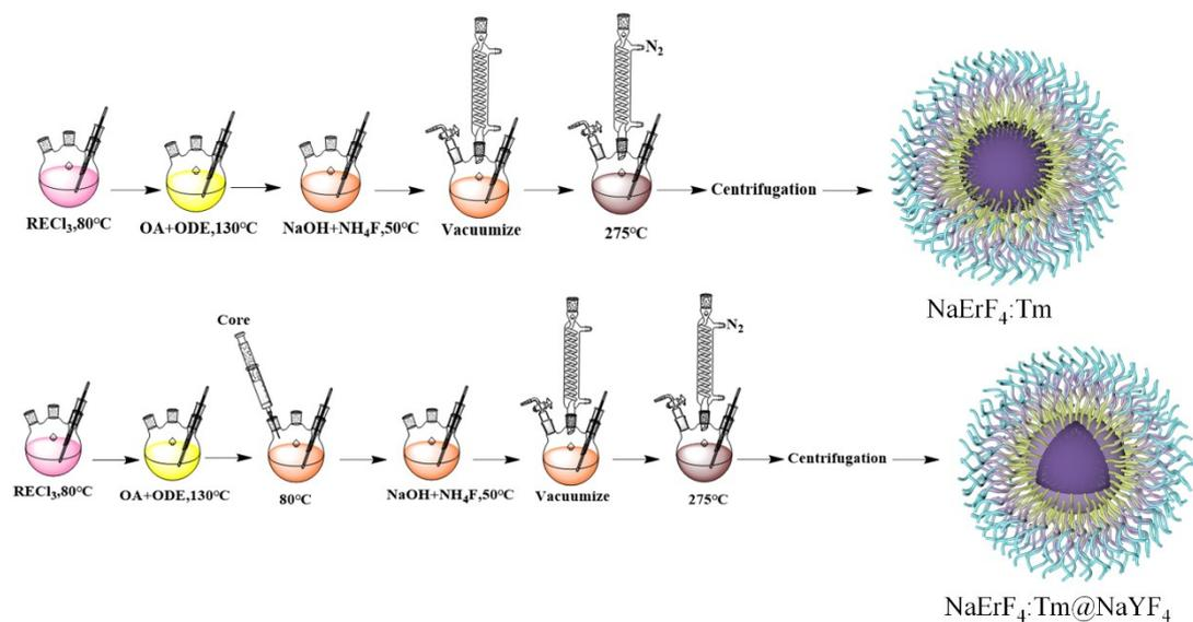
**Scheme S1.** Synthesis process of NaErF<sub>4</sub>:Tm core UCNPs and NaErF<sub>4</sub>:Tm@NaYF<sub>4</sub> core-shell UCNPs using typical hydrothermal methods.
