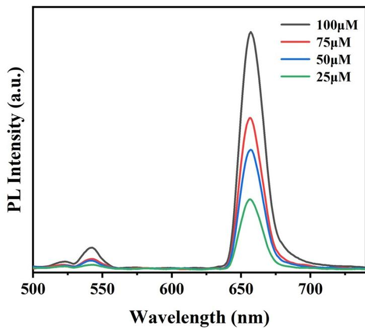
**Figure S5.** PL emission spectrum of CMPN complexes under different Ce6 loading concentrations.
