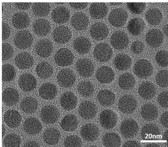
**Figure S1.** TEM images of NaErF<sub>4</sub>:Tm core UCNPs.
