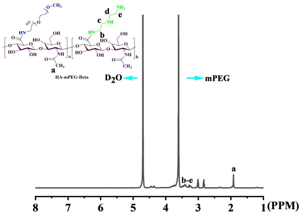
**Figure S2.**  $^1\text{H}$  NMR spectrum (500 MHz) of HA-mPEG-Deta ligand polymer in  $\text{D}_2\text{O}$ .
