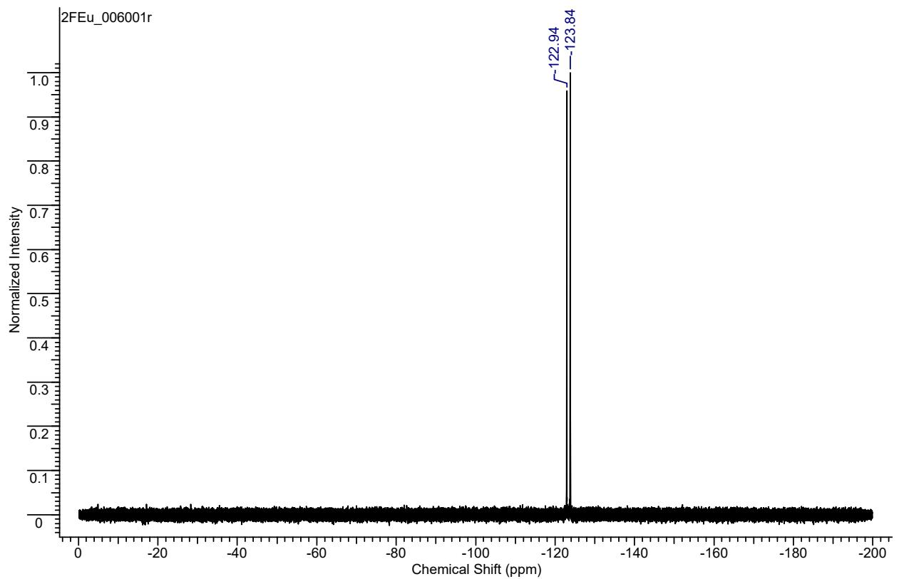
**Fig 23**  $^{19}\text{F}$  Spectrum of  $\text{Eu}_2\text{F}(\text{NO}_3)_3$  in acetonitrile
