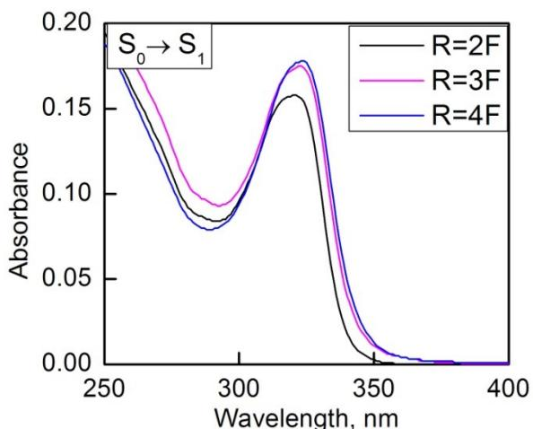
**Fig 30** Absorption spectra of europium complexes with different fluoride-substituted ligands in acetonitrile, C=1·10<sup>-5</sup> mol/l.
