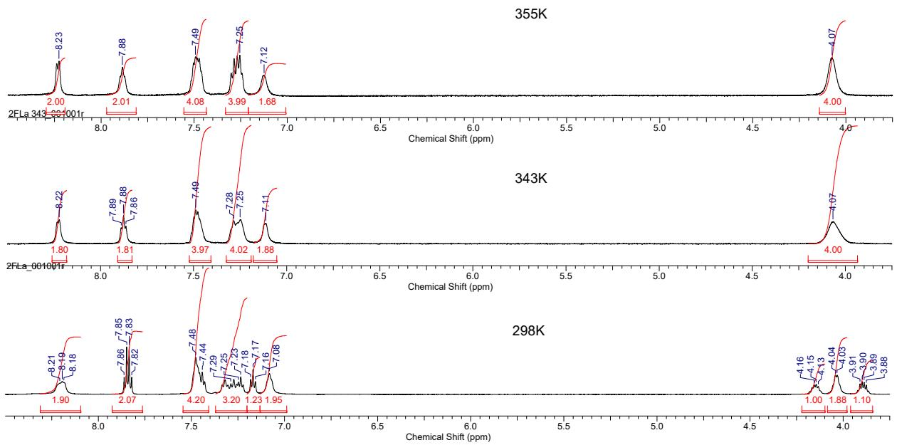
**Fig 1** The temperature-dependent coalescence of the fluoroaromatic and methylene-groups protons in  $\text{La}_2\text{F}(\text{NO}_3)_3$  in acetonitrile
