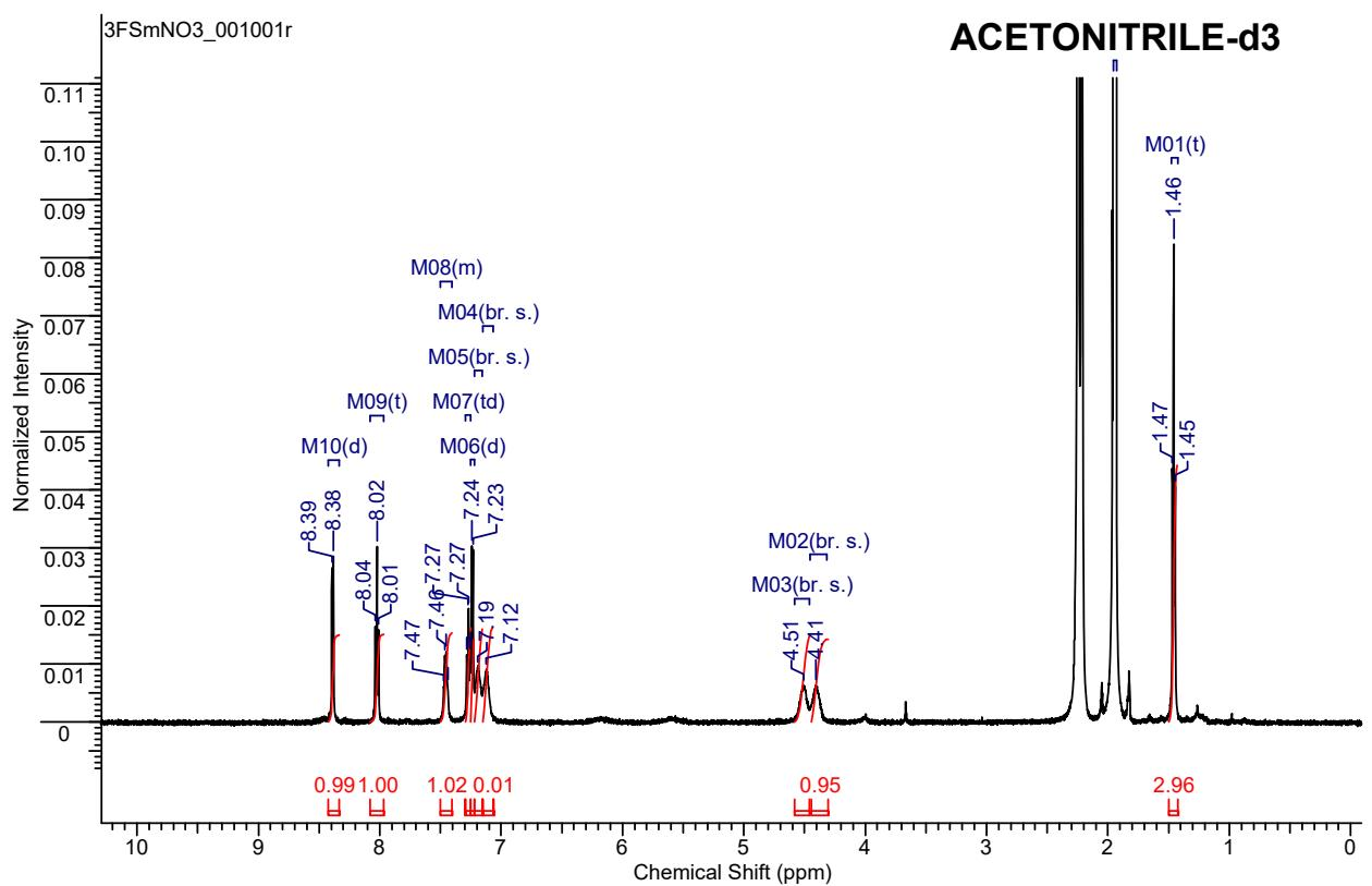
Fig 7  $^1\text{H}$  Spectrum of  $\text{Sm}_3\text{F}(\text{NO}_3)_3$  in acetonitrile
