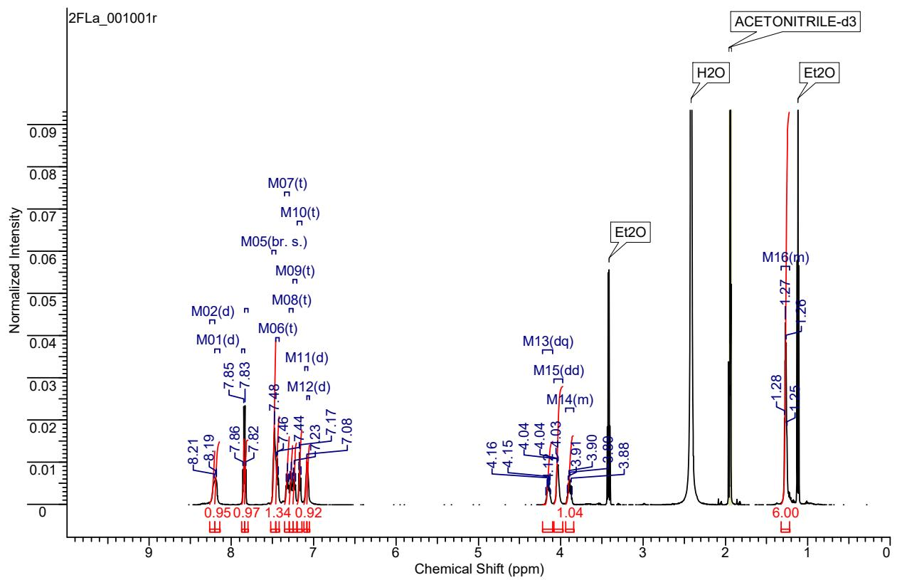
Fig 27 1H Spectrum of La<sub>2</sub>F(No<sub>3</sub>)<sub>3</sub> in acetonitrile
