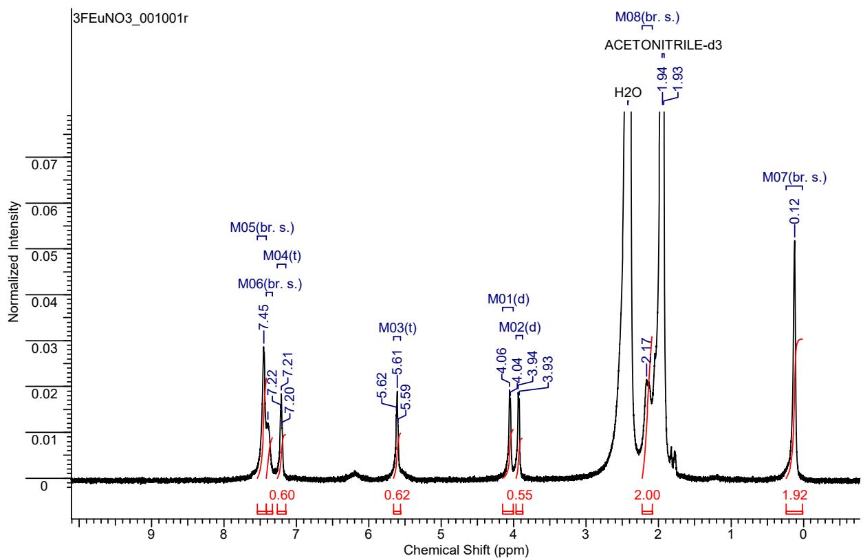
Fig 4 1H Spectrum of Eu3F(No<sub>3</sub>)<sub>3</sub> in acetonitrile
