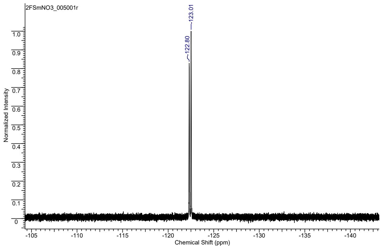
Fig 19 <sup>19</sup>F Spectrum of Sm<sub>2</sub>F(No<sub>3</sub>)<sub>3</sub> in acetonitrile
