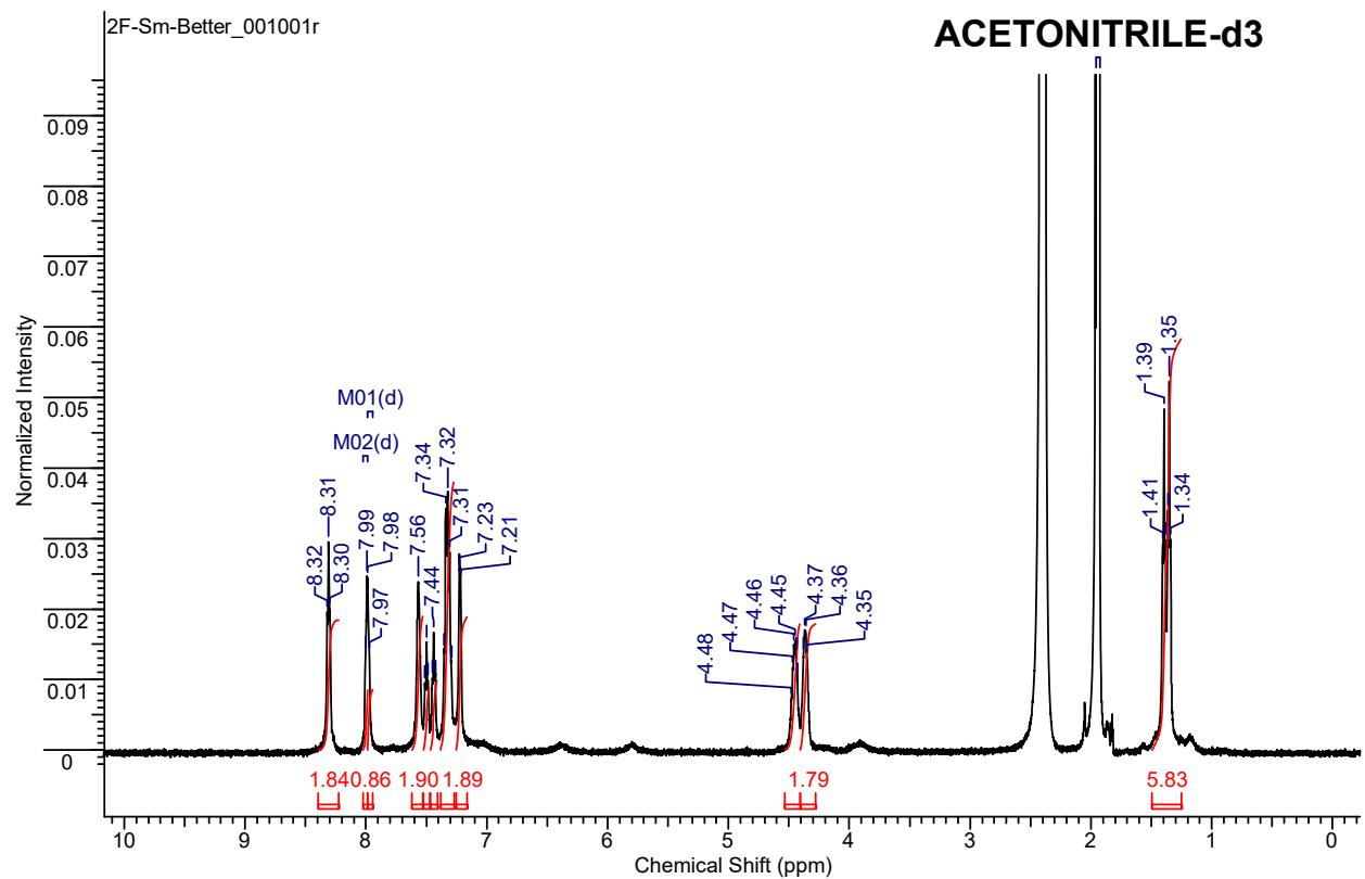
Fig 16 1H Spectrum of Sm2F(NO<sub>3</sub>)<sub>3</sub> in acetonitrile
