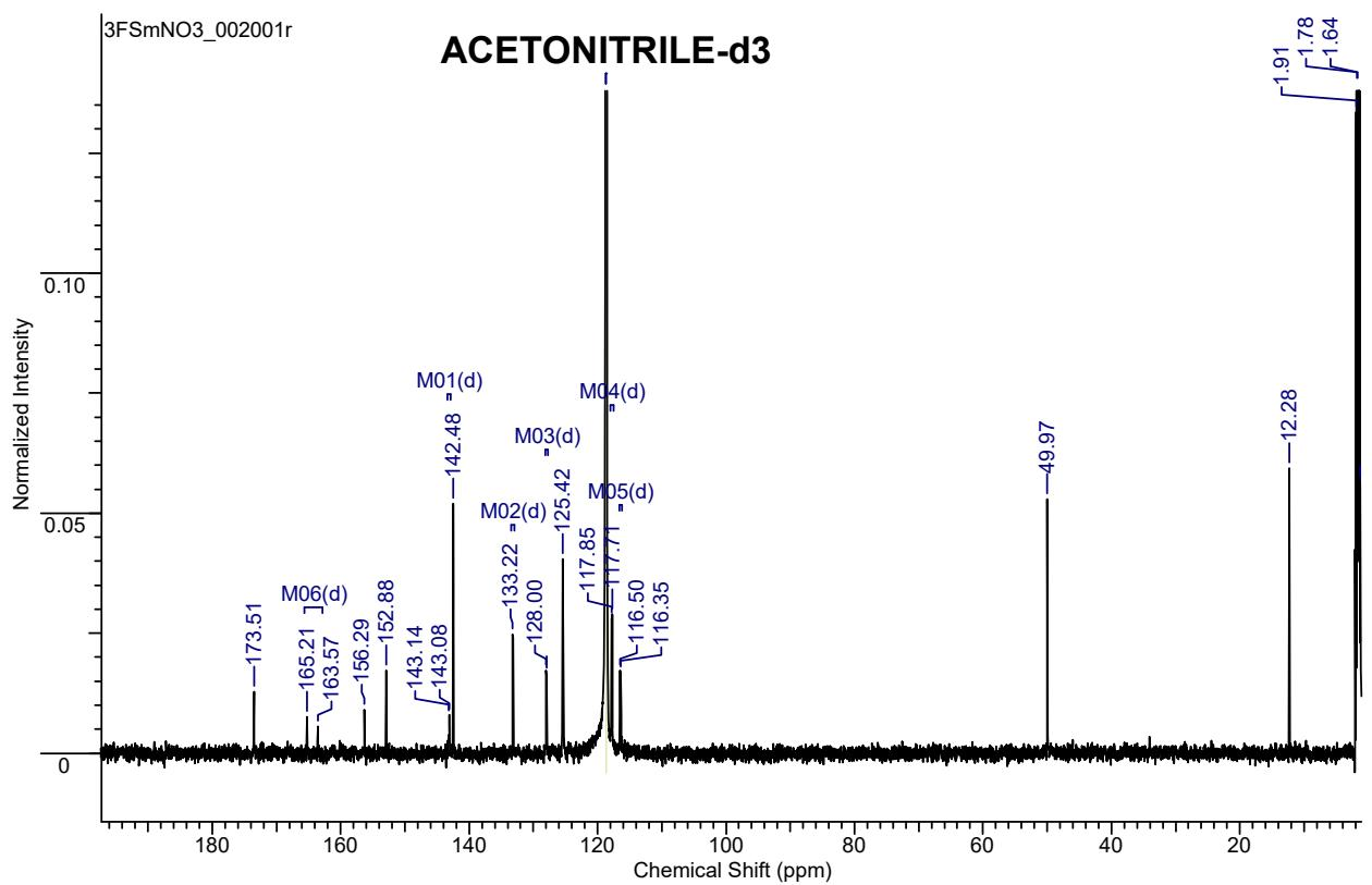
Fig 8  $^{13}\text{C}$  Spectrum of  $\text{Sm}_3\text{F}(\text{NO}_3)_3$  in acetonitrile
