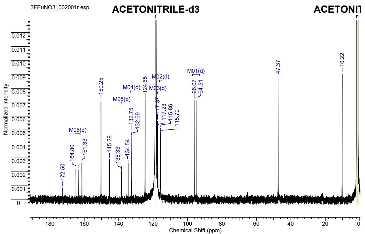
Fig 5 <sup>13</sup>C Spectrum of Eu<sub>3</sub>F(NO<sub>3</sub>)<sub>3</sub> in acetonitrile
