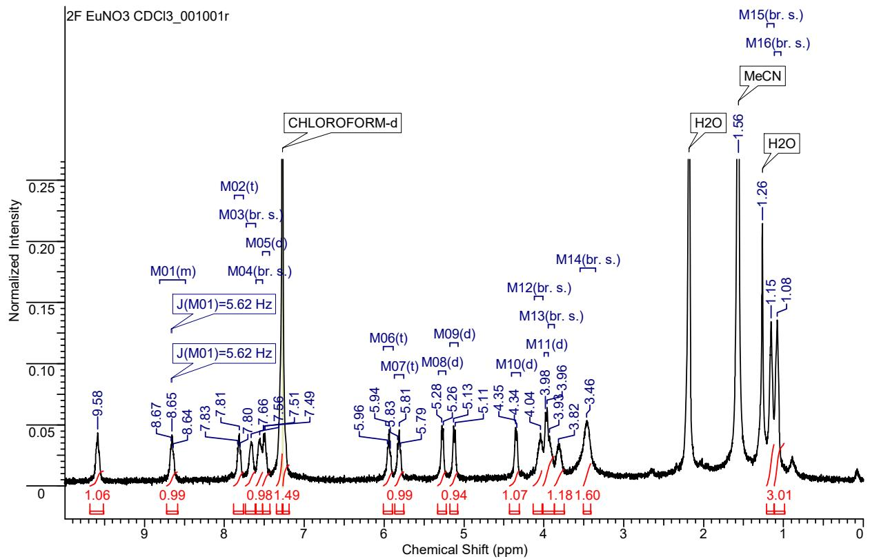
**Fig 22**  $^1\text{H}$  Spectrum of Eu $^{2+}$ F(NO<sub>3</sub>)<sub>3</sub> in acetonitrile
