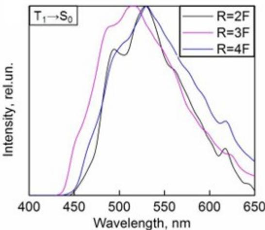
**Fig 31 Normalized phosphorescence spectrum of gadolinium complexes with different fluoride-substituted ligands at 77 K.**
