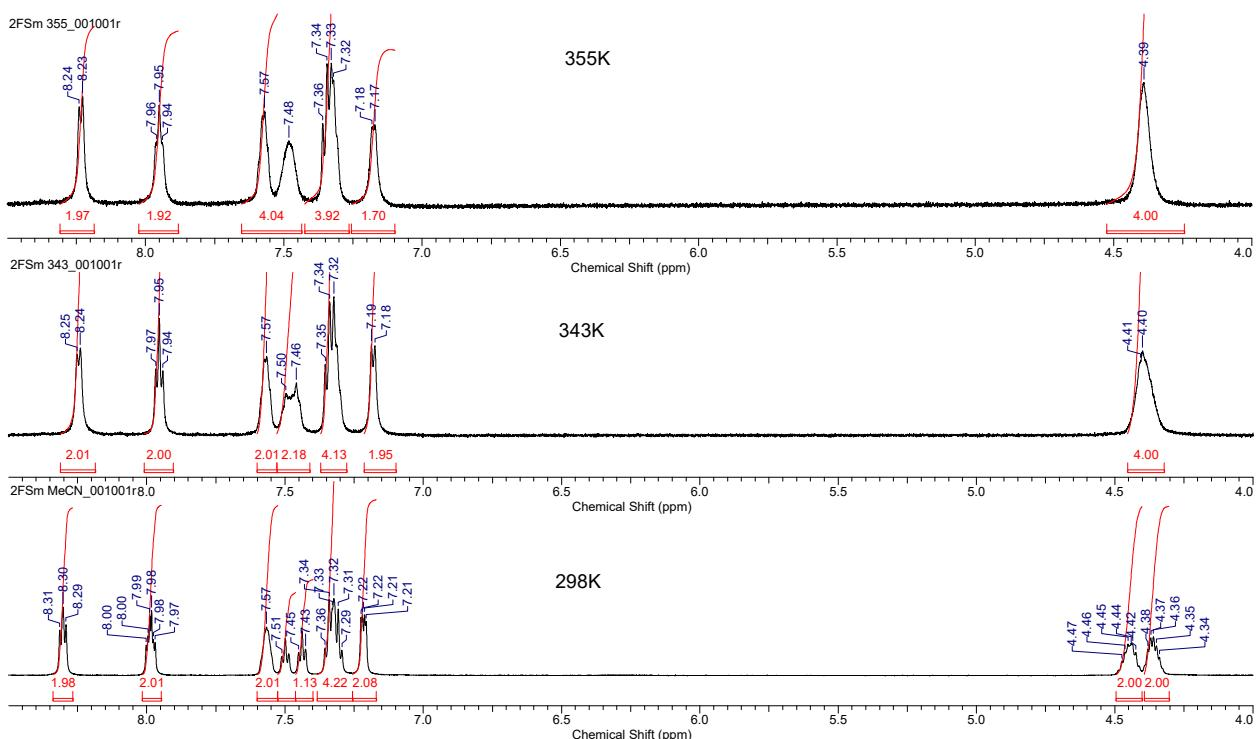
**Fig 2** The temperature-dependent coalescence of the fluoroaromatic and methylene-groups protons in  $\text{Sm}_2\text{F}(\text{NO}_3)_3$  in acetonitrile
