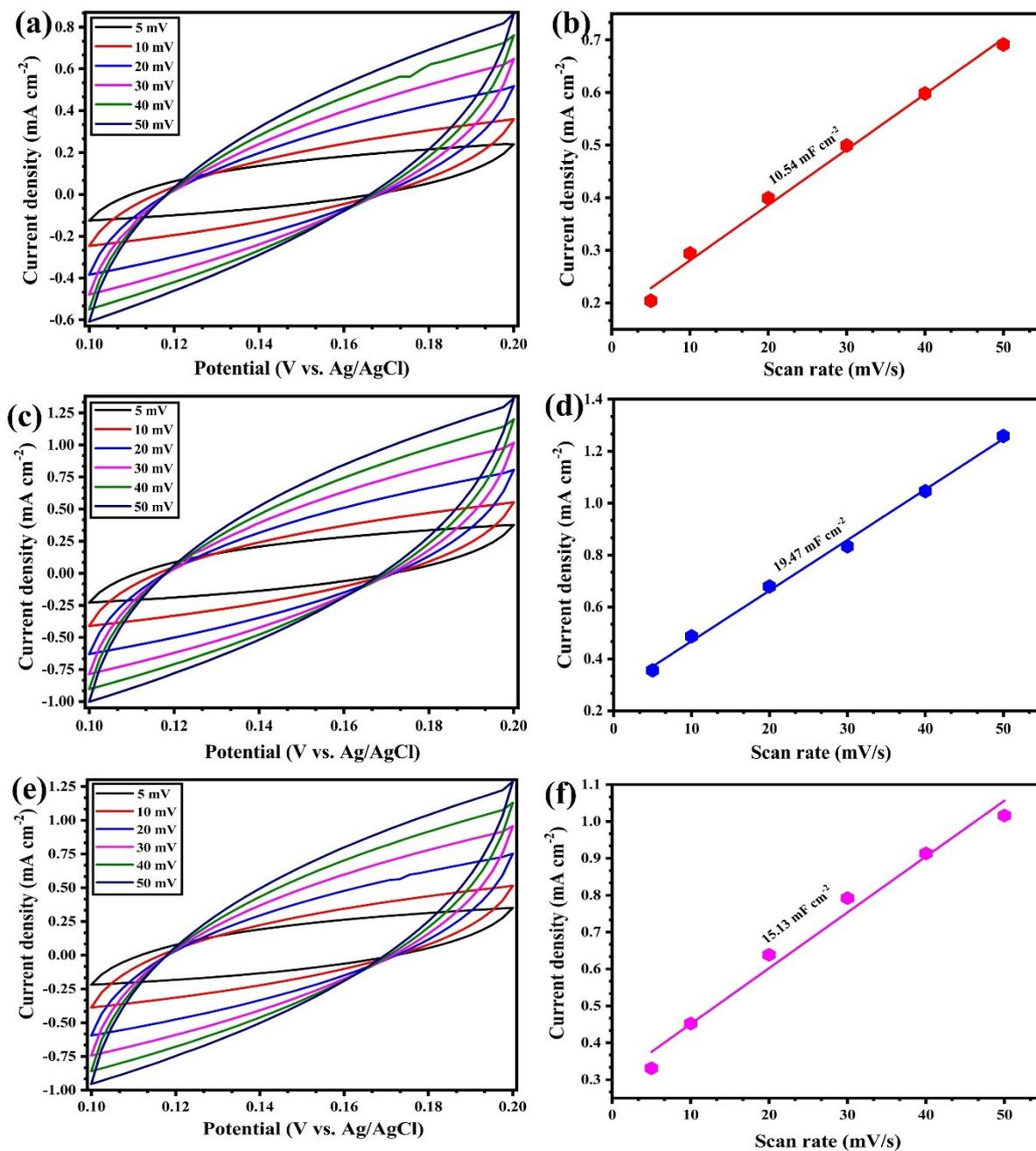
**Fig. S2** CV profile of (a) Zr-MOF; (c) Se-ZrO<sub>2</sub>@NC-300 and (e) Se-ZrO<sub>2</sub>@NC-400 at non-faradic region at different scan rates (5 to 50 mV/s) in 1 M KOH, plot of current density as a function of scan rate of (b) Zr-MOF; (d) Se-ZrO<sub>2</sub>@NC-300 and (f) Se-ZrO<sub>2</sub>@NC-400.
