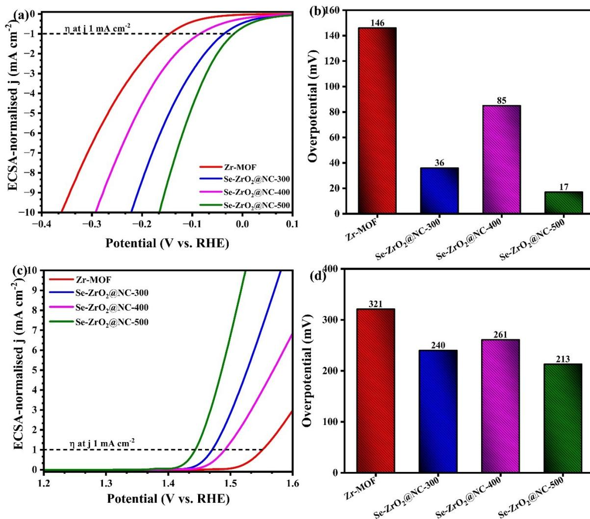
**Fig. S5** ECSA normalized LSV curve and corresponding overpotential at 1 mA cm<sup>-2</sup> current density of Zr-MOF, Se-ZrO<sub>2</sub>@NC-300, Se-ZrO<sub>2</sub>@NC-400 and Se-ZrO<sub>2</sub>@NC-500 for (a, b) HER and (c, d) OER activity.
