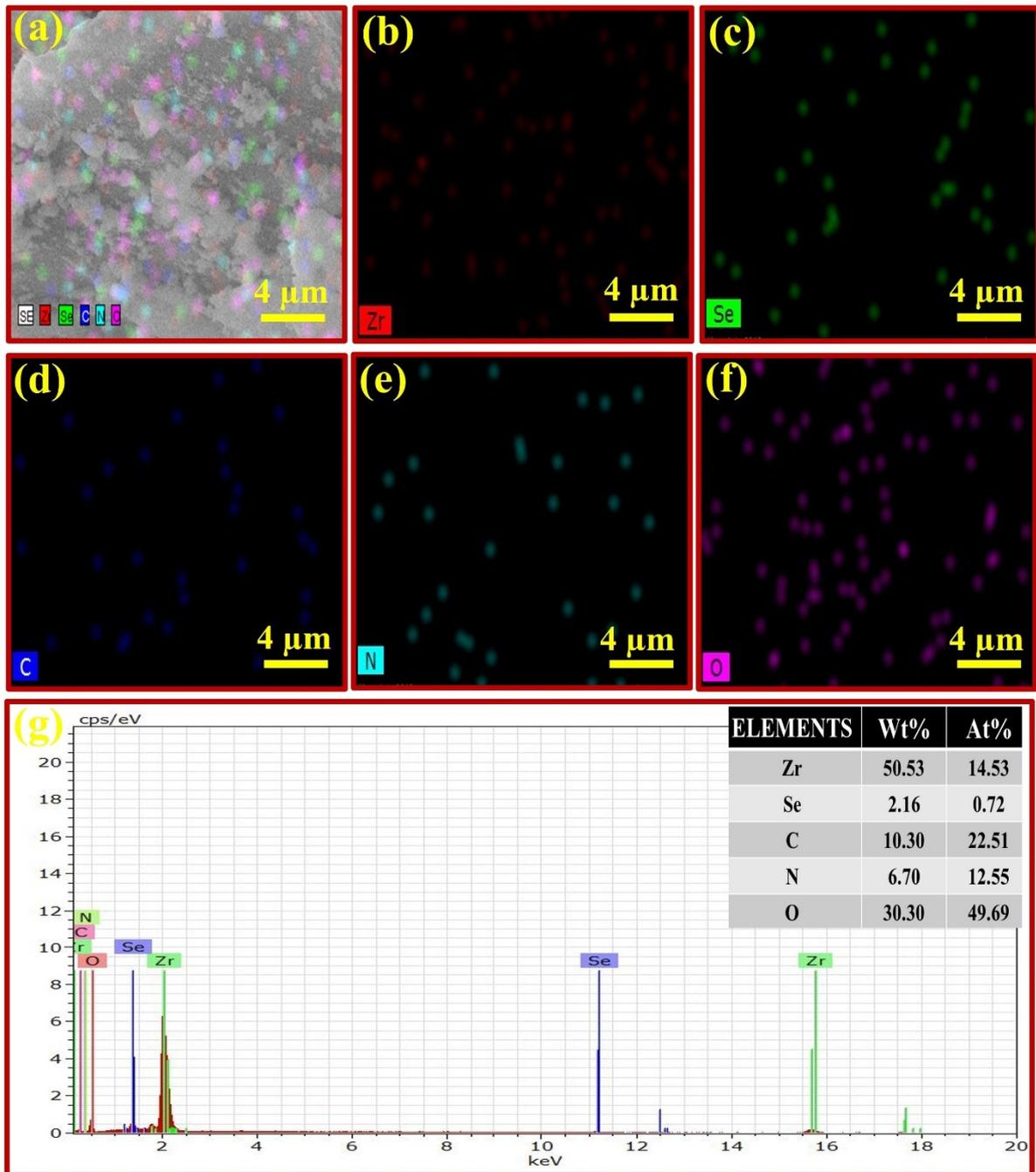
**Fig. S1** (a) Elemental mapping of Se-ZrO<sub>2</sub>@NC-500 composite; (b-f) individual elemental mapping of Zr, Se, C, N and O respectively and (g) elemental composition.
