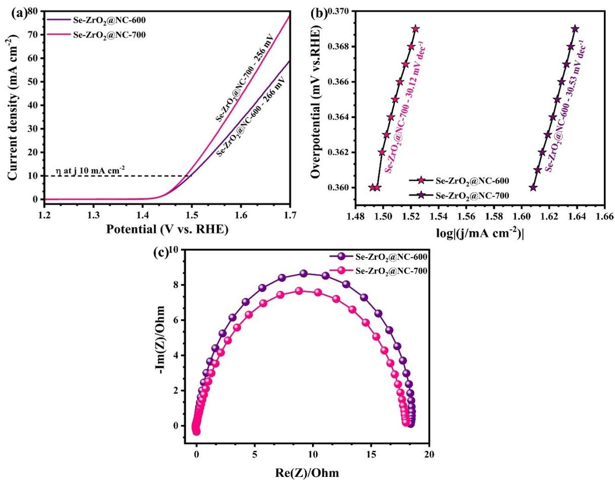
**Fig. S4** OER activity of Se-ZrO<sub>2</sub>@NC-600 and Se-ZrO<sub>2</sub>@NC-700 loaded electrode in 1.0 M KOH. (a) LSV polarization curves at 2 mV/s; (b) the corresponding Tafel plot and (c) Nyquist plots.
