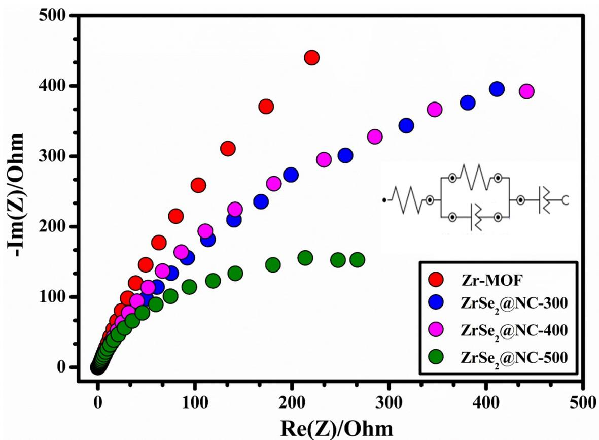
**Fig. S7** Nyquist plots for overall water splitting reactions of Zr-MOF, Se-ZrO<sub>2</sub>@NC-300, Se-ZrO<sub>2</sub>@NC-400 and Se-ZrO<sub>2</sub>@NC-500 in 1 M KOH. Inset shows the equivalent circuit fitted for loaded electrode.
