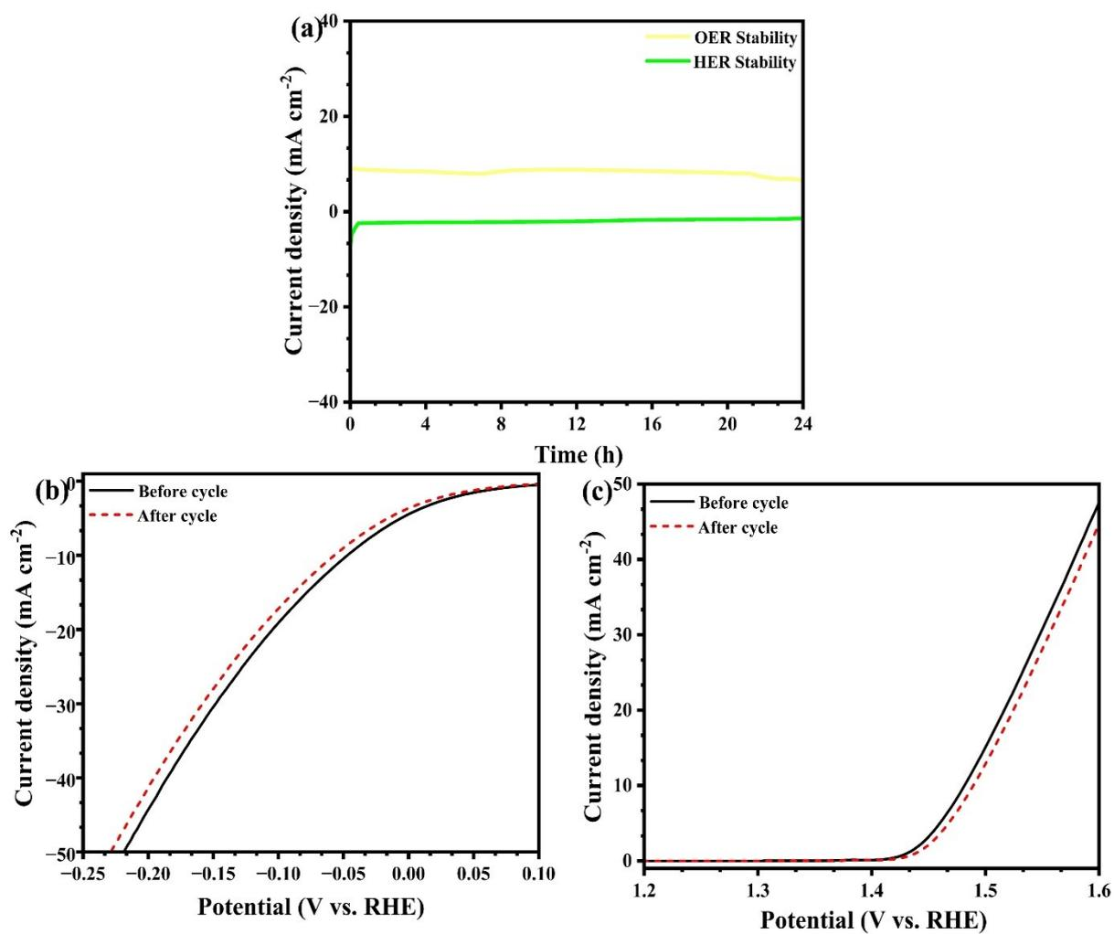
**Fig. S6** (a) Chronoamperometric  $i-t$  curves for Se-ZrO<sub>2</sub>@NC-500 loaded electrode showing HER and OER stability for 24 h; LSV curves for before and after chronoamperometric studies (b) HER and (c) OER activity.
