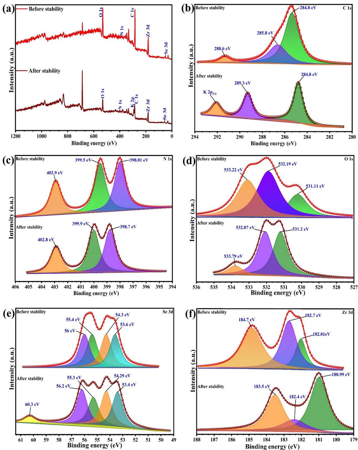
**Fig. S8** (a) XPS survey spectra studied before and after stability for Se-ZrO<sub>2</sub>@NC-500 composite and (b–f) the corresponding high-resolution XPS of C 1s, N 1s, O 1s, Se 3d and Zr 3d, respectively.
