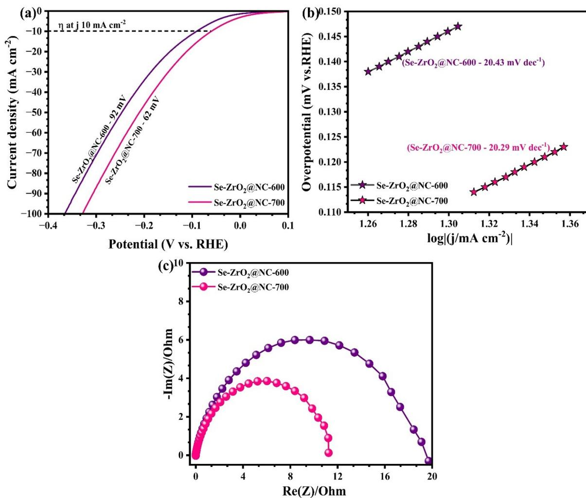
**Fig. S3** HER activity of Se-ZrO<sub>2</sub>@NC-600 and Se-ZrO<sub>2</sub>@NC-700 loaded electrode in 1.0 M KOH. (a) LSV polarization curves at 2 mV/s; (b) the corresponding Tafel plot and (c) Nyquist plots.
