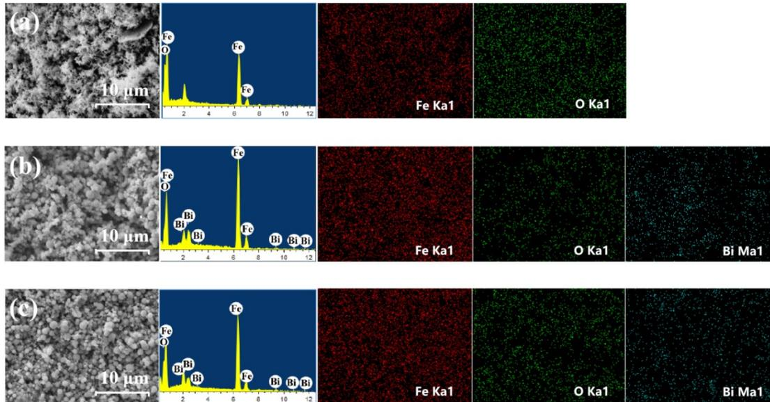
Fig. S9 SEM-EDS elemental mapping of (a) nZVI (b) Bi/nZVI and (c) 3<sup>rd</sup> Bi/nZVI
