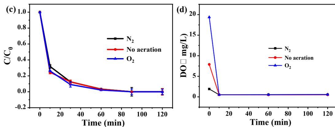
**Fig. S3** Degradation of (a) SM2 (b) SMX and (c) SD in the mixed liquid with different initial DO concentrations by Bi/nZVI-CA/NaCA system; (d) DO variation of the mixed liquid with different initial DO concentrations degraded by Bi/nZVI-
