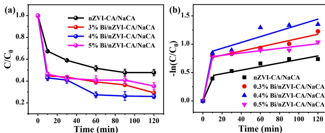
**Fig. S1** (a) Degradation efficiency of SM2 in Bi/nZVI-CA/NaCA system with different molar ratios of Bi/Fe; (b) Plots of  $\ln(C/C_0)$  versus time for the SAs
