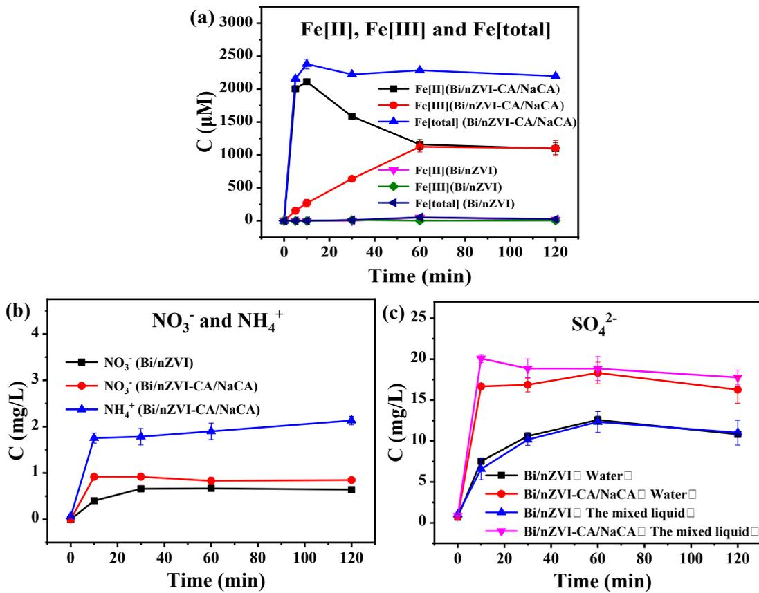
**Fig. S6** The concentration of (a) iron ion dissolution and (b) NO<sub>3</sub><sup>-</sup>/NH<sub>4</sub><sup>+</sup> in the mixed liquid by different systems; (c) The concentration of SO<sub>4</sub><sup>2-</sup> in the deionized water and mixed liquid by different systems
