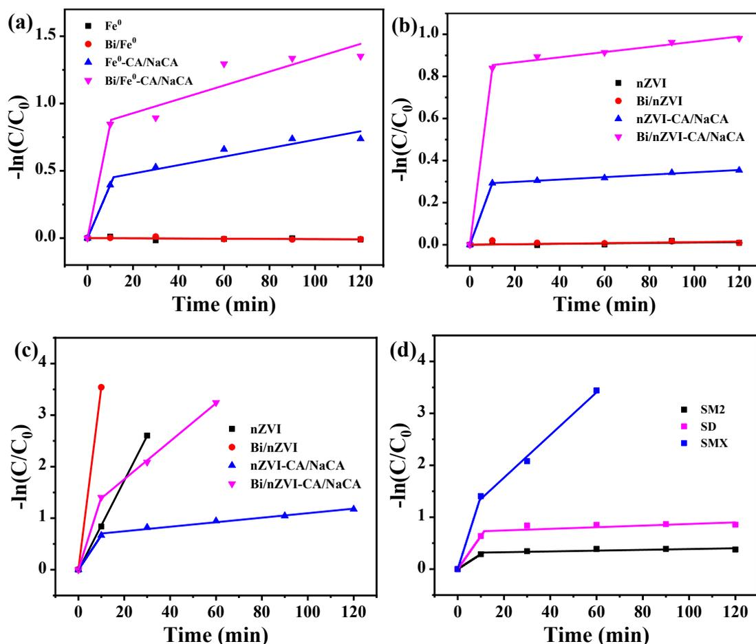
**Fig. S2** Plots of  $\ln(C/C_0)$  versus time for (a) SM2, (b) SD and (c) SMX degradation in different systems; (d) Plots of  $\ln(C/C_0)$  versus time for the SAs degradation in Bi/nZVI-CA/NaCA system
