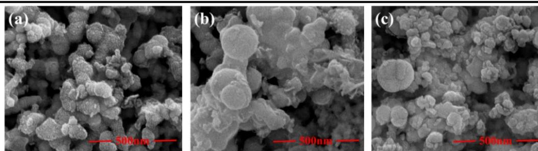
**Fig. S8** The SEM of (a) nZVI, (b) Bi/nZVI and (c) 3<sup>rd</sup> Bi/nZVI
