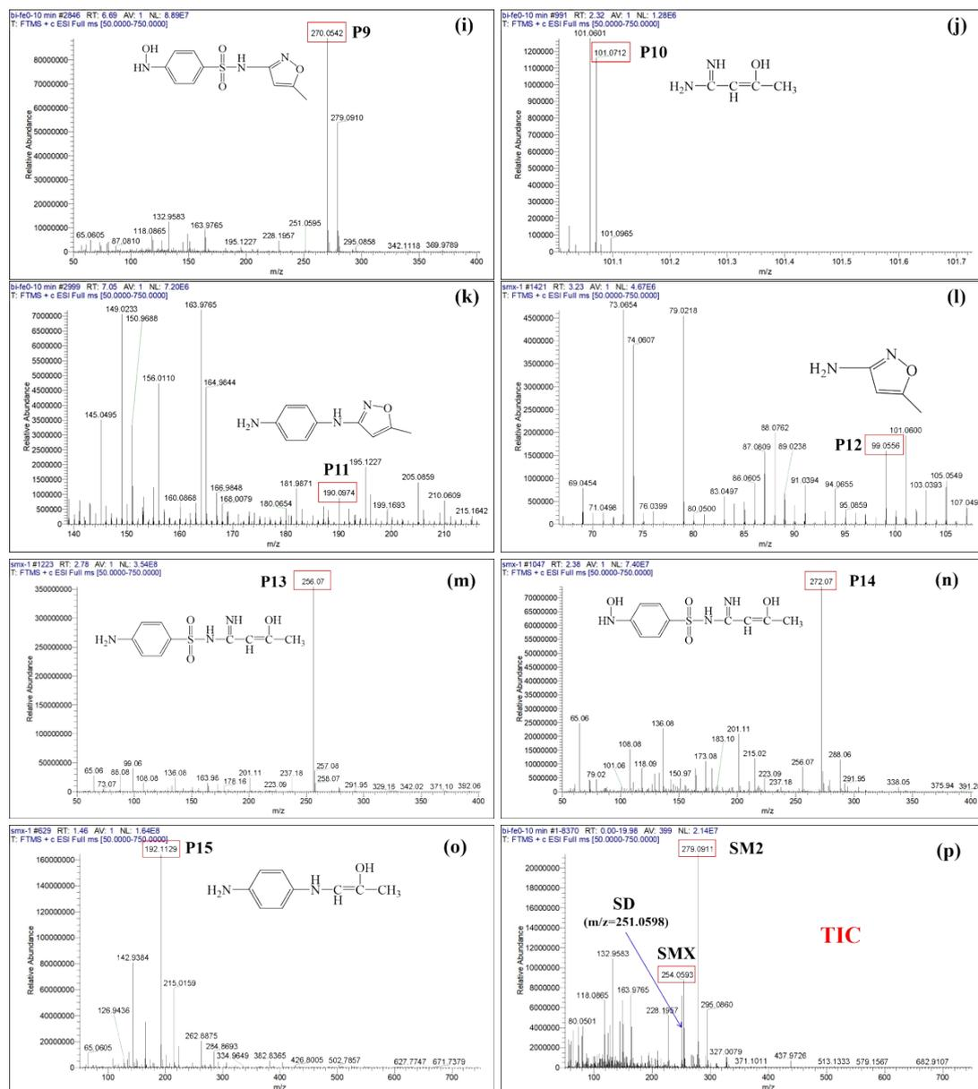
**Fig. S12** Mass spectrum of intermediate products produced by the degradation of SAs in Bi/nZVI-CA/NaCA system
