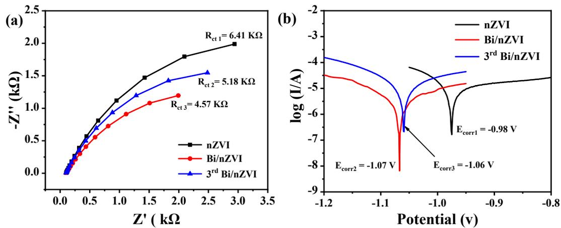
Fig. S11 (a) EIS and (b) Tafel curves of different samples
