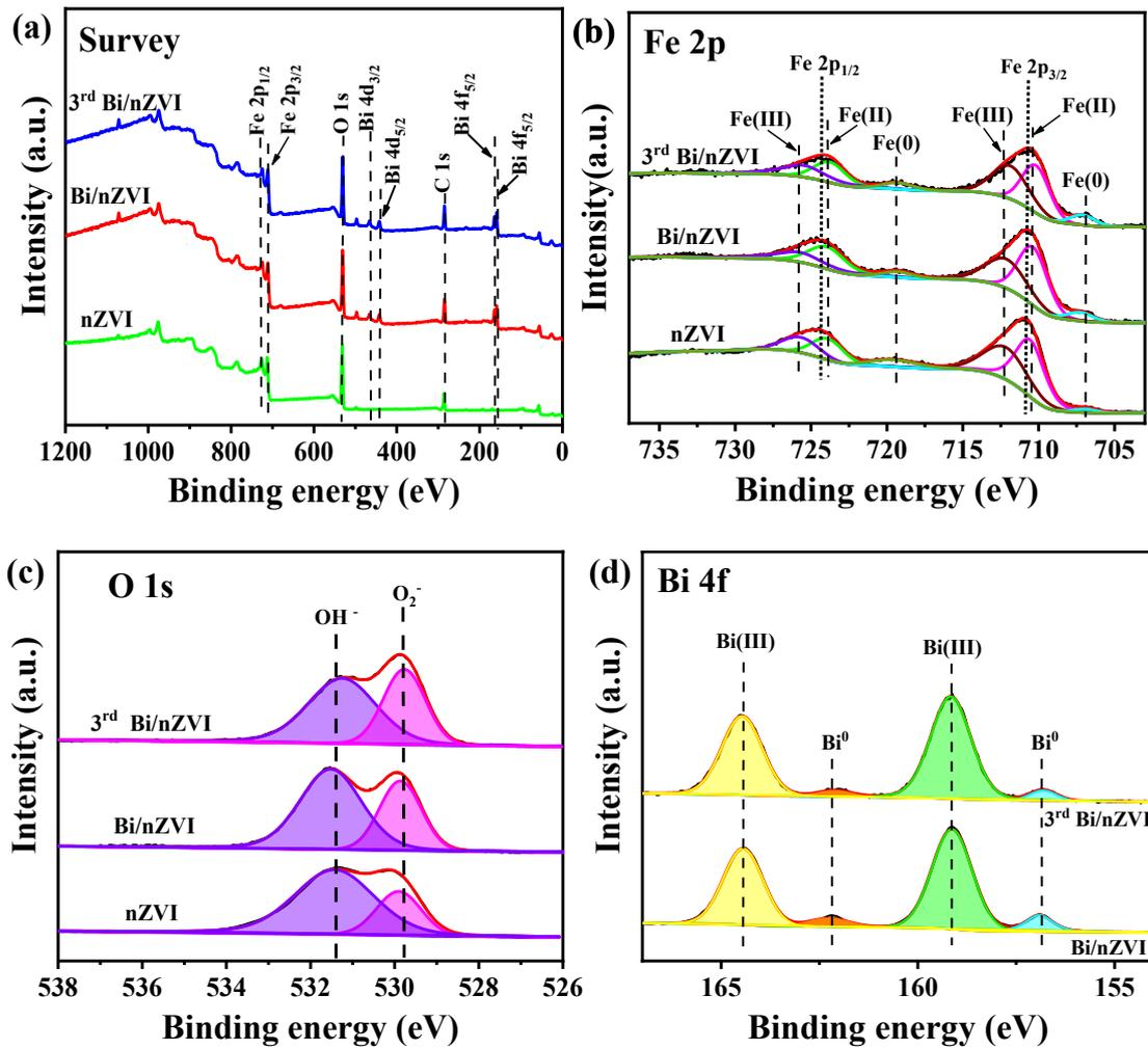
Fig. S10 XPS of (a) survey, (b) Fe 2p, (c) O 1s and (d) Bi 4f of different samples
