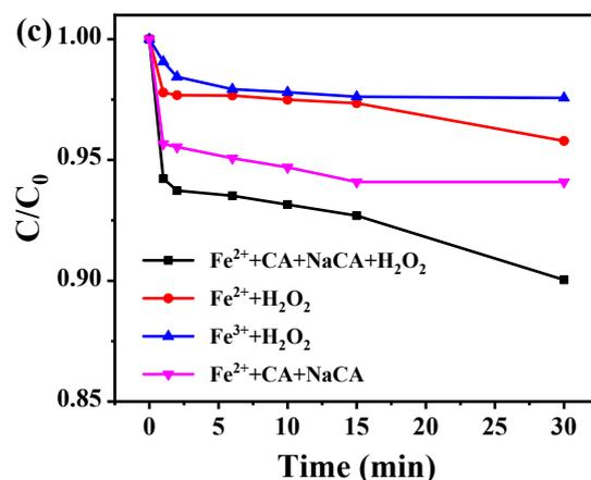
**Fig. S7** The degradation effects of different systems on (a) SM2, (b) SMX, and (c) SD in the mixed liquid (initial concentrations of Fe<sup>2+</sup> and Fe<sup>3+</sup> are both 2 mmol/L, initial concentrations of CA and NaCA are both 1 mmol/L, the initial concentration of H<sub>2</sub>O<sub>2</sub> is 400 μmol/L, and the quencher is tert butanol)
