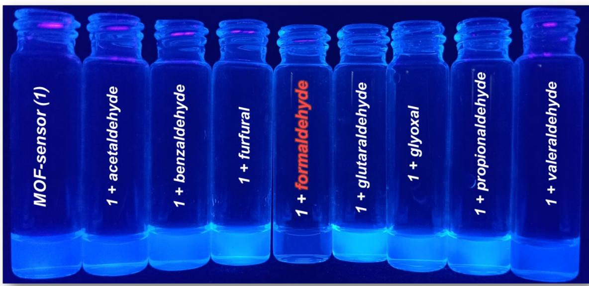
**Fig S25.** Physical image of the MOF-sensor (**1**) and sensor + analytes (aldehyde series) (1:1, v/v) under UV-irradiation.
