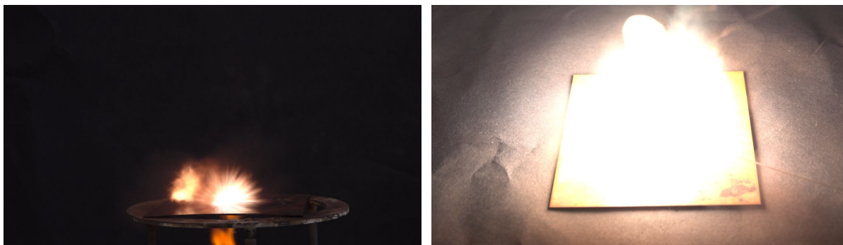
Figure S 13. Hot plate (left) and hot needle test of 1 .
