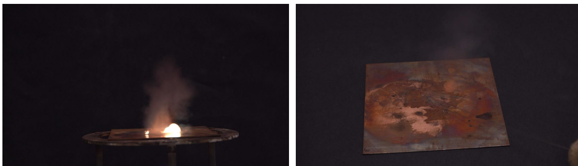
Figure S 17. Hot plate (left) and hot needle test of 5a .
