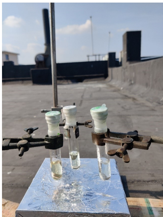
photo irradiation \lambda \geq 400 \text{ nm} , irradiation time 5 hours (a), without catalyst (b) with catalyst
