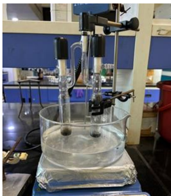
Figure. S16: Experimental bridge-shaped Schlenk tube setup for hydrogenation of styrene using Pd/C and generated H 2 from amine dehydrogenation.
