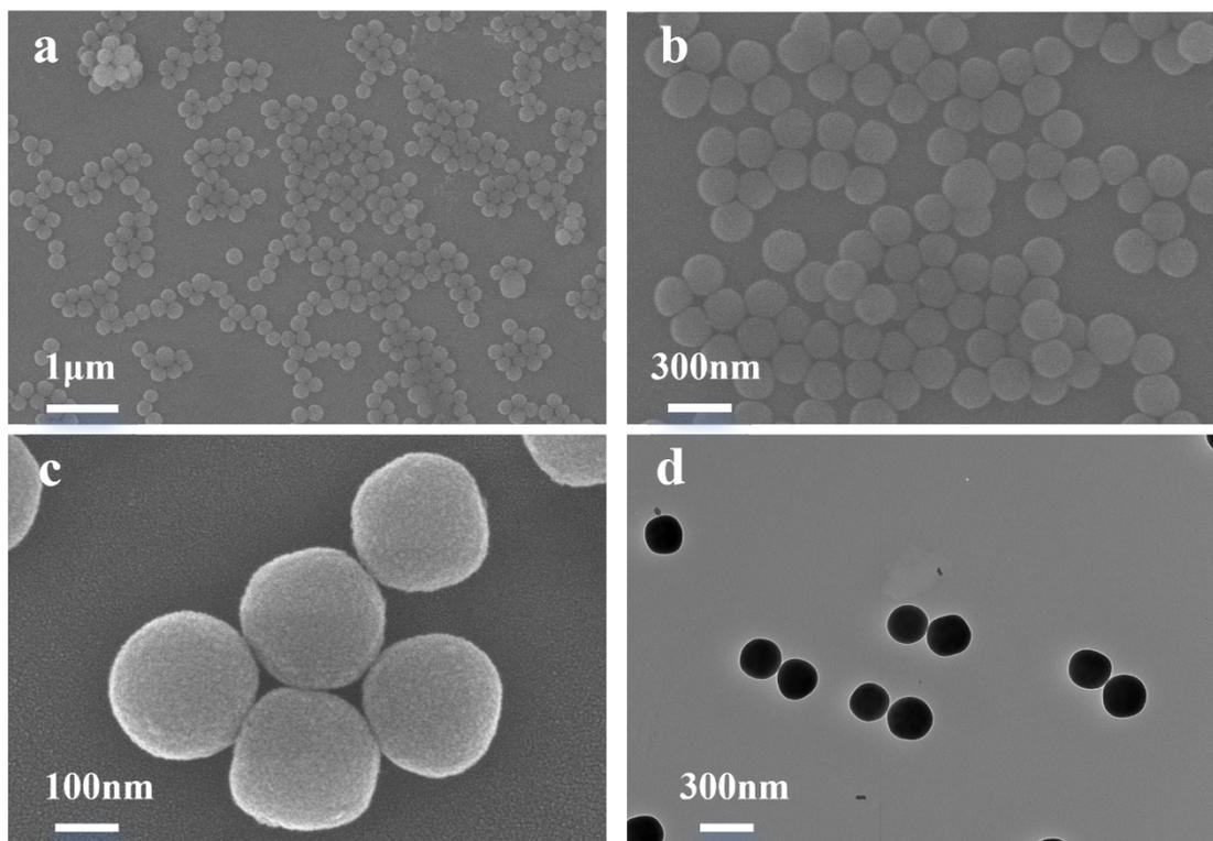
**Figure S1.** SEM and TEM images of the SiO<sub>2</sub> nanospheres prepared by the *Stöber* method. The SEM and TEM images reveal that the SiO<sub>2</sub> nanospheres (ca. 240 nm in diameter) exhibit a uniform and relatively smooth spherical morphology over a wide scope.
