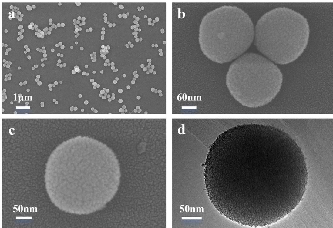
**Figure S2.** SEM and TEM images of the SiO<sub>2</sub>@CeO<sub>2</sub> composite abrasives.
