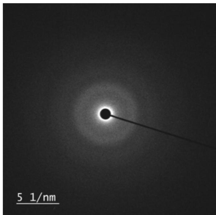
**Figure S5.** Selected area electronic diffraction (SAED) pattern, indicating the amorphous characteristics of such monodisperse  $\text{SiO}_2@\text{CeO}_2@\text{PDA}$  composite abrasives.
