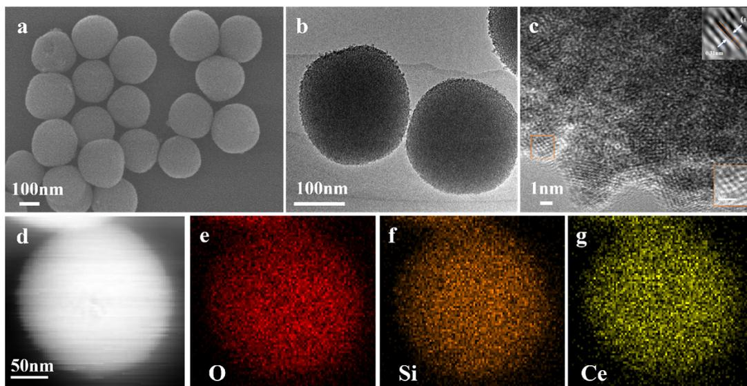
**Figure S3.** SEM (a), low- and high-resolution TEM (b, c) images of the SiO<sub>2</sub>@CeO<sub>2</sub> composite abrasives, which show the anisotropic growth of the lattice orientation along the (111) crystal plane in different regions. High-angle annular darkfield scanning TEM (HAADF-STEM) image (d) and energy dispersive X-ray spectroscopy (EDS) elemental mapping images of O (e), Si (f), Ce (g) of SiO<sub>2</sub>@CeO<sub>2</sub> composite abrasives.
