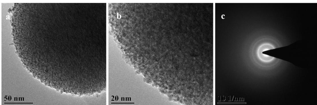
**Figure S4.** (a, b) HR-TEM images of the SiO<sub>2</sub>@CeO<sub>2</sub> composite abrasives at different magnifications. (c) Lattice and selected electron diffraction patterns of the SiO<sub>2</sub>@CeO<sub>2</sub> composite abrasives. No well-resolved diffraction rings can be observed in the high-resolution transmission electron microscopy (HRTEM) image and SAED pattern indicating the amorphous characteristics of such monodisperse SiO<sub>2</sub>@CeO<sub>2</sub> composite abrasives.
