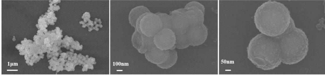
**Figure S7.** SEM(a), (b), (c) images of the SiO<sub>2</sub>@CeO<sub>2</sub>@PDA (16h) composite abrasives at different magnifications. While the reaction time was increased to 16 h, the further disordered growth of PDA resulted in serious abrasive agglomeration.
