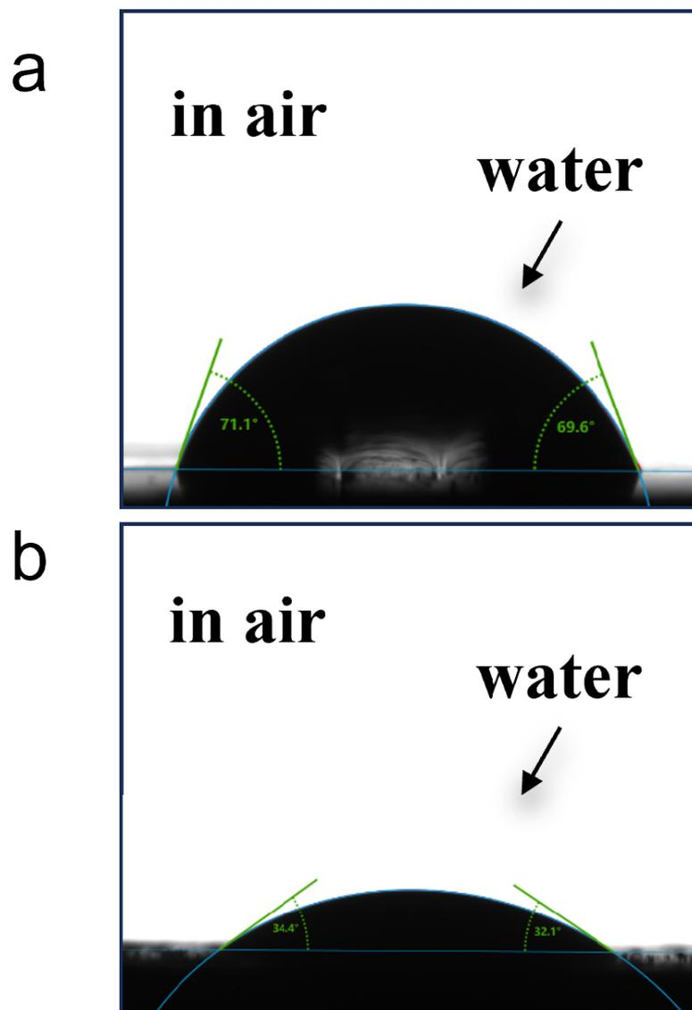
**Figure S6.** The contact angle (CA) of SiO<sub>2</sub>@CeO<sub>2</sub> (a) and SiO<sub>2</sub>@CeO<sub>2</sub>@PDA (b) composite abrasives on the SiO<sub>2</sub> wafer. The results showed that the hydrophilicity of the dopamine-modified abrasives was significantly enhanced.
