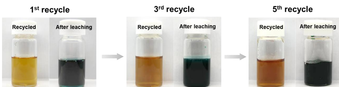
Figure S16. Recycling of the imidazolium glycol, the imidazolium glycol can be recovered and reused to dissolve the LCO five times with a similar color change due to its cyclability.
