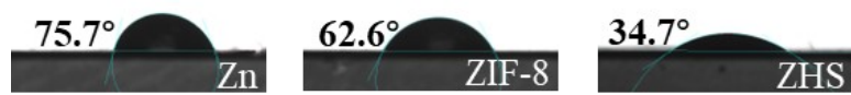
Figure S10. Contact angles of deionized water on the surfaces of bare Zn, Zn@ZIF-8 and Zn@ZHS-3h.
