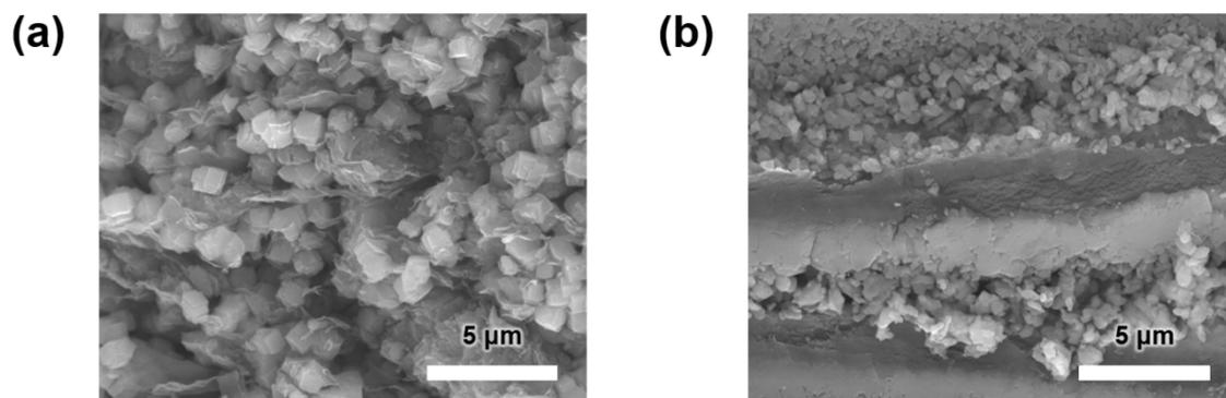
**Fig. S1.** SEM images of (a) BG particles in the BGC layer and (b) NaCl particles in the NC layer. NaCl and BG were incorporated in each layer in the form of crystalline particles, with sizes of  $\sim 1 \mu\text{m}$  (BG) and  $\sim 0.5 \mu\text{m}$  (NaCl).
