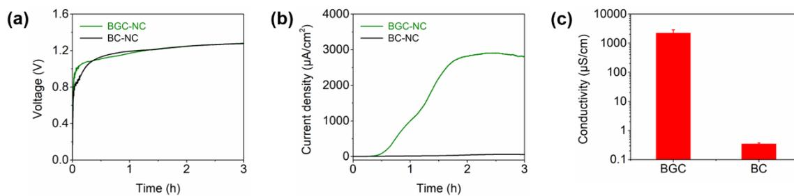
**Fig. S8.** Time-dependent changes in (a) voltage and (b) current density of BGC–NC (green) and BC–NC (black) at 90% RH for 3 h. (c) Electrical conductivity of BGC and BC. BC–NC reaches similar voltage (1.28 V), but has lower current and electrical conductivity ( $59.3 \mu\text{A}/\text{cm}^2$ ,  $0.347 \mu\text{S}/\text{cm}$ ) compared to BGC–NC ( $2,910 \mu\text{A}/\text{cm}^2$ ,  $2,230 \mu\text{S}/\text{cm}$ ), highlighting that GO acts as a conductive material within BGC.
