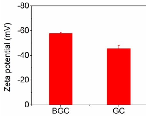
**Fig. S3.** Zeta potential of BGC and GC in DI water. Since BGC contains carboxyl and cyano functional groups, its surface becomes negatively charged at -57.8 mV.
