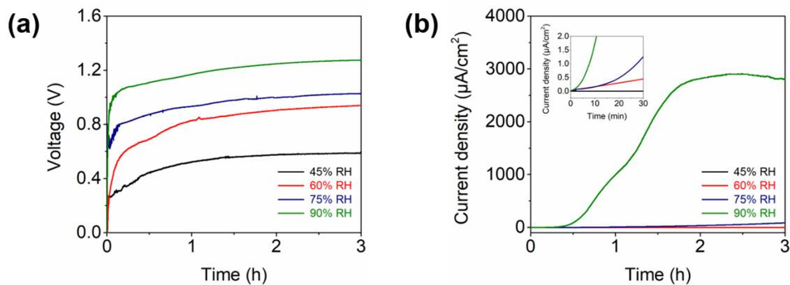
**Fig. S5.** Time-dependent changes in (a) voltage and (b) current density of BGC-NC at various RH values for 3 h. Inset provides a magnified view for below 75% RH. The voltage output increased with increasing RH, reaching its peak at 90% RH (1.28 V). Similarly, the current output increased with increasing RH, reaching 2,910  $\mu\text{A}/\text{cm}^2$  at 90% RH.
