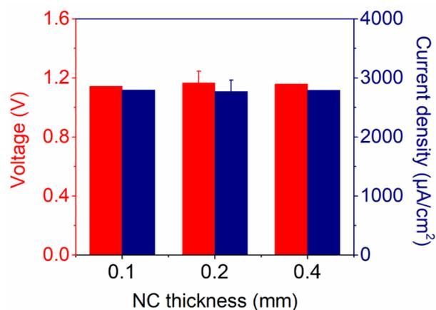
**Fig. S7.** Variations of the voltage (red) and current density (blue) output as a function of NC layer thickness of BGC–NC. While keeping the thickness of the BGC layer fixed at 1.1 mm, the thickness of the NC layer was varied to 0.1, 0.2, and 0.4 mm. The changes in the voltage and current outputs were negligible, indicating that the NC layer contains excess sodium ions that can reduce BG to PB.
