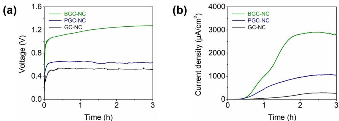
**Fig. S4.** Time-dependent changes in (a) voltage and (b) current density of GC-NC (black), PGC-NC (blue), and BGC-NC (green) at 90% RH for 3 h. The voltage (0.65 V) and current outputs ( $1,070 \mu\text{A}/\text{cm}^2$ ) of PGC-NC were higher than those of GC-NC due to the increased surface area for the physical adsorption of  $\text{Na}^+$  ions, but lower than those of BGC-NC.
