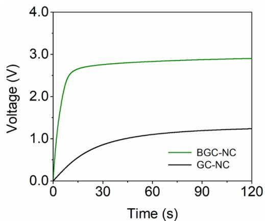
**Fig. S9.** Time-dependent changes in voltage when a 2000  $\mu\text{F}$  capacitor is charged by three GC-NCs (black) or three BGC-NCs (green) at 90 % RH. When a 2000  $\mu\text{F}$  capacitor was connected to three BGC-NCs, the BGC-NCs exhibited a much faster charging rate and reached a higher voltage than the GC-NCs.
