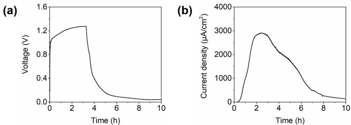
**Fig. S2.** Time-dependent changes in (a) open-circuit voltage and (b) short-circuit current density of BGC-NC at 90% RH for 10 h. Although the current density decreased from its peak value of 2,910  $\mu\text{A}/\text{cm}^2$ , it sustained a level of 140  $\mu\text{A}/\text{cm}^2$  even after 10 h.
