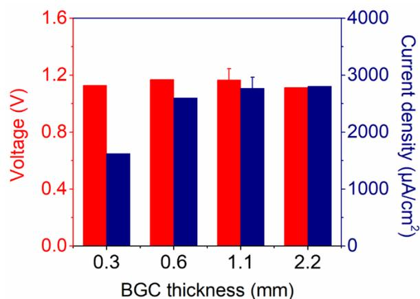
**Fig. S6.** Variations of the voltage (red) and current density (blue) output as a function of BGC layer thickness of BGC–NC. While keeping the thickness of the NC layer fixed at 0.2 mm, the thickness of the BGC layer was varied to 0.3, 0.6, 1.1, and 2.2 mm. The MEET performance increased as the BGC thickness increased, whereas it remained constant when the BGC layer thickness reached 2.2 mm.
