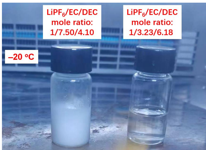
Fig. S13. The picture of dilute solution (left) and determined FCE (right) after keeping at -20\text{ }^{\circ}\text{C} for 24 h (firstly being frozen in liquid \text{N}_2 ). The dilute solution is the typical commercial formula, 1M \text{LiPF}_6 in EC-DEC (1:1, vol) (mole ratio of \text{LiPF}_6/\text{EC}/\text{DEC} is 1/7.50/4.10). The FCE component mole ratio \text{LiPF}_6/\text{EC}/\text{DEC} is determined as 1/3.23/6.18 (Table S14, ESI†).
