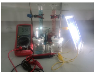
Figure S32. A photo showing a commercial silicon solar cell-driven electrolysis (1 cm 2 electrodes) of alkaline seawater.
