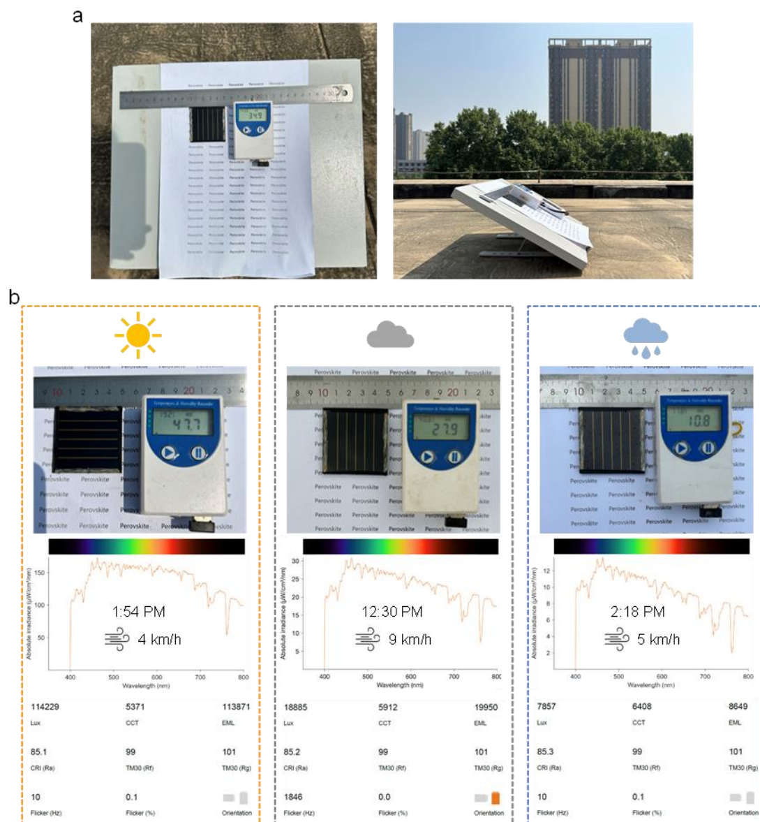
Fig. S49 Simple lighting platform for outdoor stability testing of encapsulated modules. (a) Photo of outdoor light test platform. The platform tilts at an angle of approximately 40^\circ and faces due south. The temperature and humidity are tracked in real time by the high precision temperature and humidity recorder (COS-04), which is powered by the silicon battery charging bank. (b) Photos of outdoor illumination of modules in different weather and corresponding sunlight spectrum.
